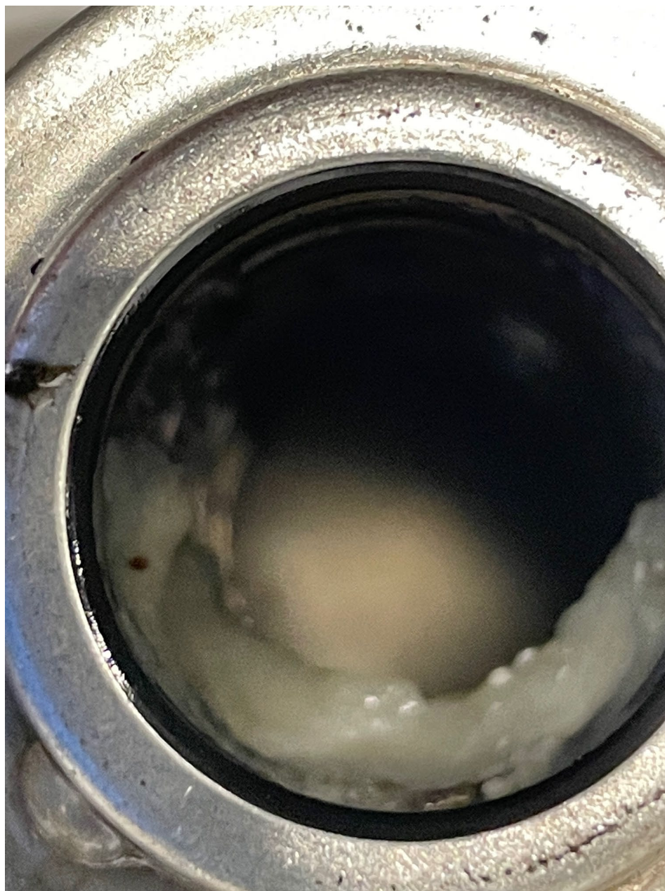
Photo 3 – Engine Mounted Fuel Filter Interior (Rolls-Royce)
