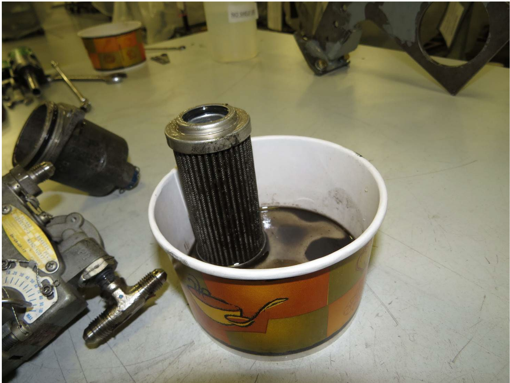
Photo 2 – Engine Mounted Fuel Filter (Rolls-Royce)
