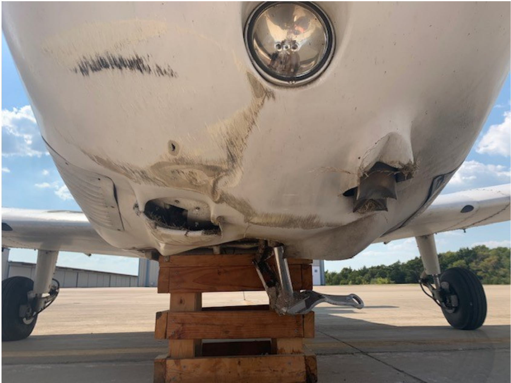
Photo 4 - Damage to the cowling after the nose gear separated. (FAA photo).
