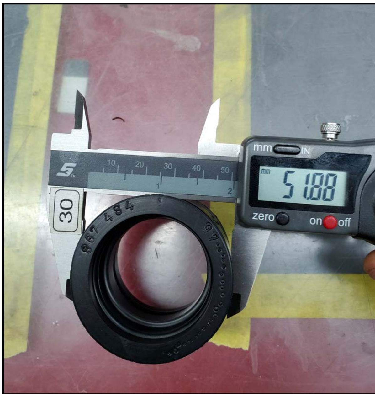
Photo 6 – Carburetor Socket (Rotech Flight Safety Photo)
