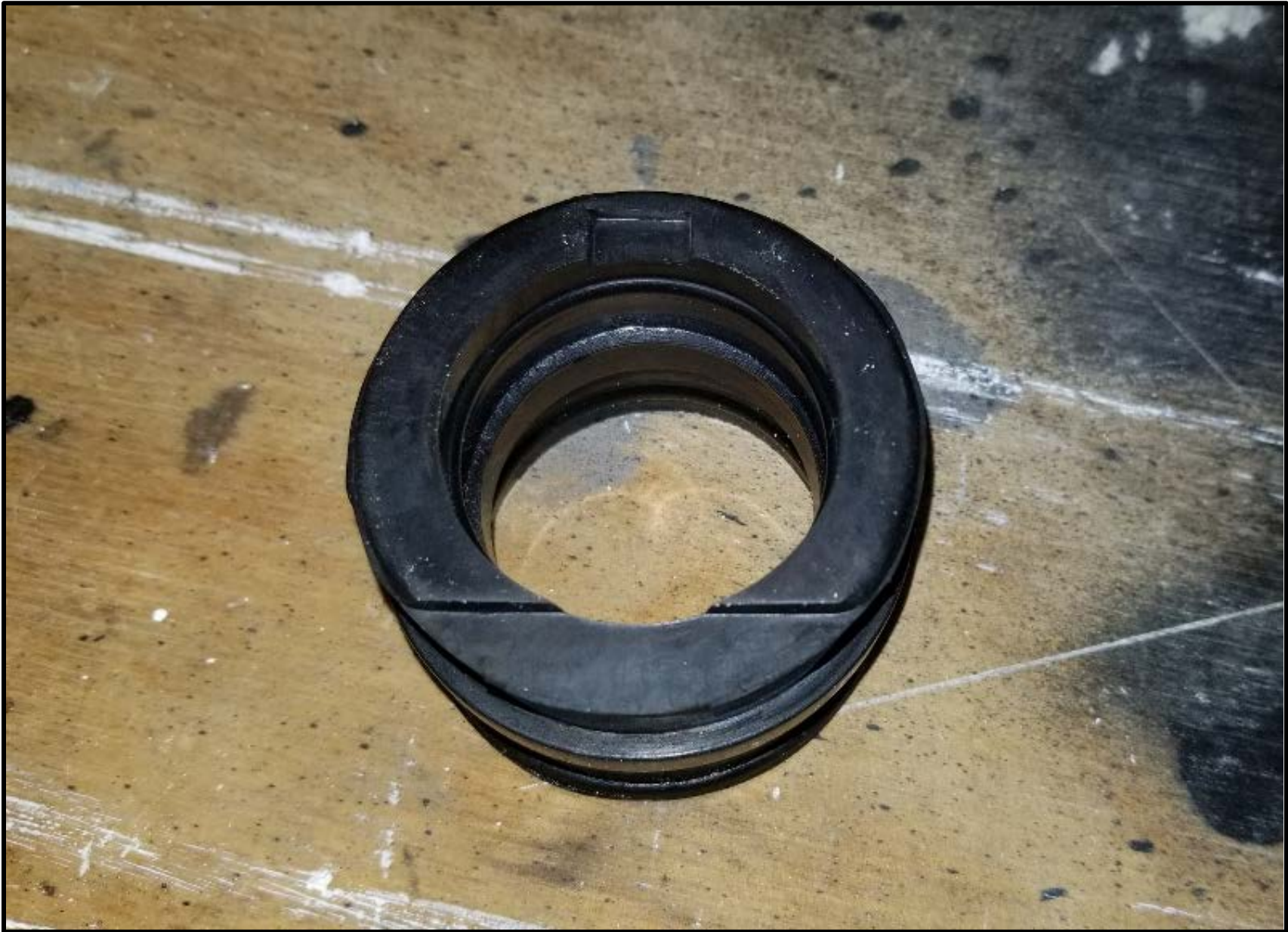
Photo 5 – Forward Carburetor Socket (Airplane Owner Photo)
