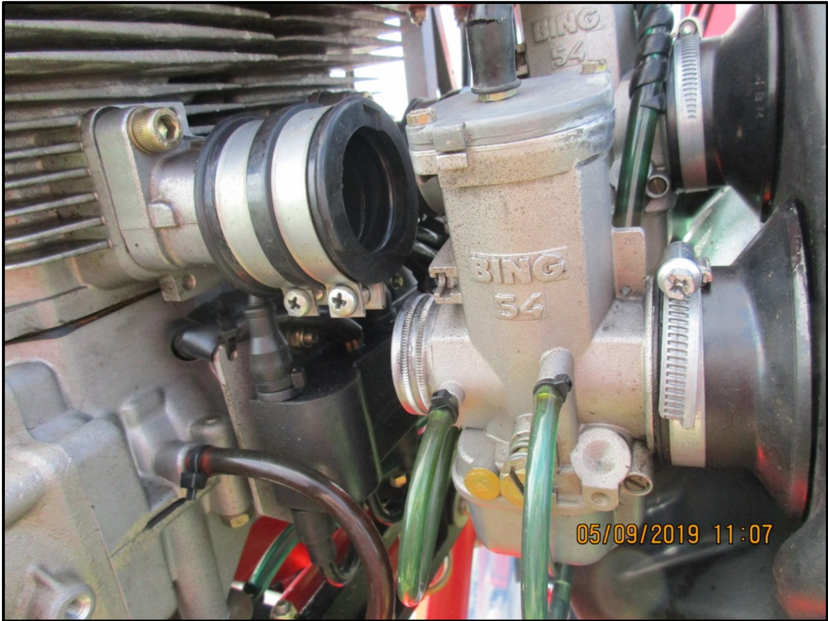
Photo 2 – Carburetor Installation (FAA Photo)
