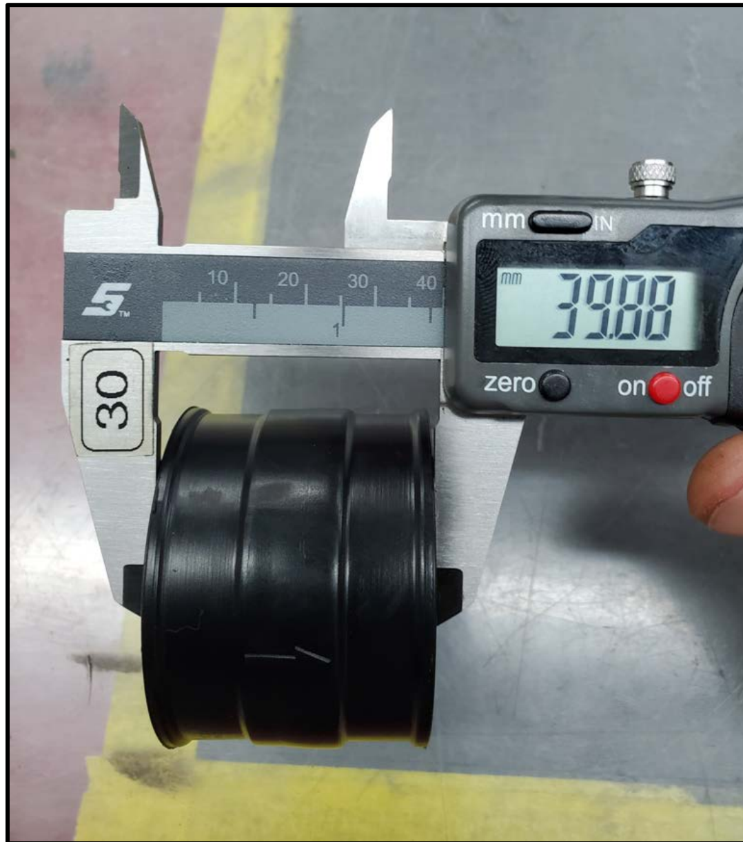
Photo 8 - Carburetor Socket (Rotech Flight Safety Photo)
