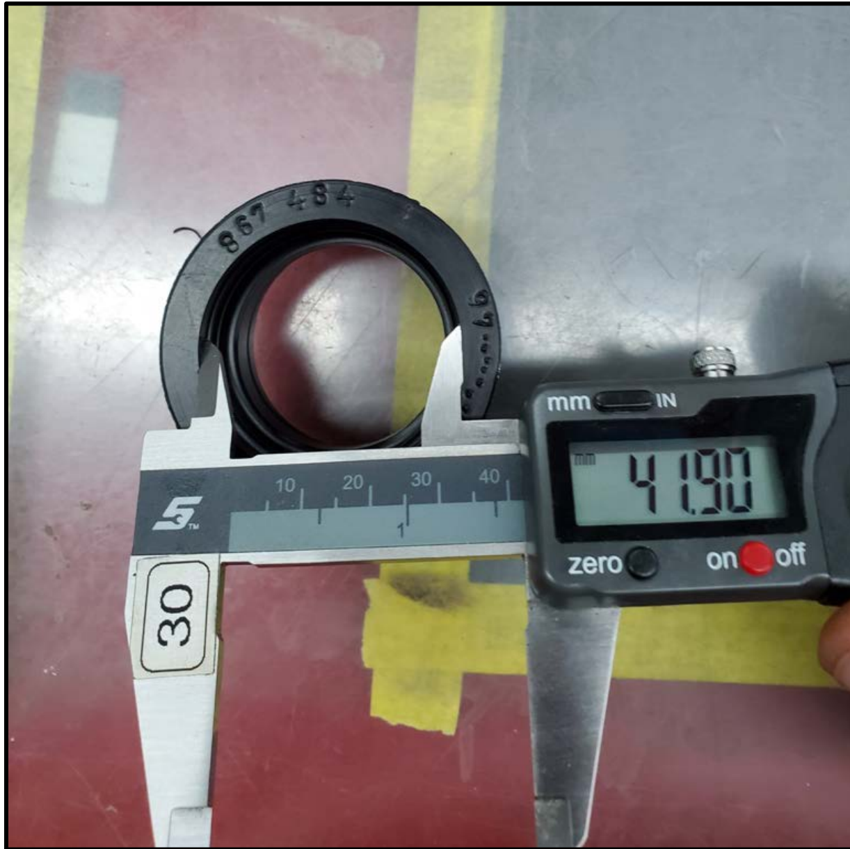
Photo 7 - Carburetor Socket (Rotech Flight Safety Photo)
