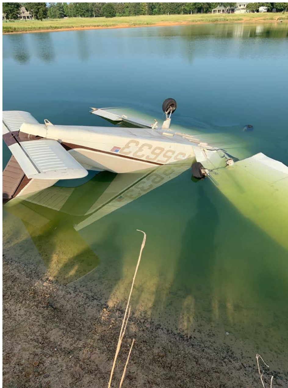
Photo 3 – View of the submerged inverted airplane in the pond, with a visible fuel sheen on the water (courtesy of the Federal Aviation Administration).
