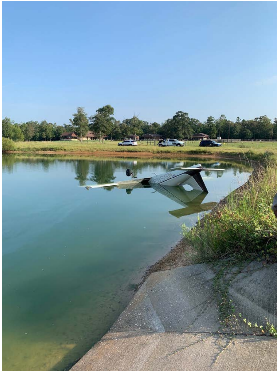
Photo 1 – View of the submerged inverted airplane in the pond, with a visible fuel sheen on the water (courtesy of the Federal Aviation Administration).
