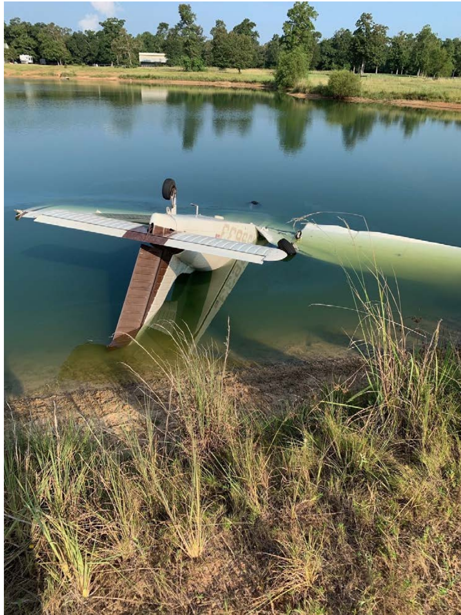
Photo 2 – View of the submerged inverted airplane in the pond, with a visible fuel sheen on the water (courtesy of the Federal Aviation Administration).
