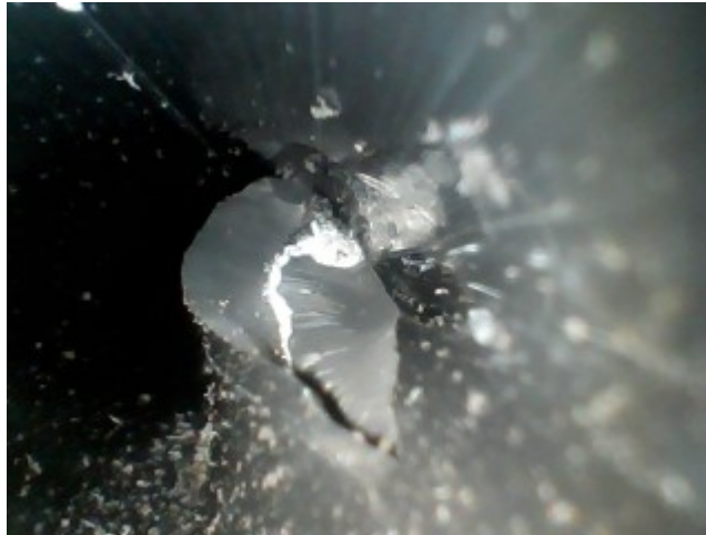
Tear in Boost Pump to Fuel Selector Valve Hose
