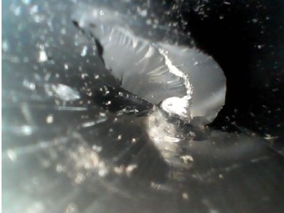
Photo 11 – Fuel Hose #2 – Internal Rubber Fracture (via Borescope)
