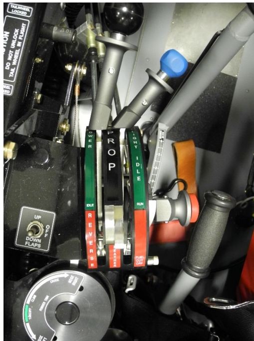
Photo 18 – Kawak Quadrant – Integrated Detent Handles Close to Control Knob
