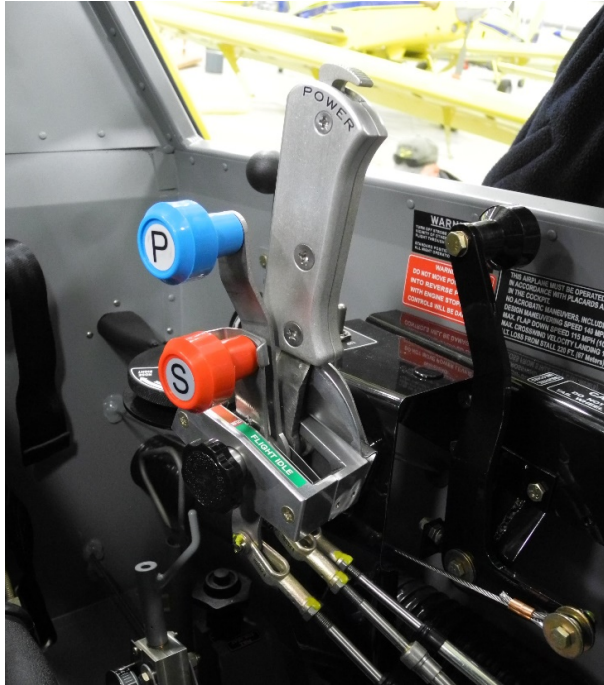
Photo 19 – Standard Air Tractor Quadrant – Note Separate Detent Handles
