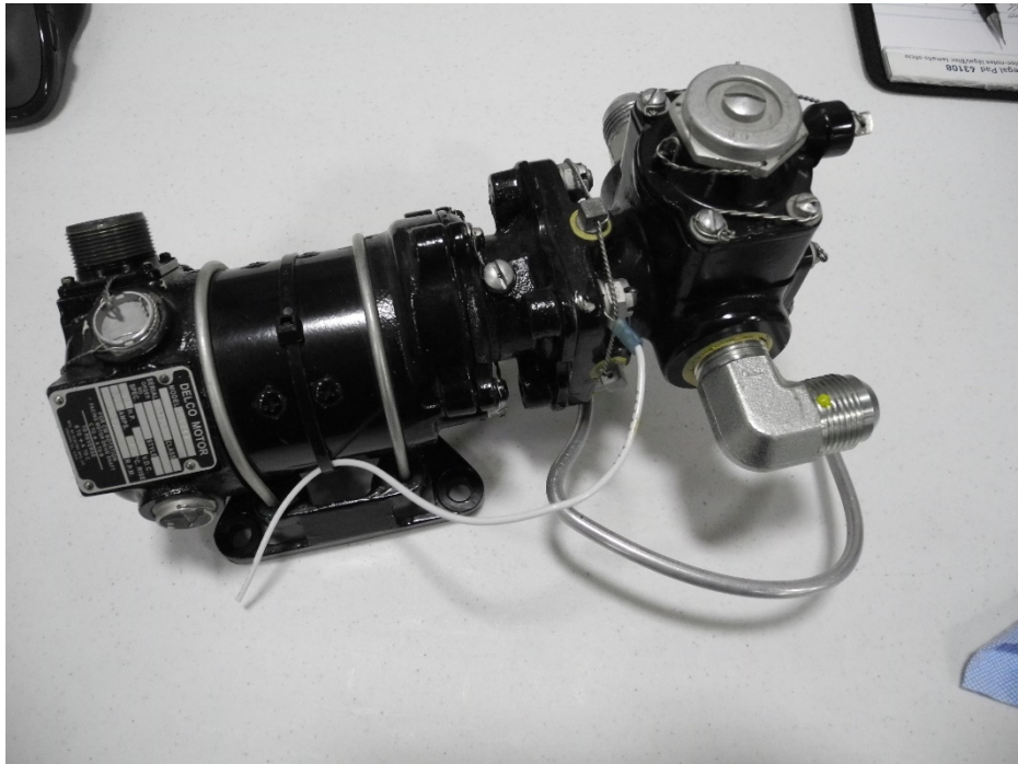
Photo 12 – Low-Pressure Airframe Electric Fuel Pump
