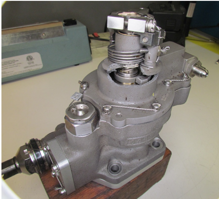
Photo 10 – Propeller Governor (CSU) - Fractured
