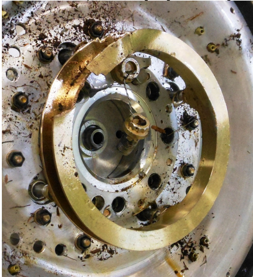
Photo #3 – Propeller mounting flange and beta ring
