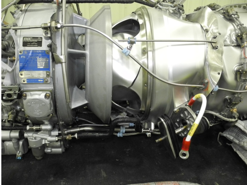
Photo 7 - Compressor Housing – Buckled and Torn
