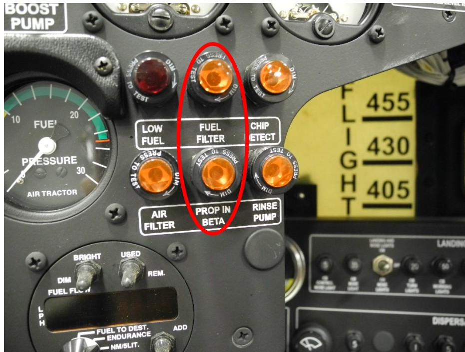
Photo 17 – Cockpit Gauges Depicting Proximity of Amber Warning Lights
