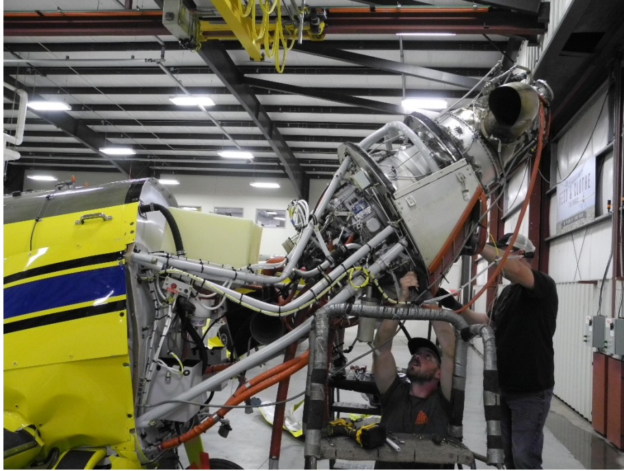
Photo 3 – Engine Still Attached to Airframe Mount
