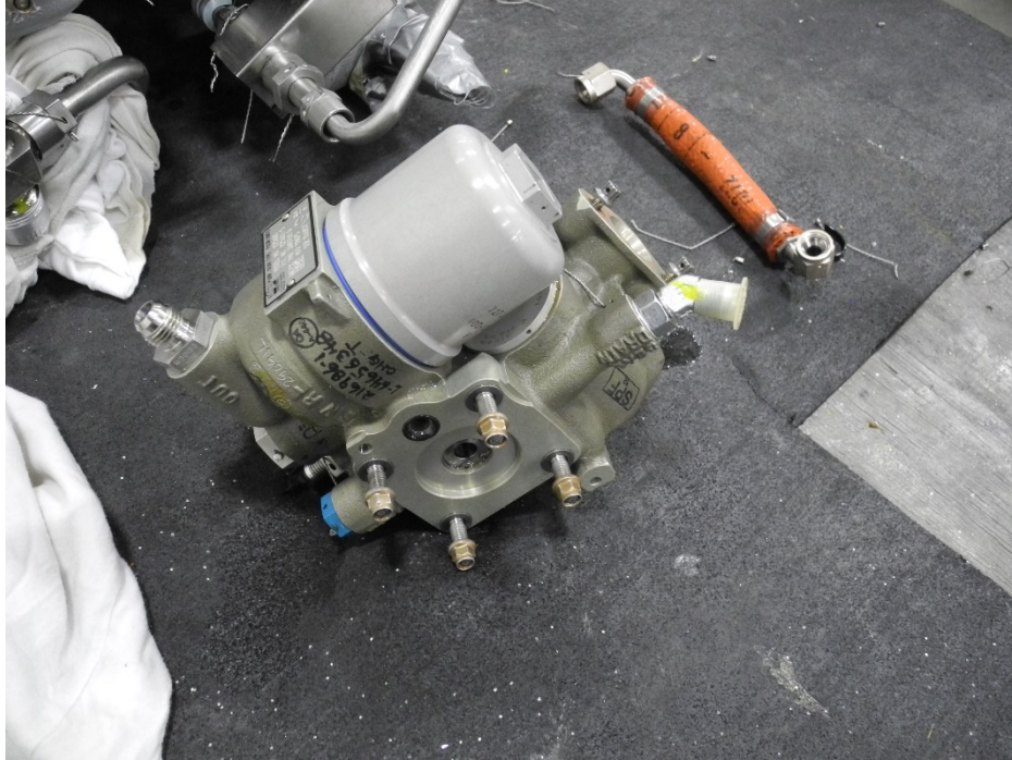
Photo 9 – Fuel Pump - Undamaged
