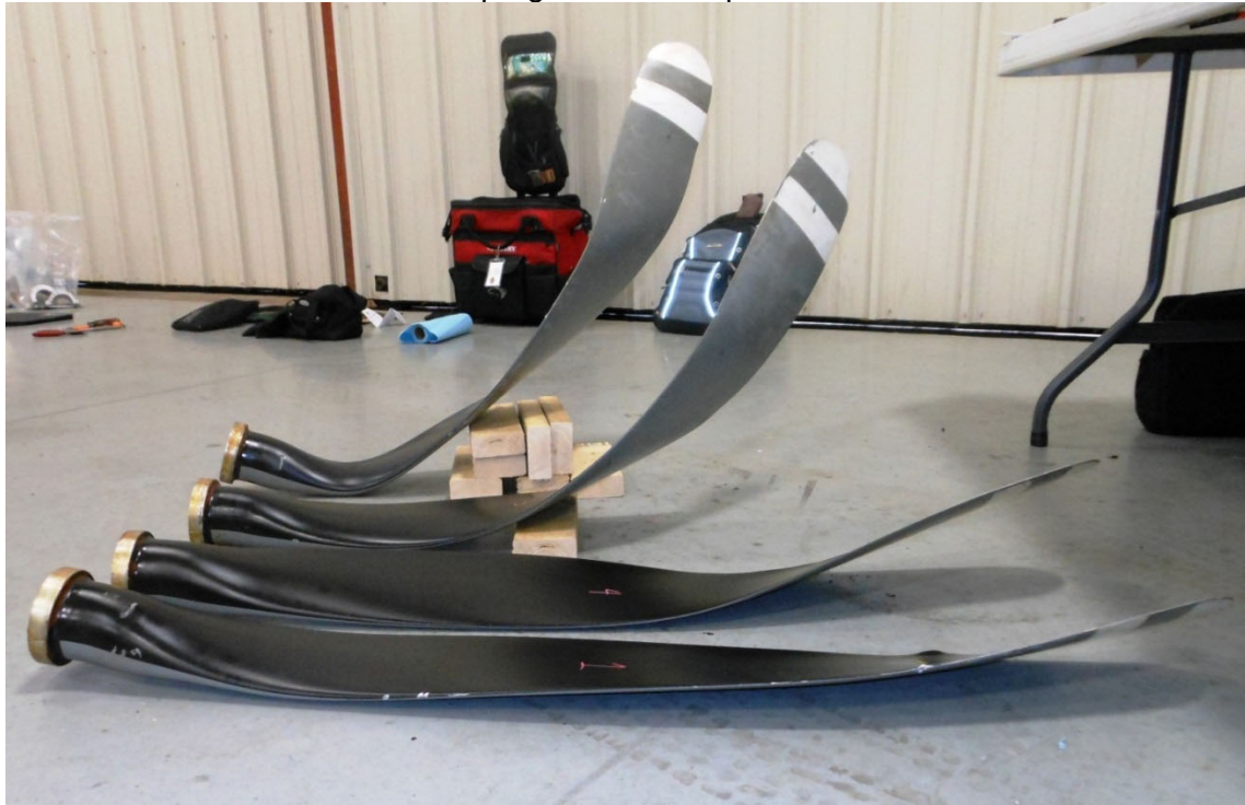
Photo #9 – Blade progressive, compound bend and twist
