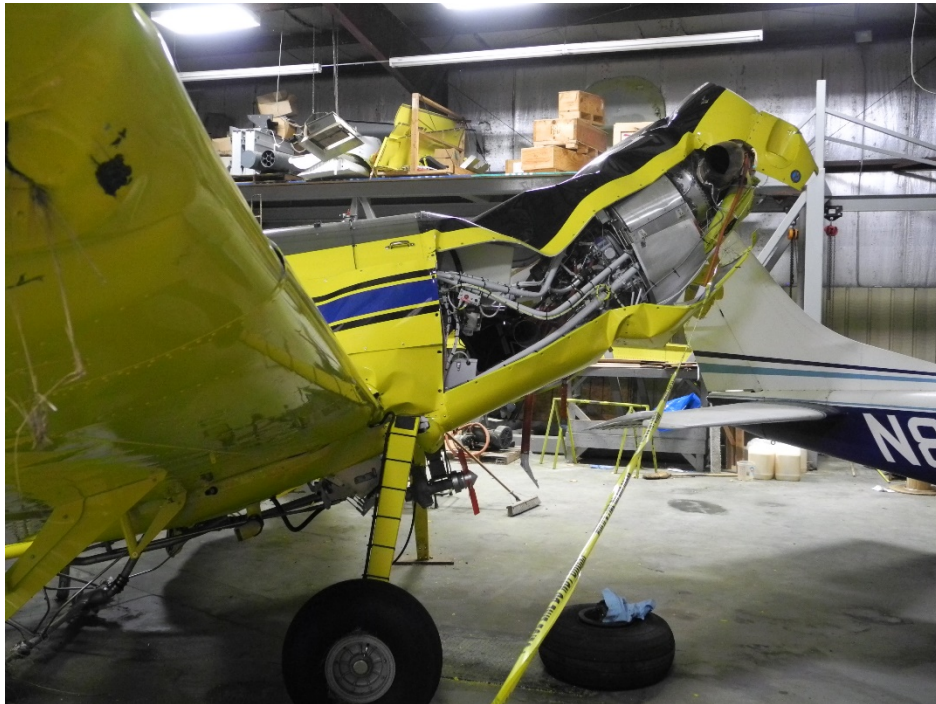
Photo 2 – AT-502 Engine Frame & Mount Damage
