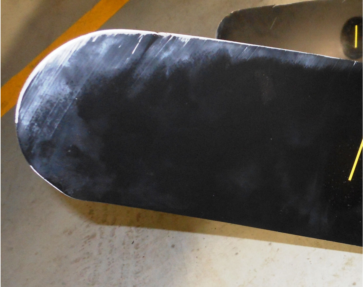
Photo #8 – Blade #3 face side – typical degree of chordwise/rotational abrasion
