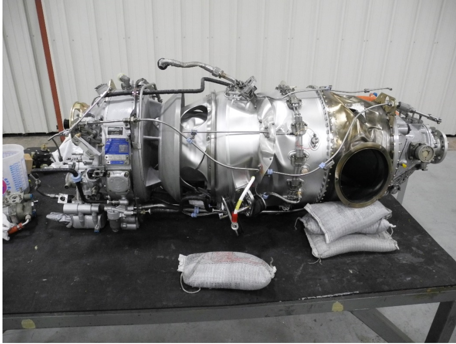
Photo 6 – RGB Fractured and Exhaust Housing Buckled
