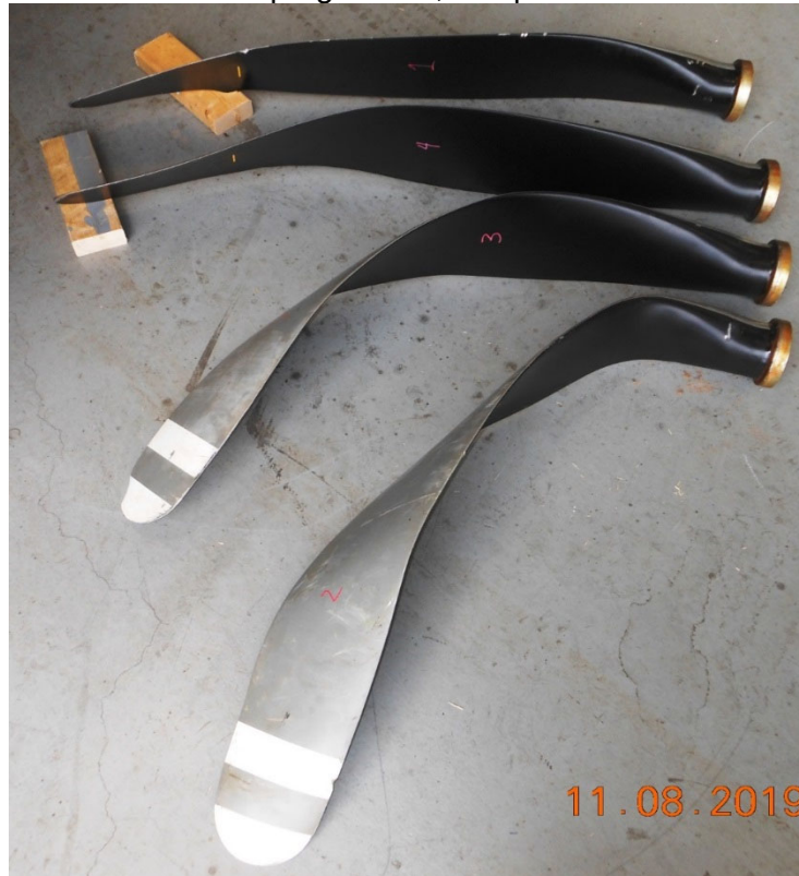
Photo #10 – Blade progressive, compound bend and twist
