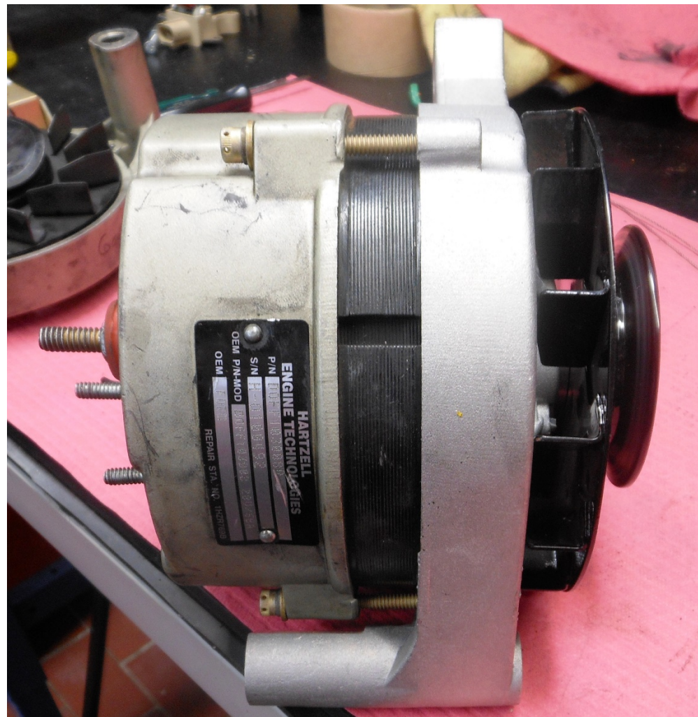
Photo 3 – Accident Alternator with Damaged Front Housing (Left) and Accident Alternator with Exemplar Front Housing Installed for Testing (Right) (Courtesy of Manufacturer)
