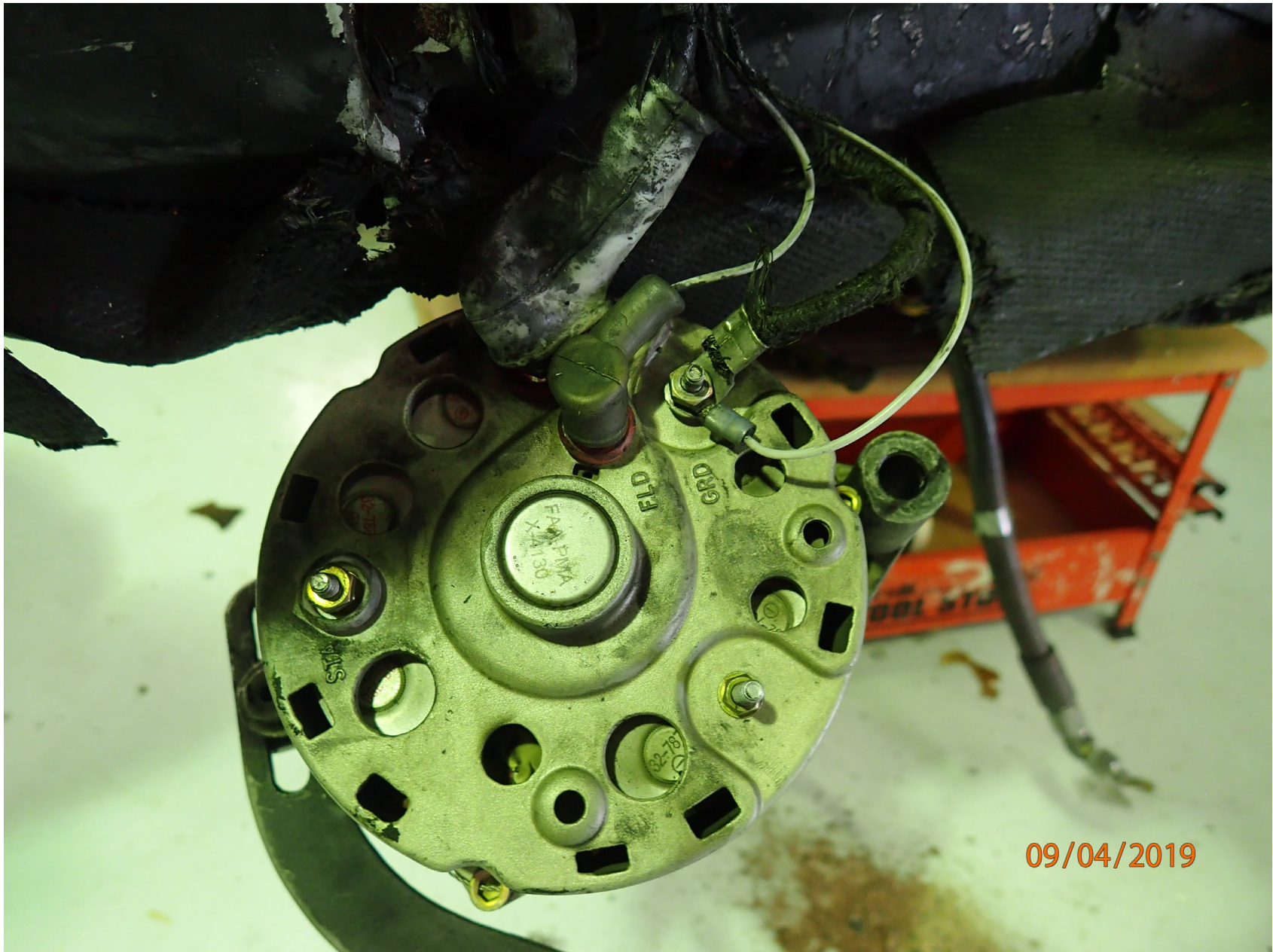
Photo 2 – Alternator as Installed in Accident Airplane
