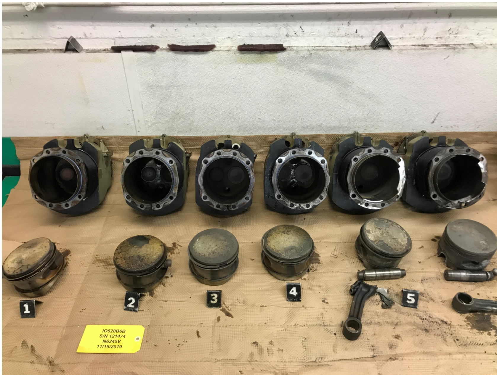
Photo 13 – All cylinders and piston heads
