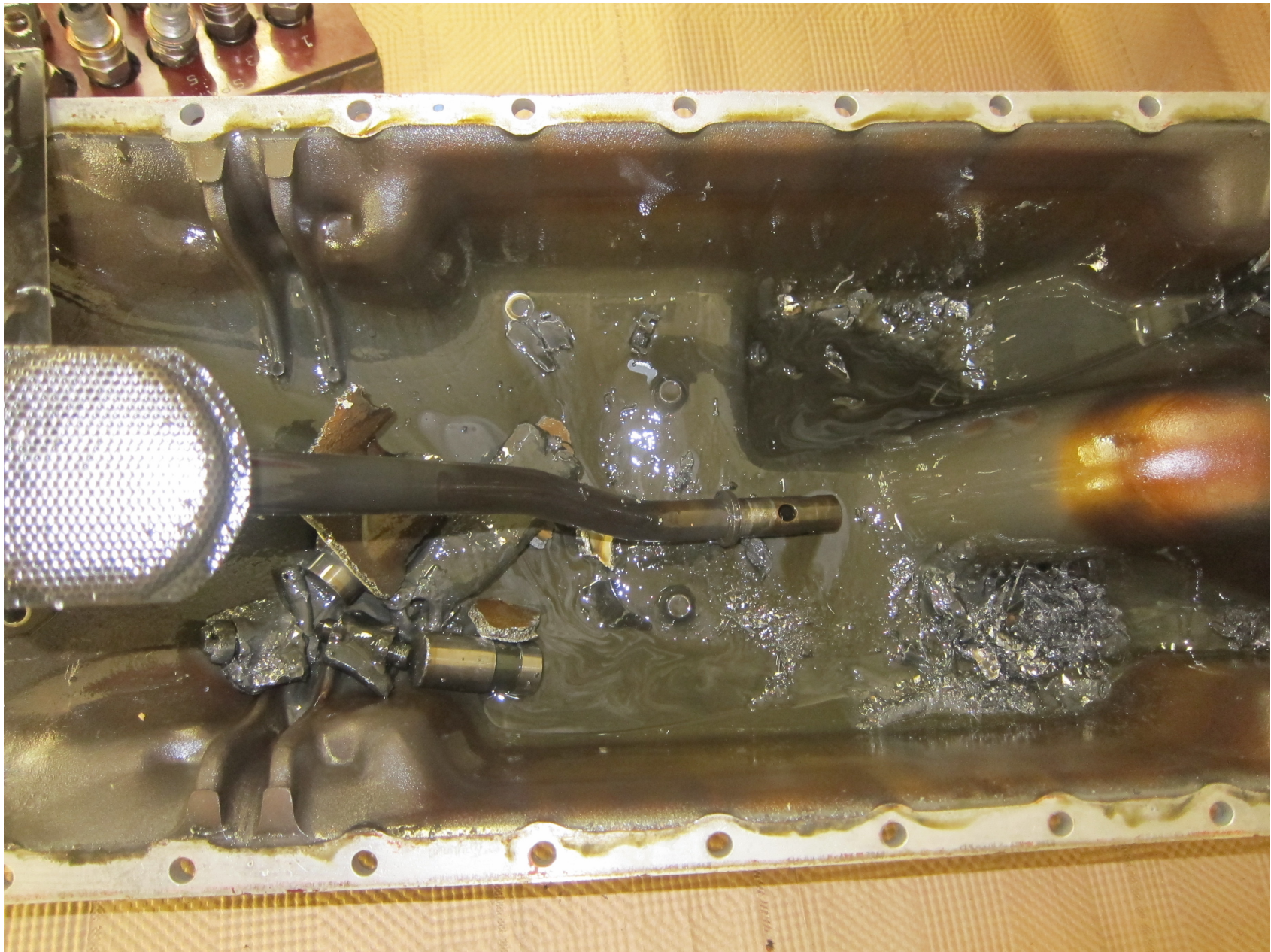
Photo 24 – Debris in oil pan
