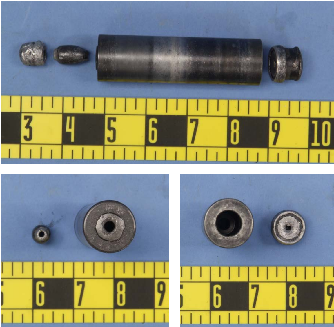
Figure 2: Overall photos of the fractured wrist pin.
