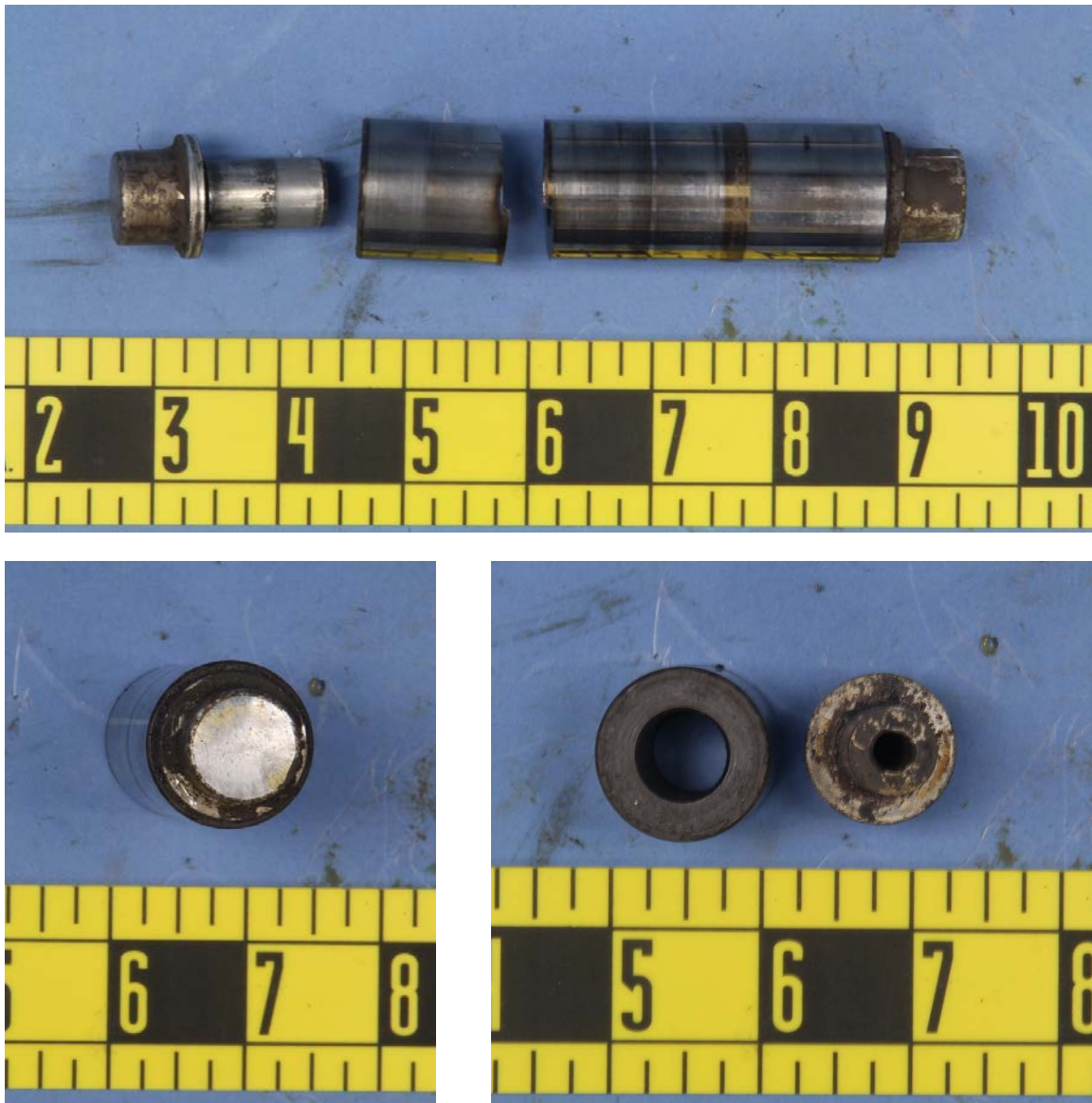
Figure 1: Overall photos of the exemplar sectioned wrist pin.
