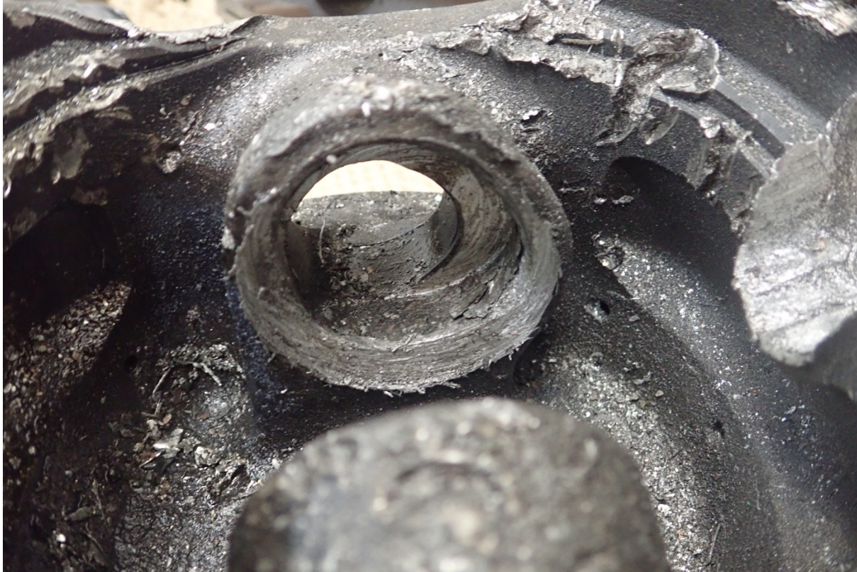
Cylinder 6 piston pin boss, ASI-19-CU-137
