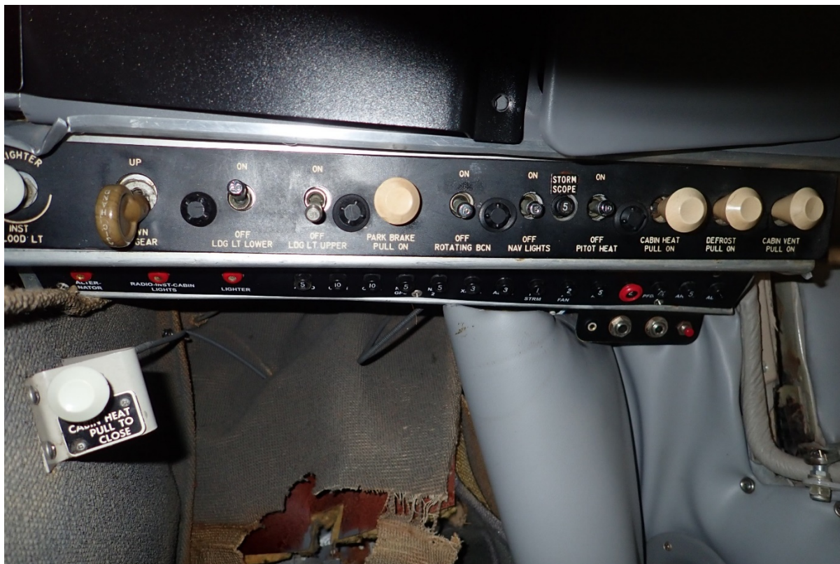
Switch panel, ASI-19-CU-043
