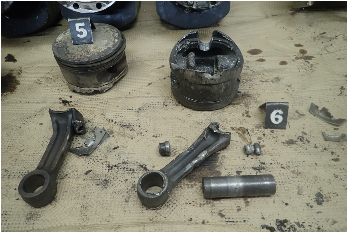
Cylinder 5 & 6 pistons and fractured connecting rods, ASI-19-CU-134
