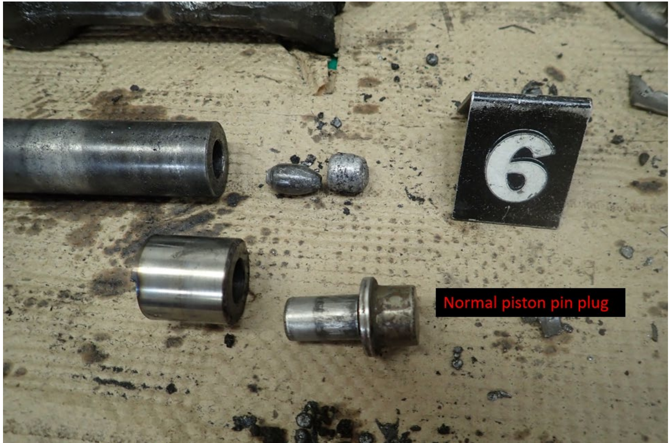
Comparison of piston pin plug from cylinder 6 to a normal plug, ASI-19-CU-136
