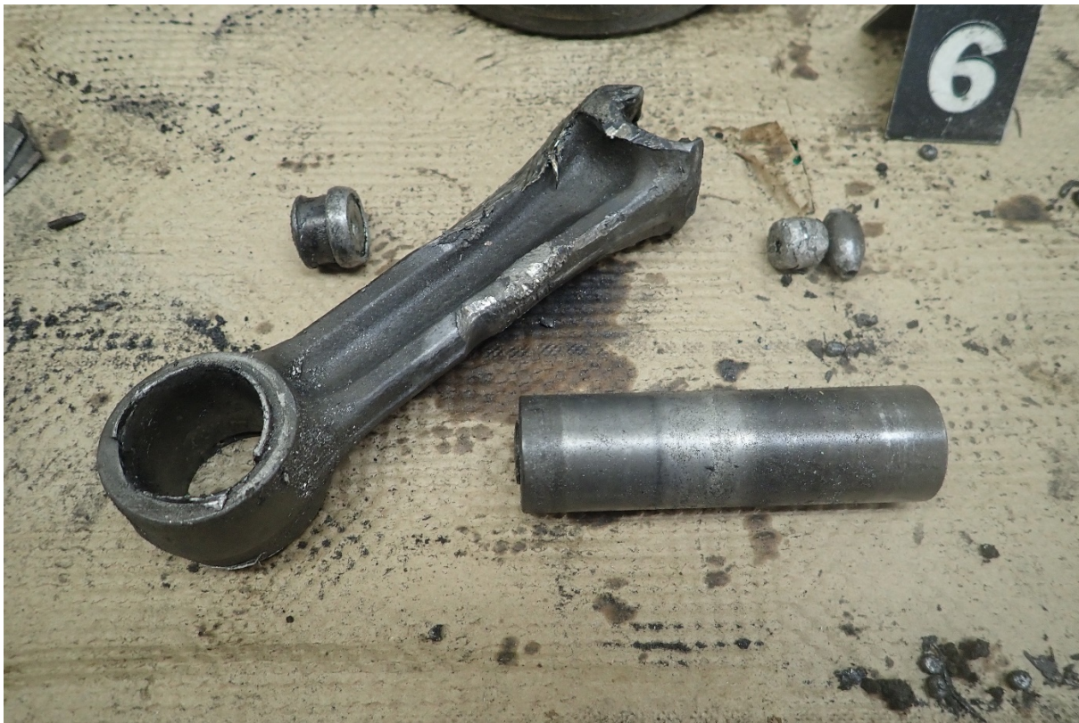
Cylinder 6 connecting rod, piston pin & plug, ASI-19-CU-135
