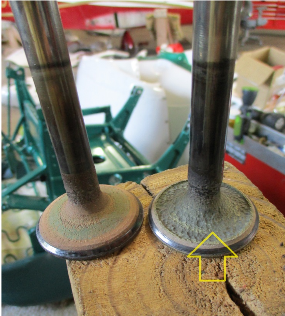
Photo 3 – Erosion on the number 4-cylinder exhaust valve
