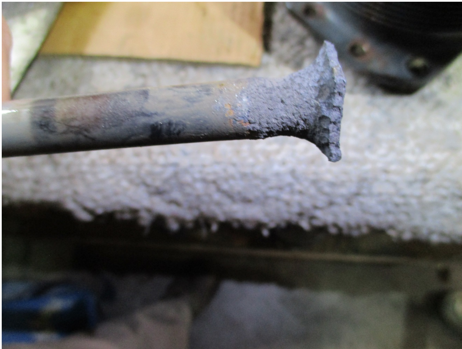
Photo 2 – Failed Exhaust valve
