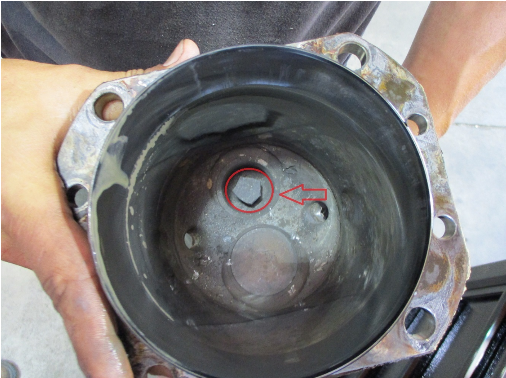
Photo 1 – Number 3 cylinder, with failed exhaust valve
