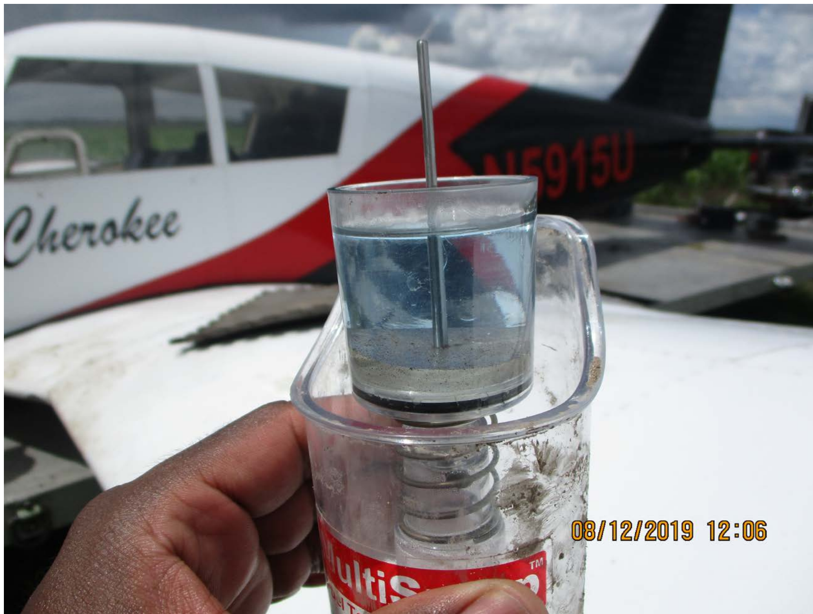
Photo 10 - FAA supplied view of an additional sample from the left wing's sump. The sample contains a cloudy colored liquid at the bottom of the sampler and a blue colored liquid above the cloudy layer.
