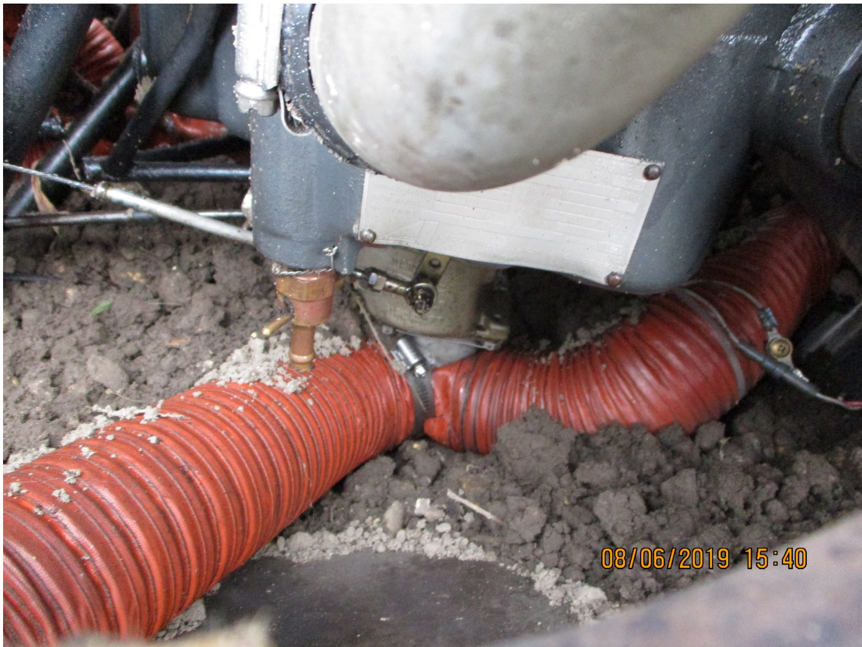
Photo 7 - FAA supplied view of the carburetor and its linkage.
