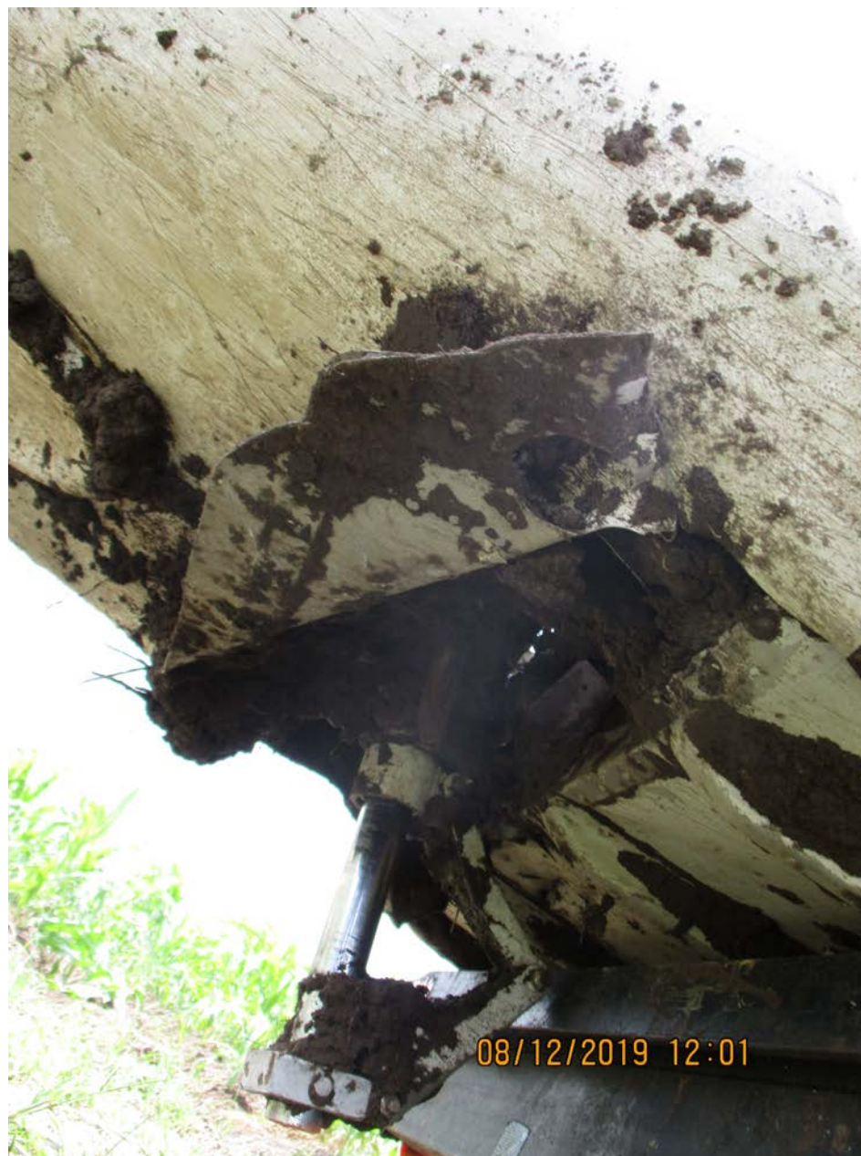
Photo 18 - FAA supplied view of the nose landing gear scissors. The landing gear below the scissors is not present.
