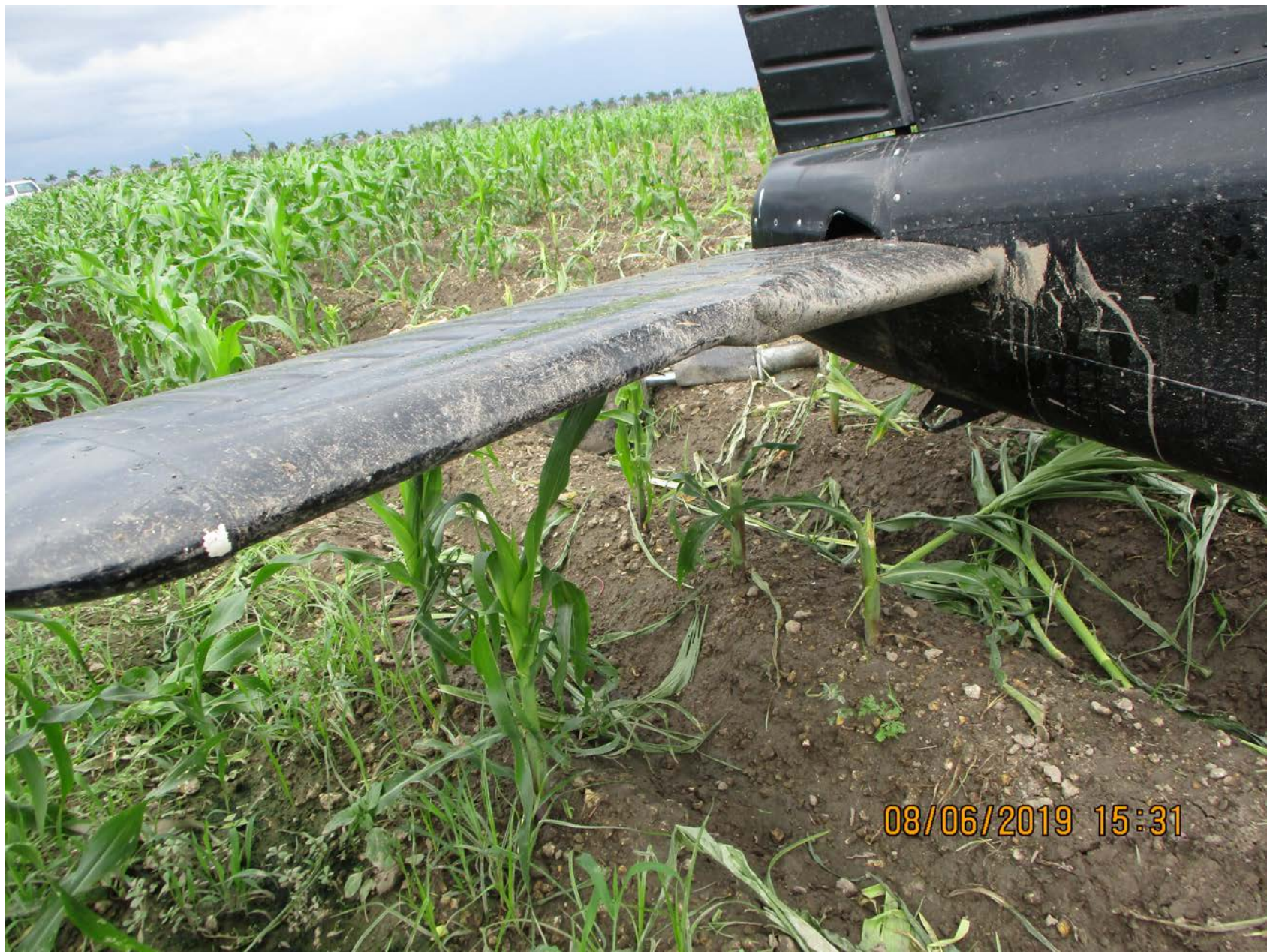
Photo 5 - FAA supplied view of the right horizontal stabilizer exhibiting leading edge damage. a landing gear.
