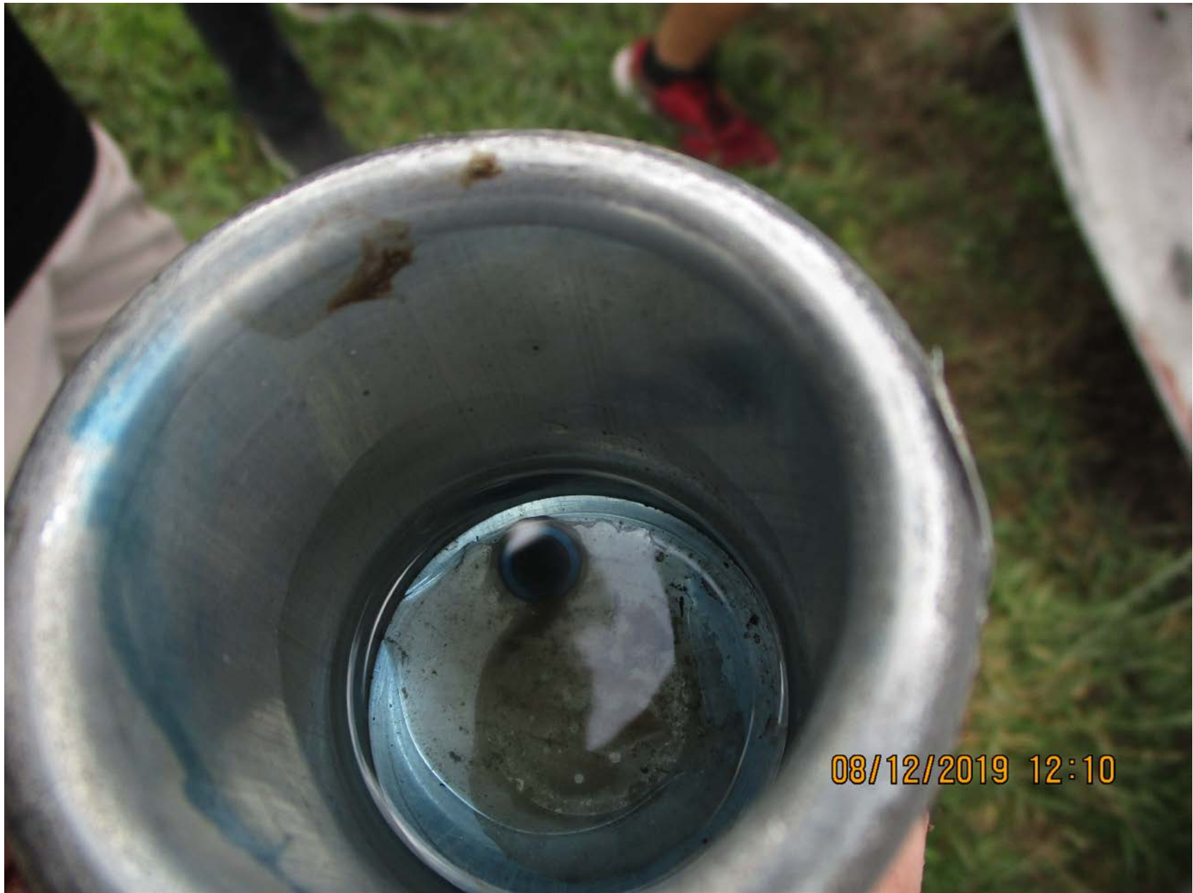
Photo 12 - FAA supplied view of the inside of the gascolator bowl.
