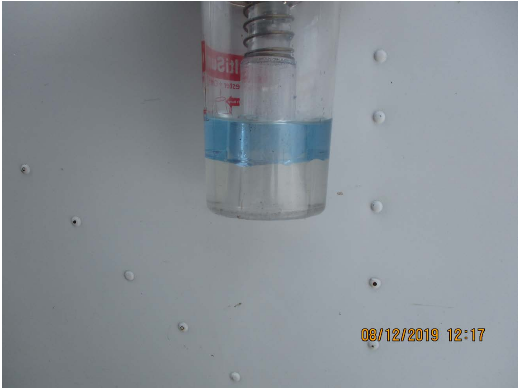
Photo 15 - FAA supplied view of a sample of liquid from the carburetor bowl. The sample contains a cloudy colored liquid at the bottom of the sampler and a blue colored liquid above the cloudy layer.
