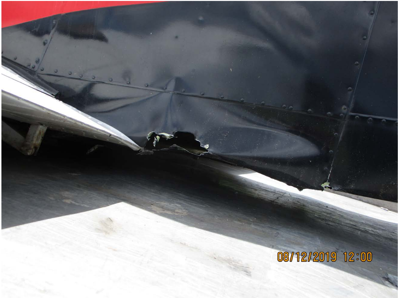
Photo 16 - FAA supplied view of damage to the left fuselage.
