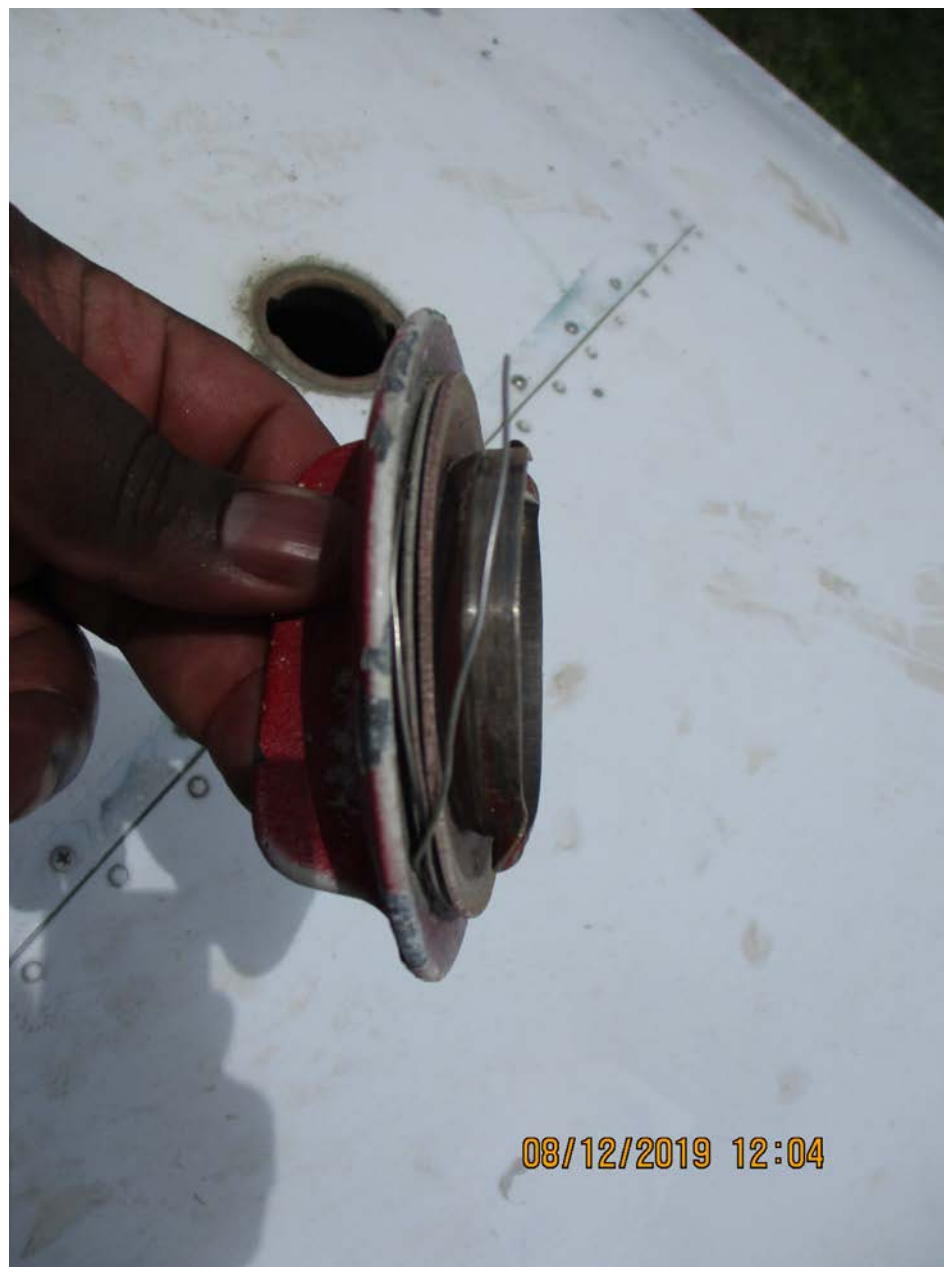
Photo 9 - FAA supplied view of a fuel cap with safety wire wrapped above its gasket.
