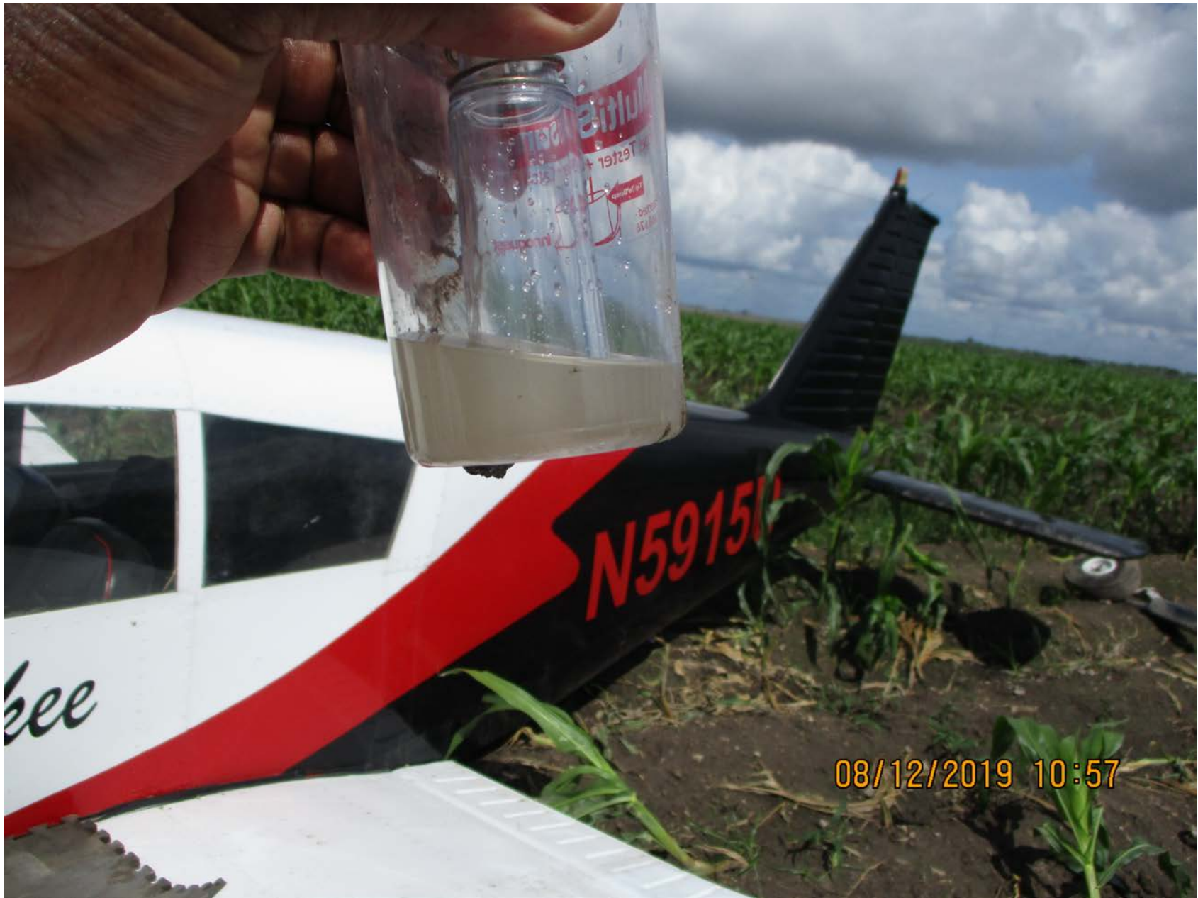
Photo 8 - FAA supplied view of a sample from the left wing's sump. The sample contains a cloudy colored liquid.
