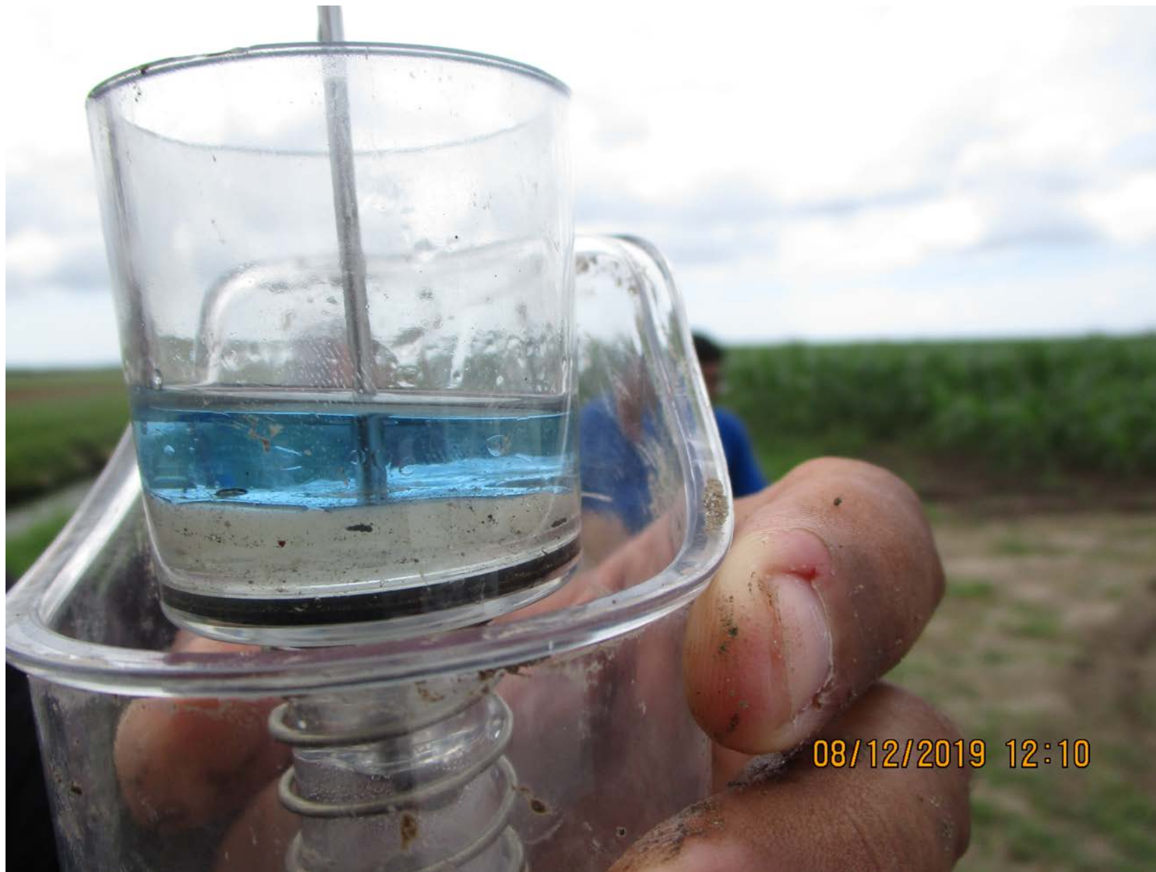
Photo 13 - FAA supplied view of a liquid sample from the gascolator bowl. The sample contains a cloudy colored liquid at the bottom of the sampler and a blue colored liquid above the cloudy layer.
