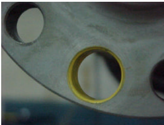
FIGURE 14 CORE SAMPLE HOLE AFTER APPLICATION OF ZINC CHROMATE PRIMER
