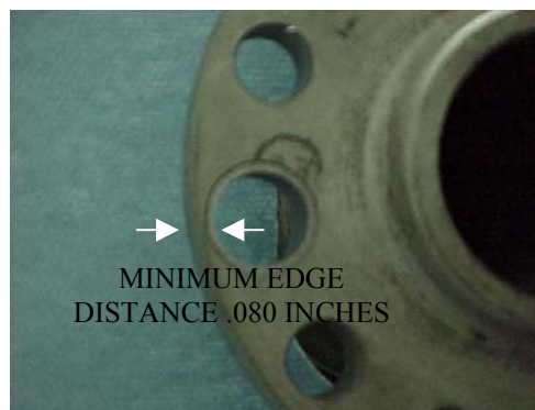
FIGURE 13 CORE SAMPLE HOLE MINIMUM EDGE DISTANCE
