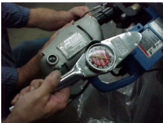
FIGURE 7 USING TORQUE WRENCH TO MAINTAIN CONSISTENT FEED RATE
