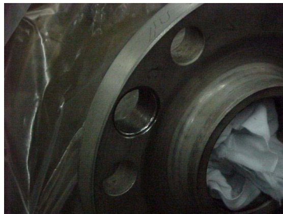
FIGURE 12 CORE SAMPLE HOLE AFTER CHAMFERING
