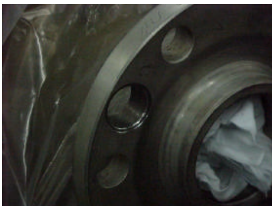
FIGURE 12 CORE SAMPLE HOLE AFTER CHAMFERING
