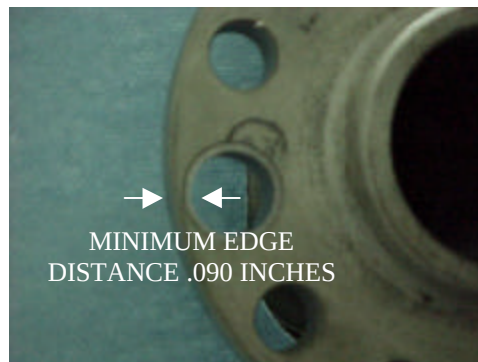
FIGURE 13 CORE SAMPLE HOLE MINIMUM EDGE DISTANCE
