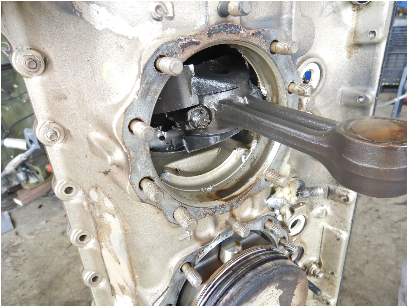
Photo 4 – Broken crankshaft is seen, behind connecting rod
