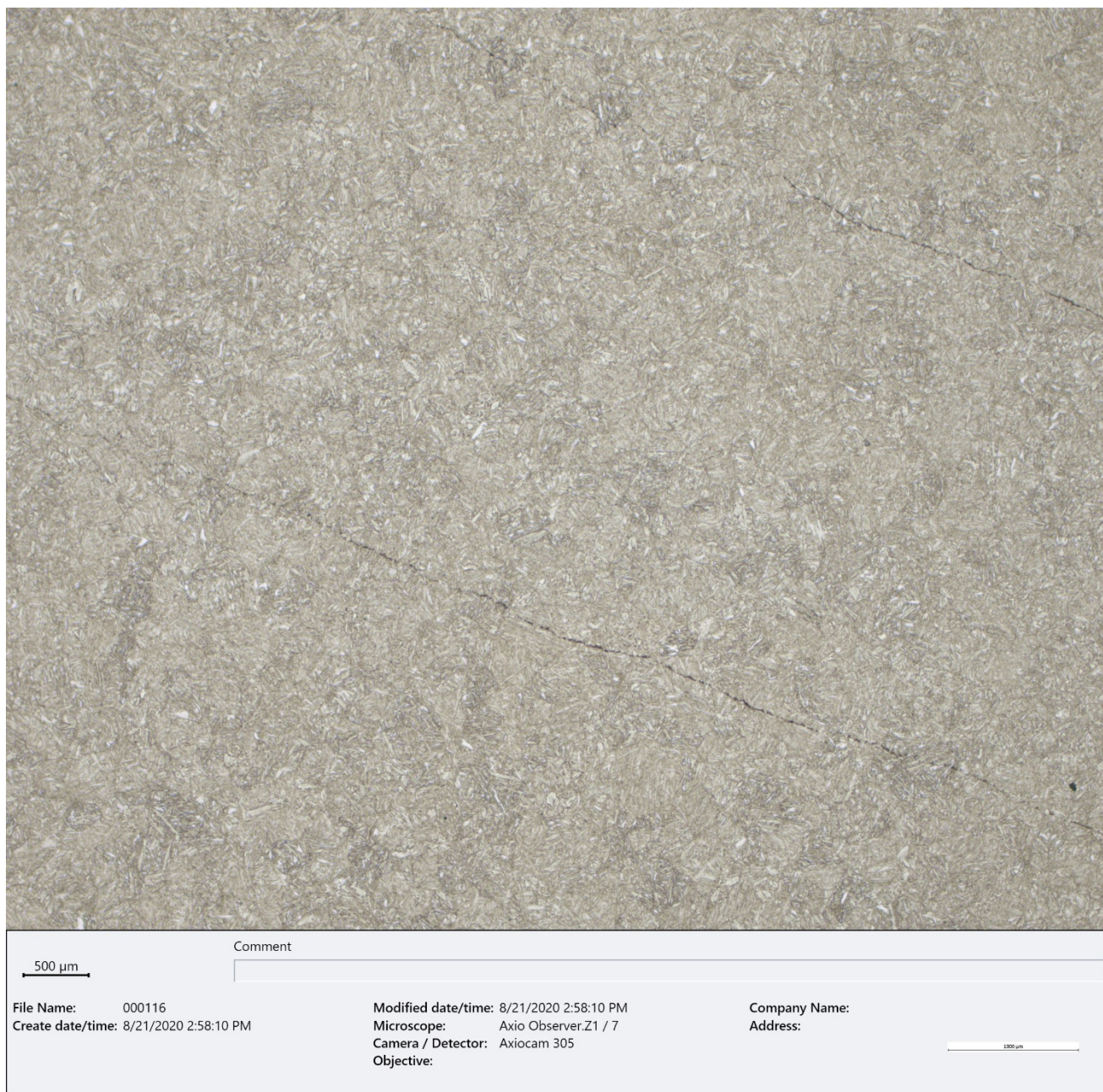
Figure 18 – BF optical micrograph of a typical area of the crankshaft web microstructure, showing tempered martensite, and thin elongated cracks (~200X, etched 2% Nital).
