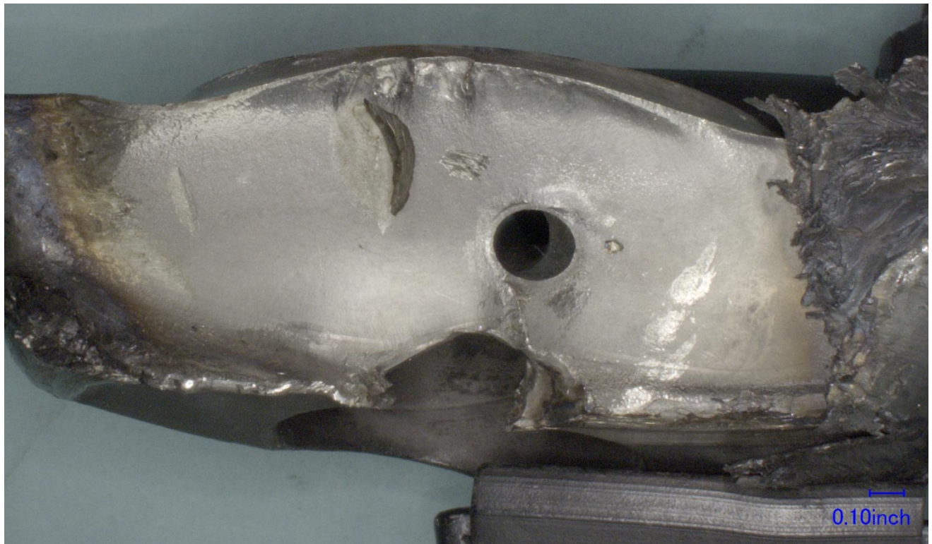
Figure 9 – View of the forward fracture surface of the fracture web, after sectioning.
