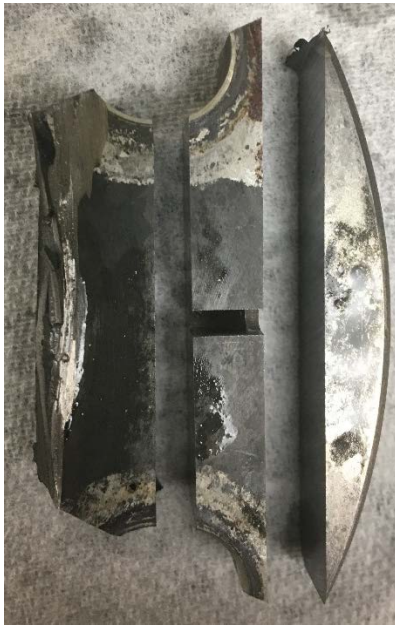
Figure 1 Section of crankshaft sectioned and notched for fracture.
