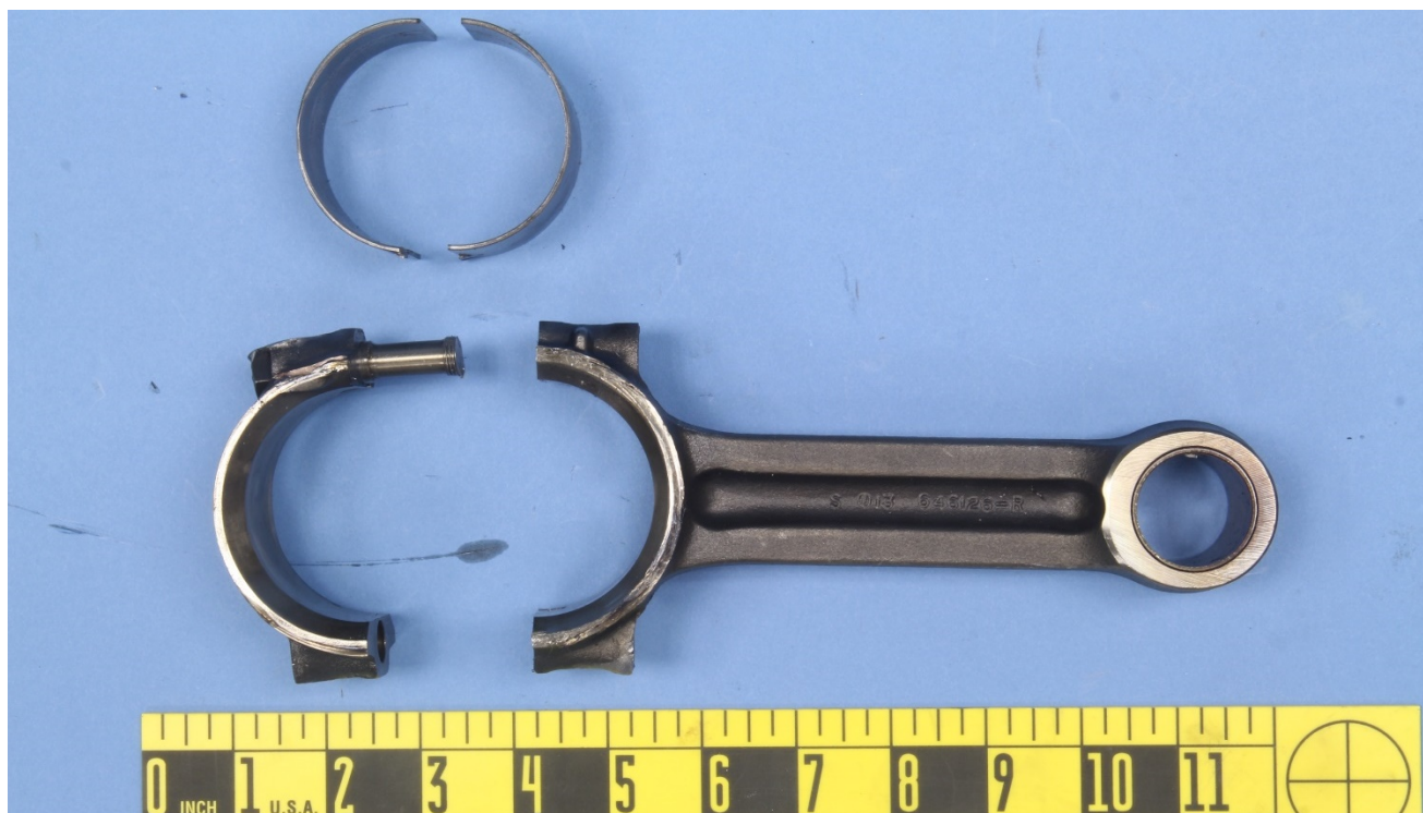
Figure 5 – View of the connecting rod and bearing from the C2 position, after disassembly.
