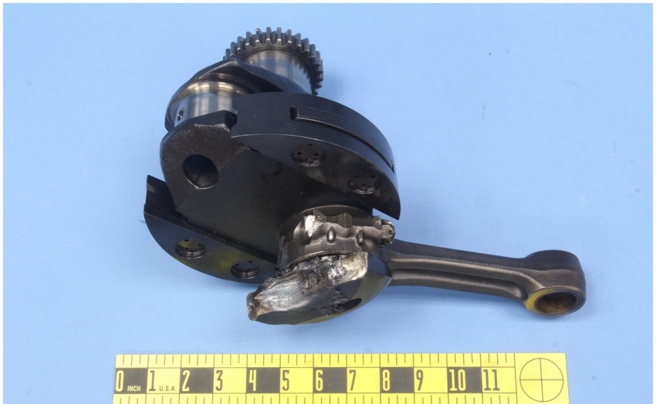
Figure 2 – View of the aft fractured piece of the crankshaft assembly, viewed forward looking aft. The fracture surface across the web adjacent to the #2 connecting rod journal is visible.
