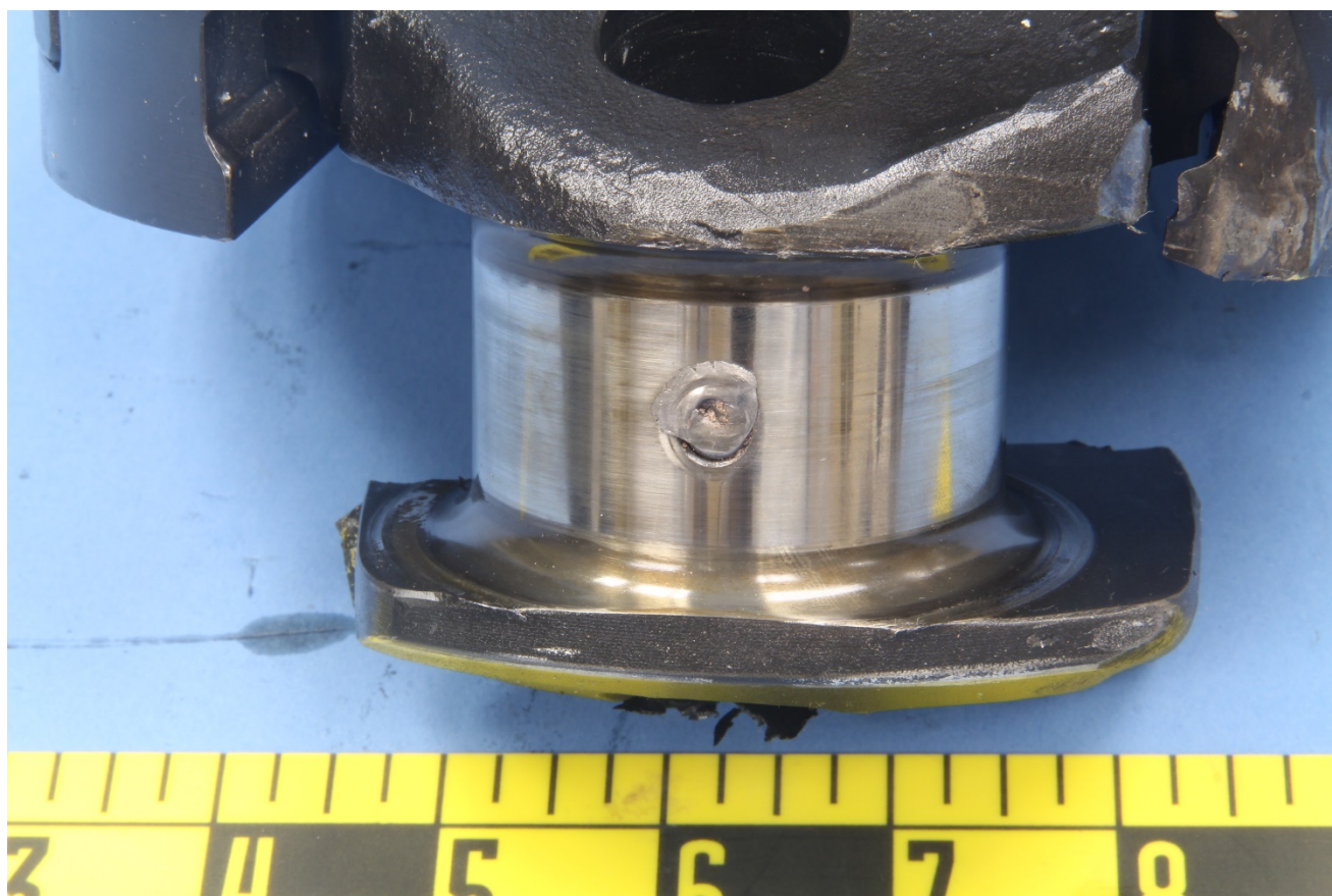
Figure 4 – View of the C2 journal adjacent to the forward side of the fractured web, showing a smeared lubrication tube in the oil lubrication hole, after removal of the connecting rod.
