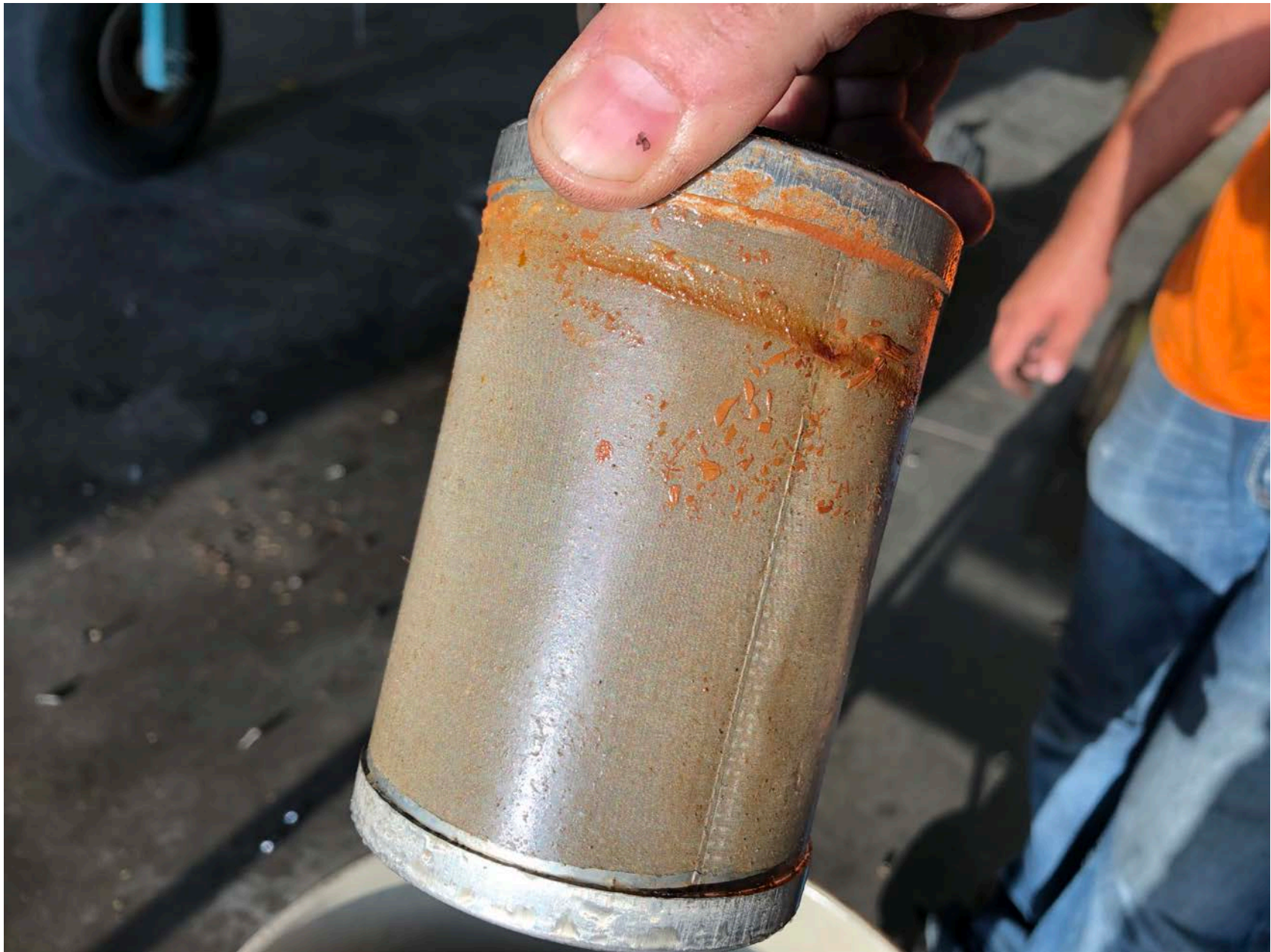
Photo 2 – Fuel filter. Photo provided by insurance company
