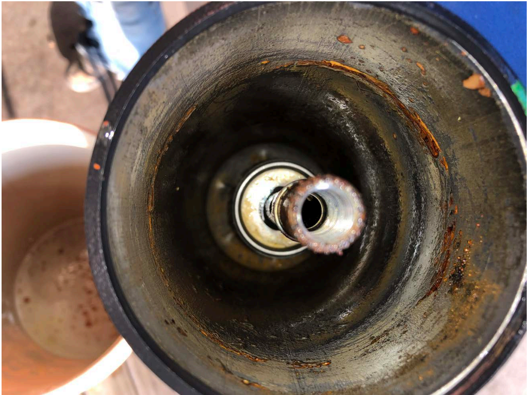
Photo 3 – Fuel filter housing. Photo provided by insurance company
