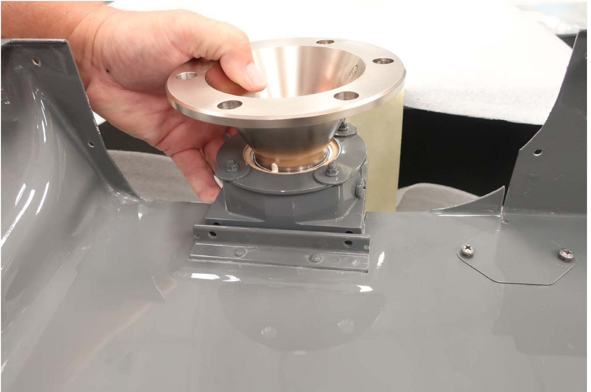
Photo 6 – Exemplar Actuator Bearing, Scroll and Bracket
