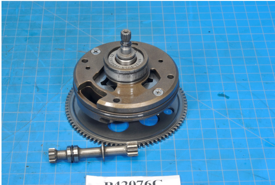
Photo 24 – Oil Scavenge Pump - Undamaged
