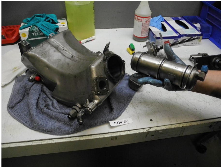
Photo 22 – Fuel/oil Heater - Undamaged
