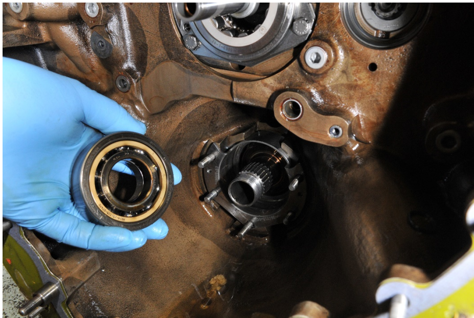
Photo 19 – Compressor Bearing - Undamaged
