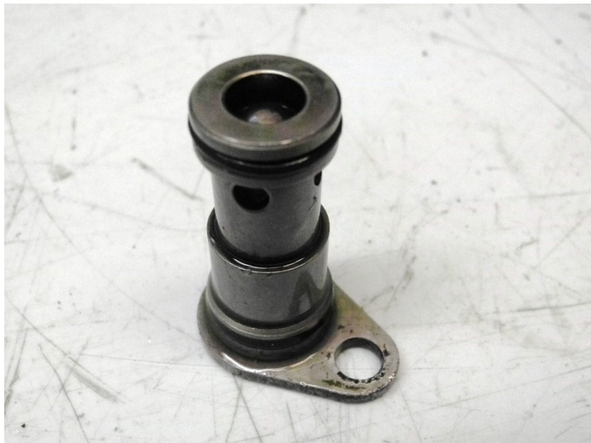
Photo 23 – Oil Pressure Regulating Valve - Undamaged
