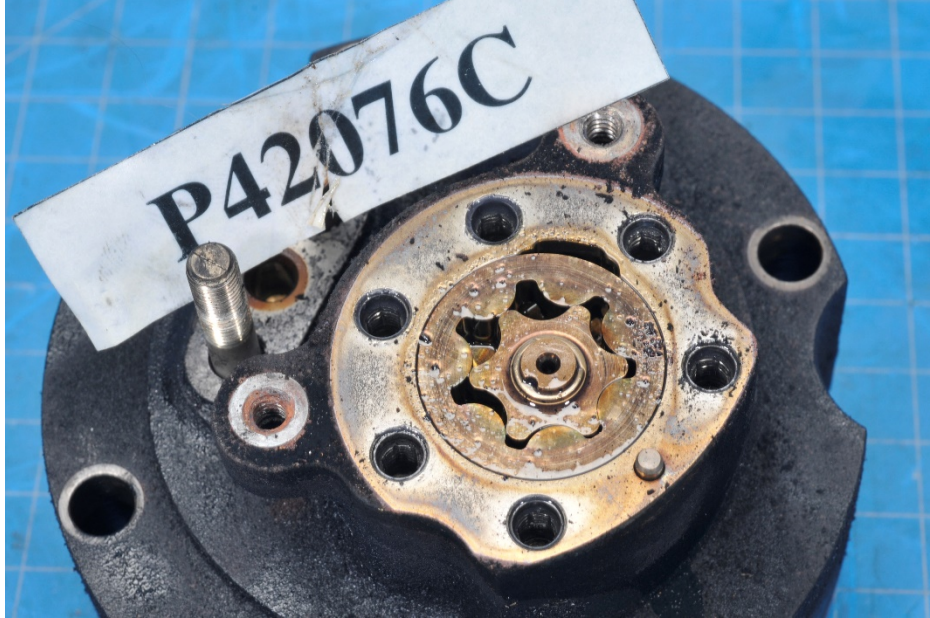
Photo 26 - Turbine Bearing Scavenge Pump - Undamaged
