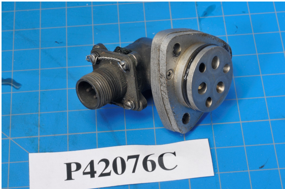
Photo 27 – Oil Vent Valve
