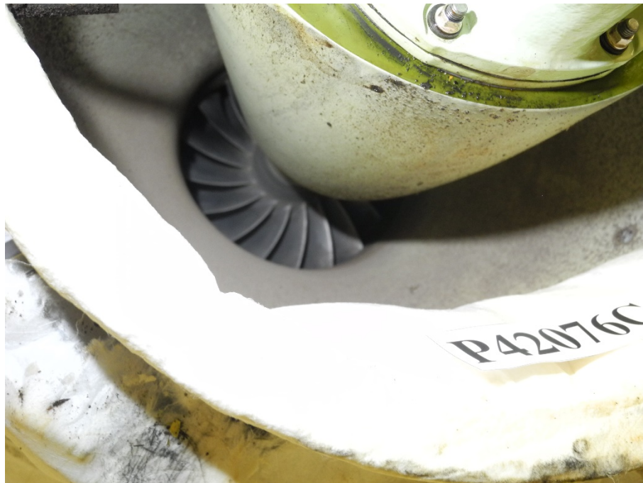
Photo 11 – 1 st Stage Impeller – Undamaged and Oil Free
