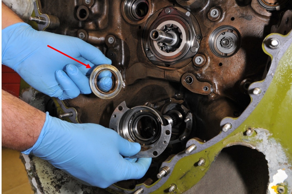
Photo 20 – Compressor Bearing Carbon Seal - Undamaged
