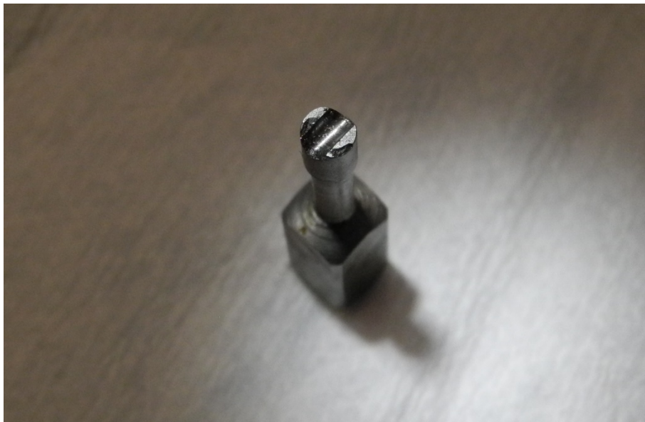
Photo 13 – Tach-Generator Drive Shaft - Fractured
