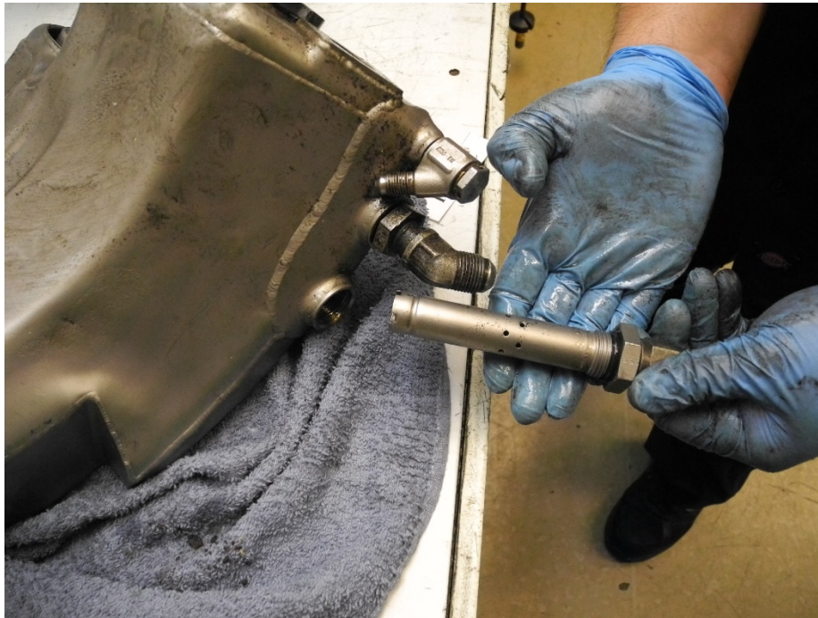
Photo 21 - Air/Oil Separator - Intact and Undamaged
