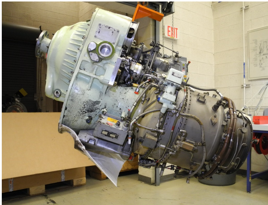
Photo 5 - Nose Cone, Gearbox Housing and Compressor Housing - Undamaged
