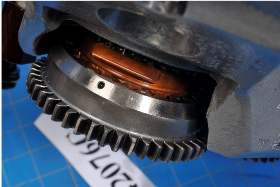
Photo 18 – Torque Sensor Helical Gearshaft & Spur Gear and Cam Assembly – Seized
