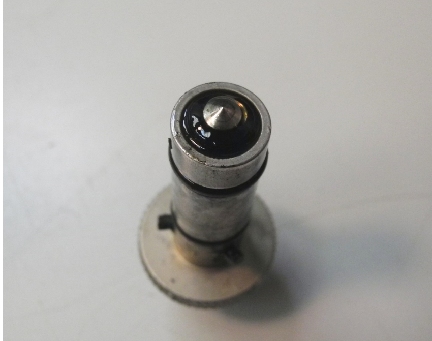
Photo 6 - Nose Cone Chip Detector - Clean
