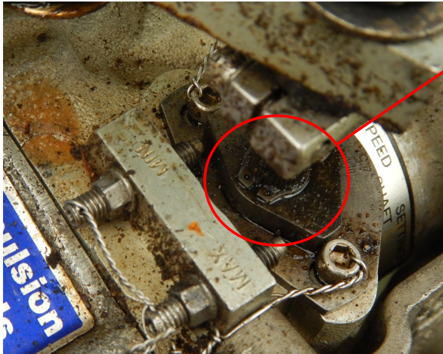
Photo 37 – FCU & Fuel Pump Assembly – General Oil Wetting
