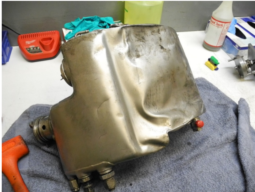
Photo 9 – Oil Tank – Removed from Engine – Dented & Unbreached
