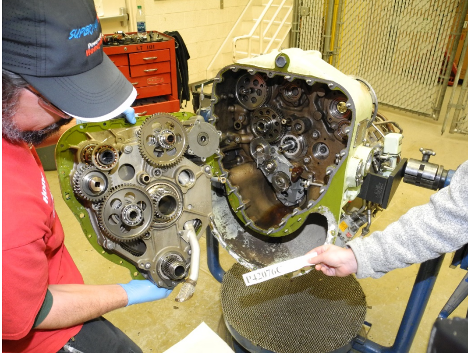
Photo 16 – Gearbox Housing – Undamaged & Oil Wetted
