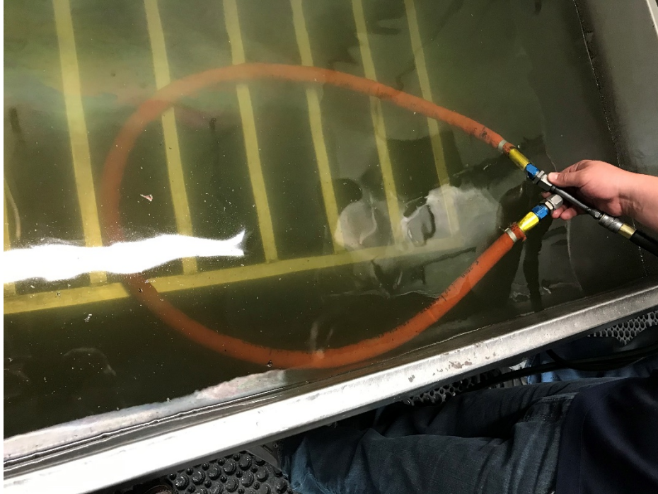
Photo 32 - Flex-Hose (1) with 100 psi Air Pressure in Tank – No Leaks
