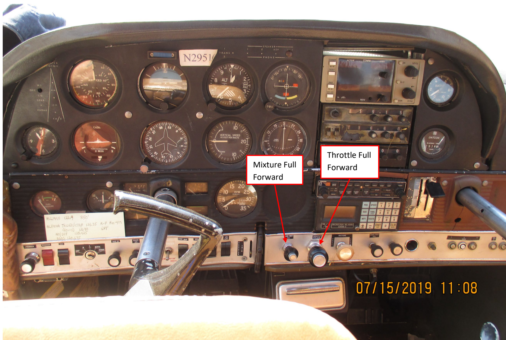
Photo 2 – Airplane Instrument Panel as Observed After the Accident (Courtesy of FAA)
