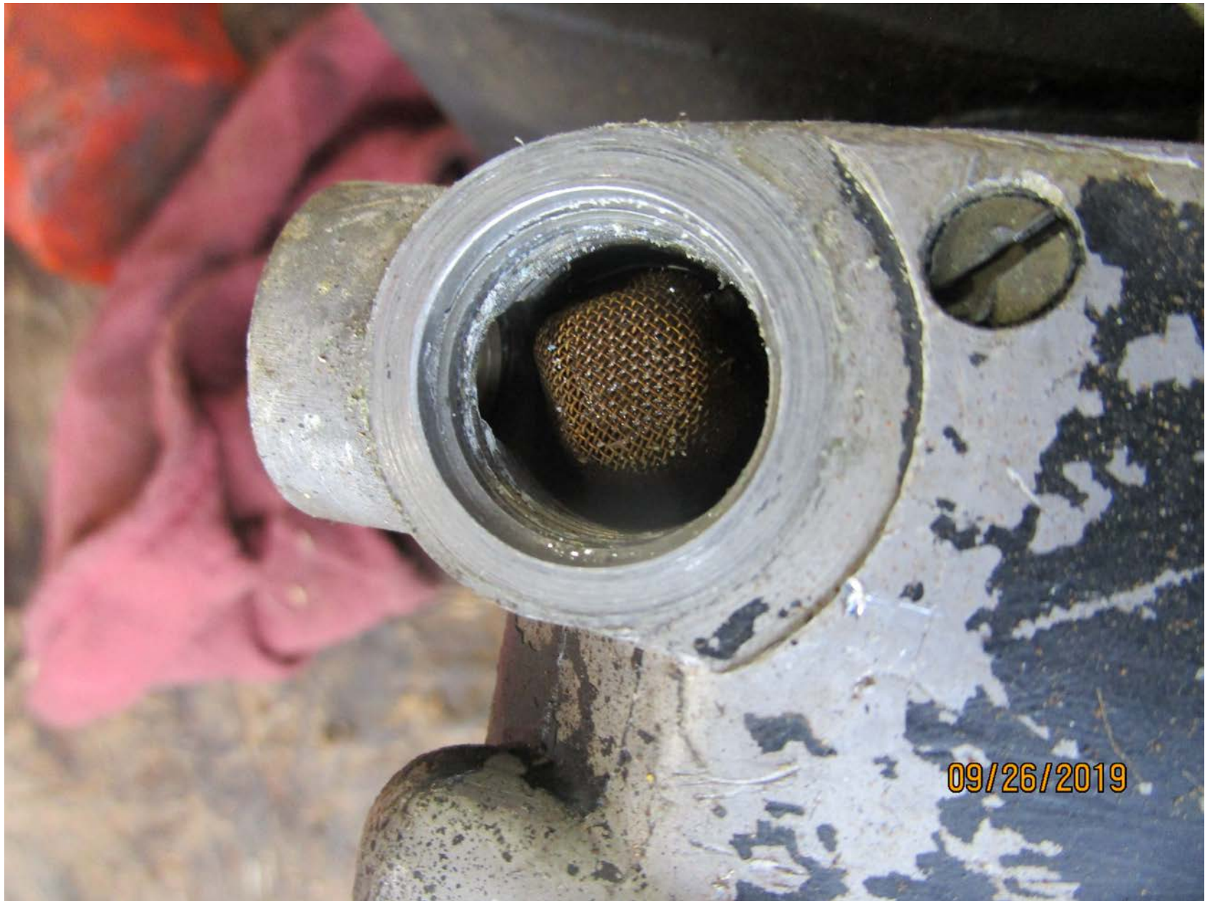
Photo 17 - View of the fuel screen.
