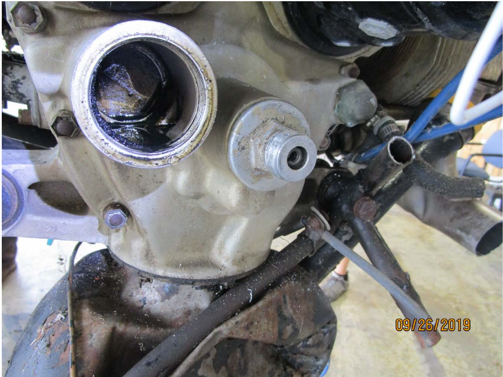
Photo 15 - View of the oil screen cavity.
