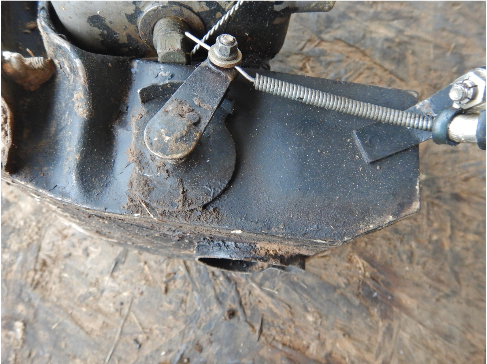
Photo 10 - Close-up view of the carburetor heat linkage.
