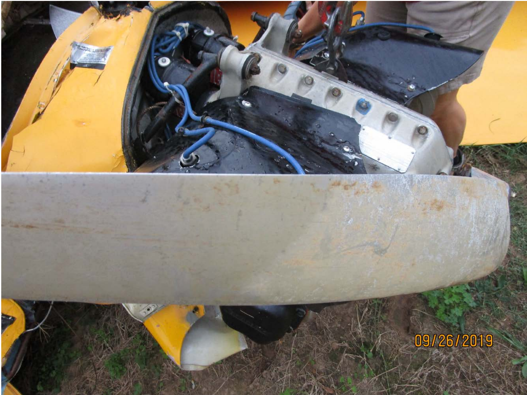
Photo 1 – View of chordwise abrasion on a propeller blade.
