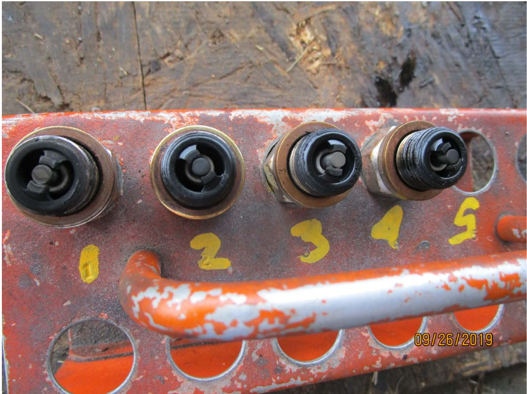
Photo 13 - Close-up view of removed sparkplugs.
