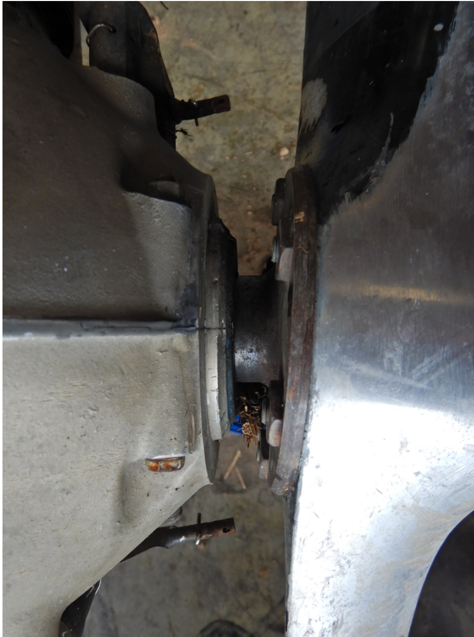
Photo 20 - View of the bent crankshaft and propeller flange.
