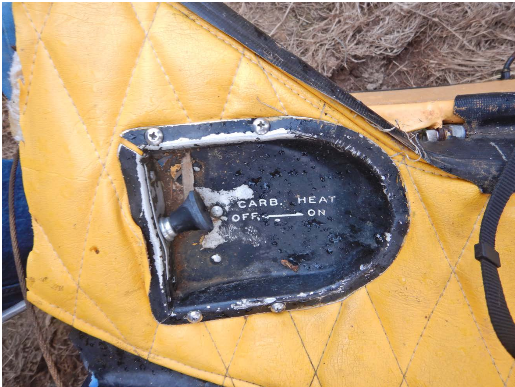
Photo 4 - View of the carb heat selector. The selector is in the OFF position.
