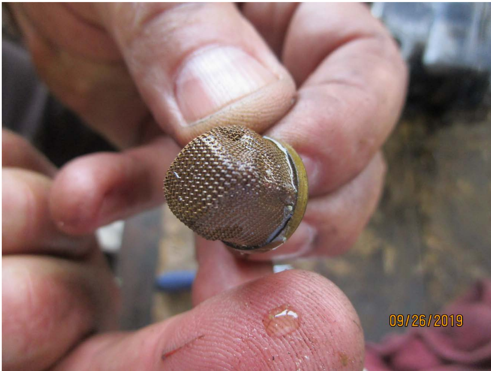
Photo 18 - View of the removed fuel screen.
