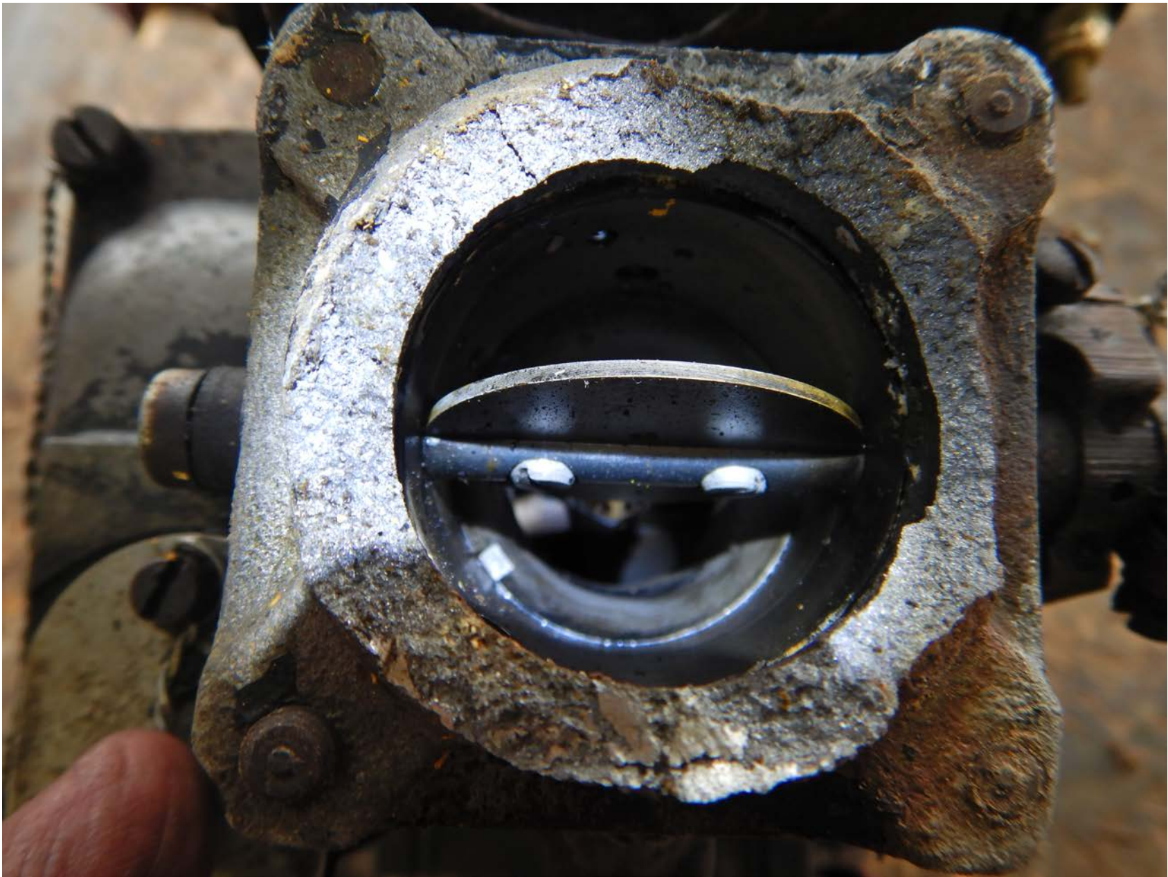
Photo 19 - View of the separated section of the carburetor venturi and butterfly throttle valve.
