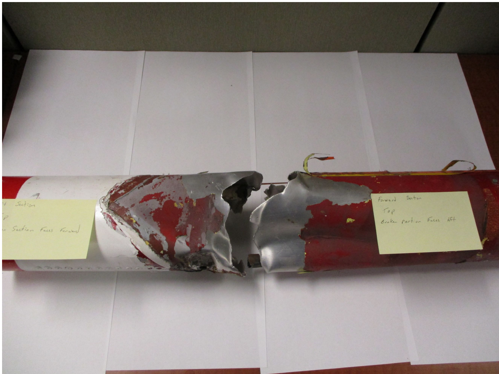
Photo 4 – A sectioned piece of the fractured tail section
