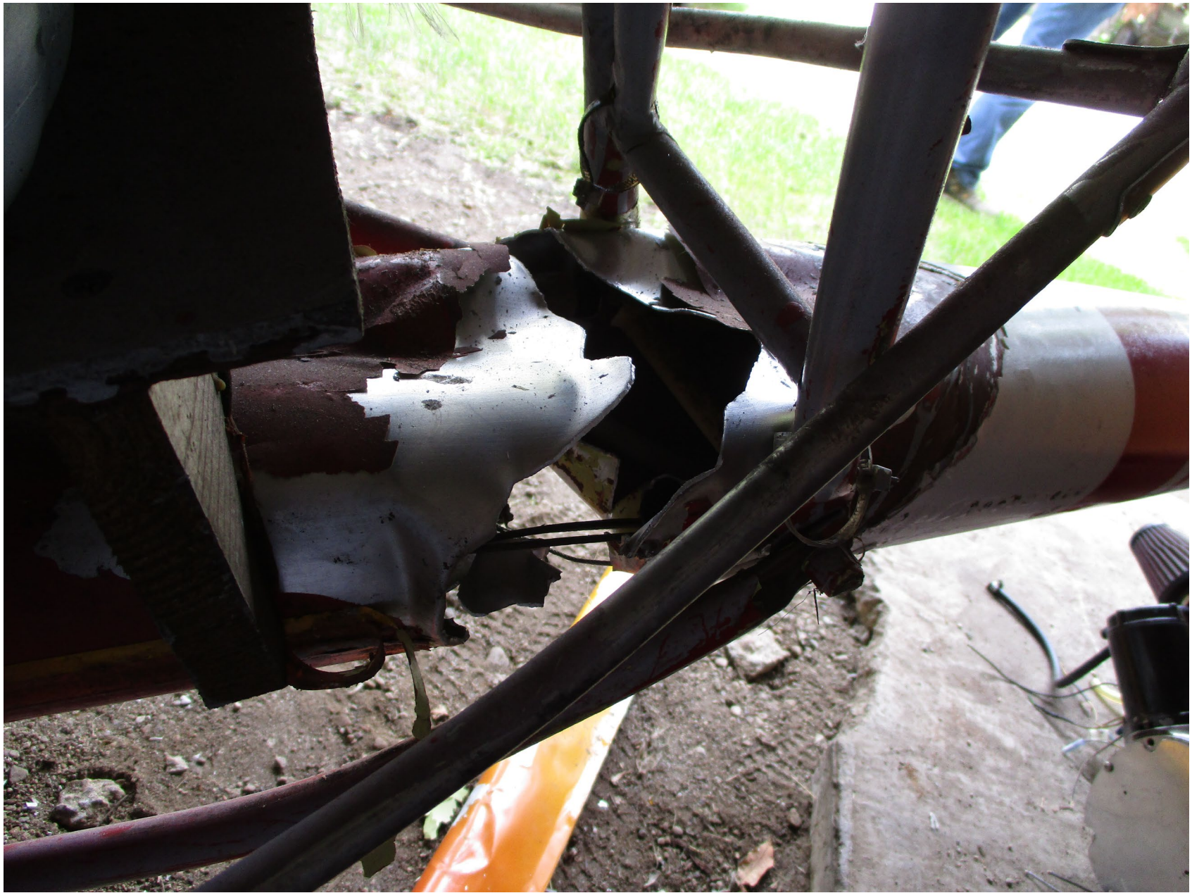
Photo 2 – Fractured tail section
