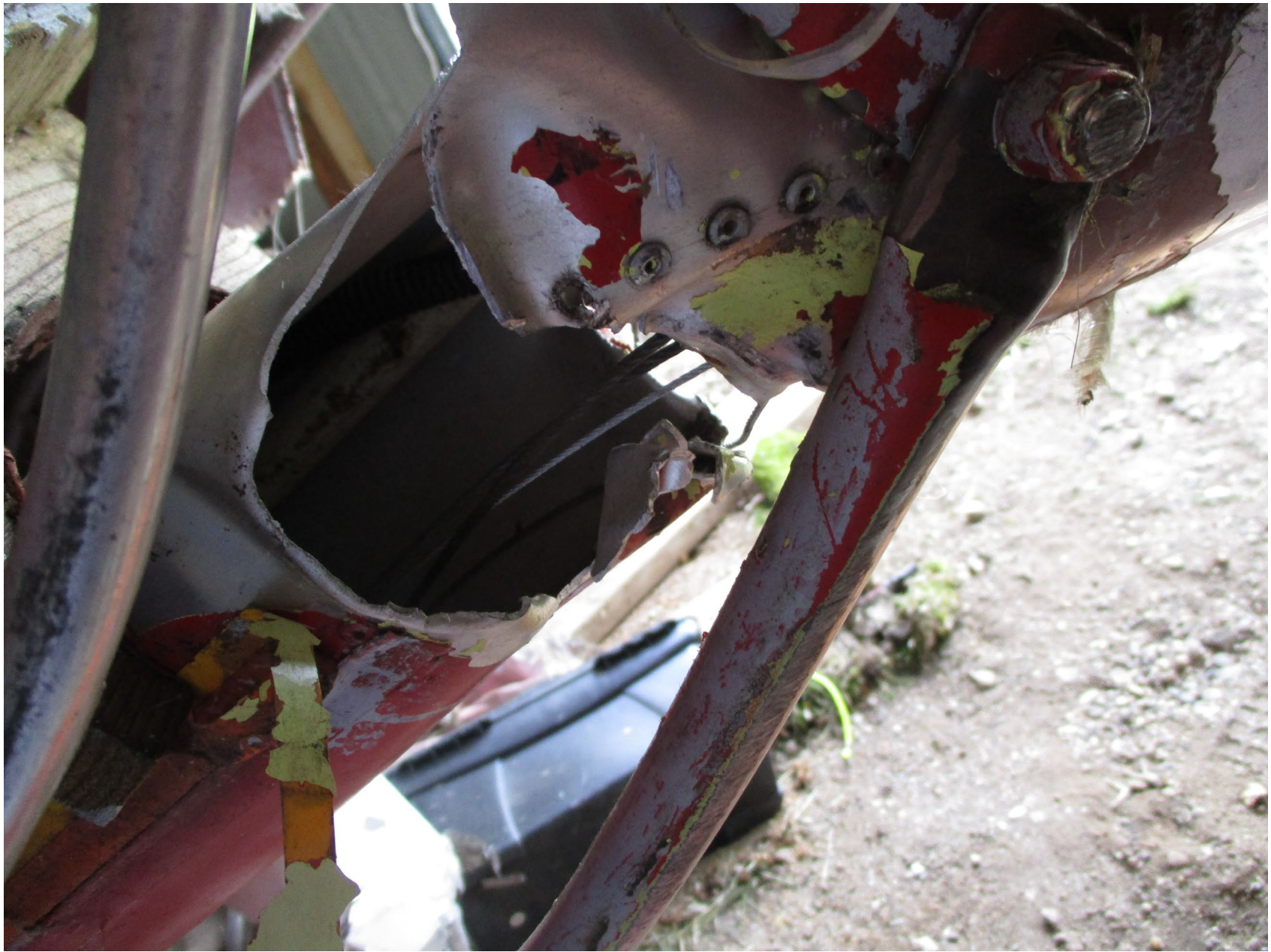
Photo 3 – Fractured tail section
