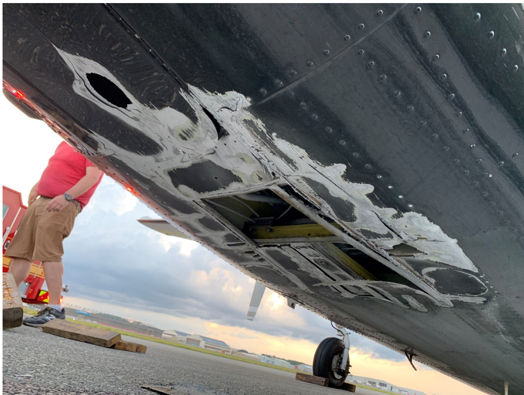
Figure 2: Damage to Lower Airplane Skin and Structure
