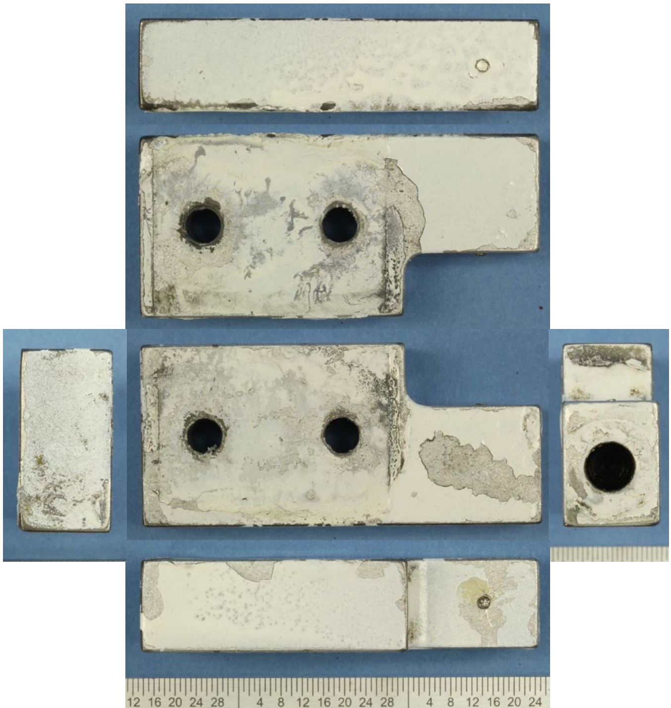
Figure 1 Image of the as-received nose gear spacer with fractured split spring pin pieces.
