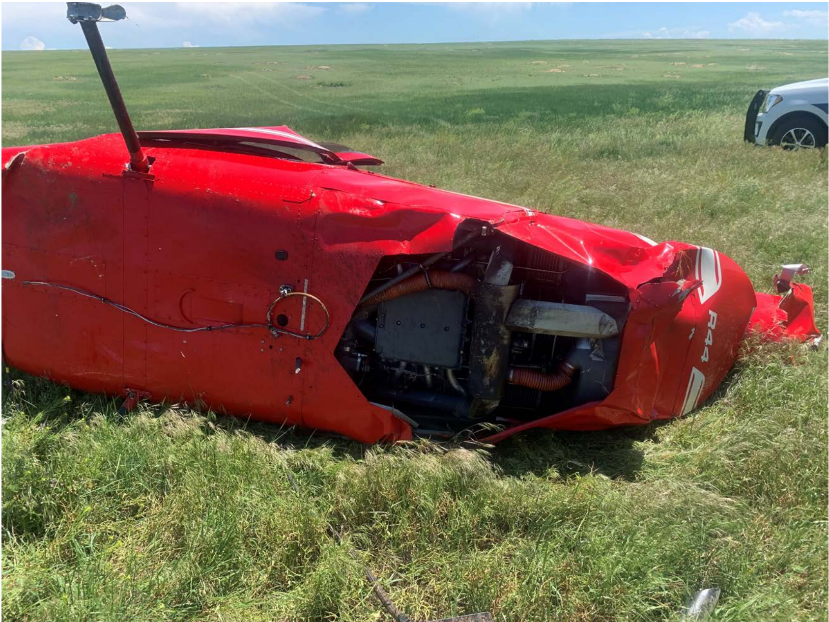
Photo 2 – Belly damage (courtesy of FAA)
