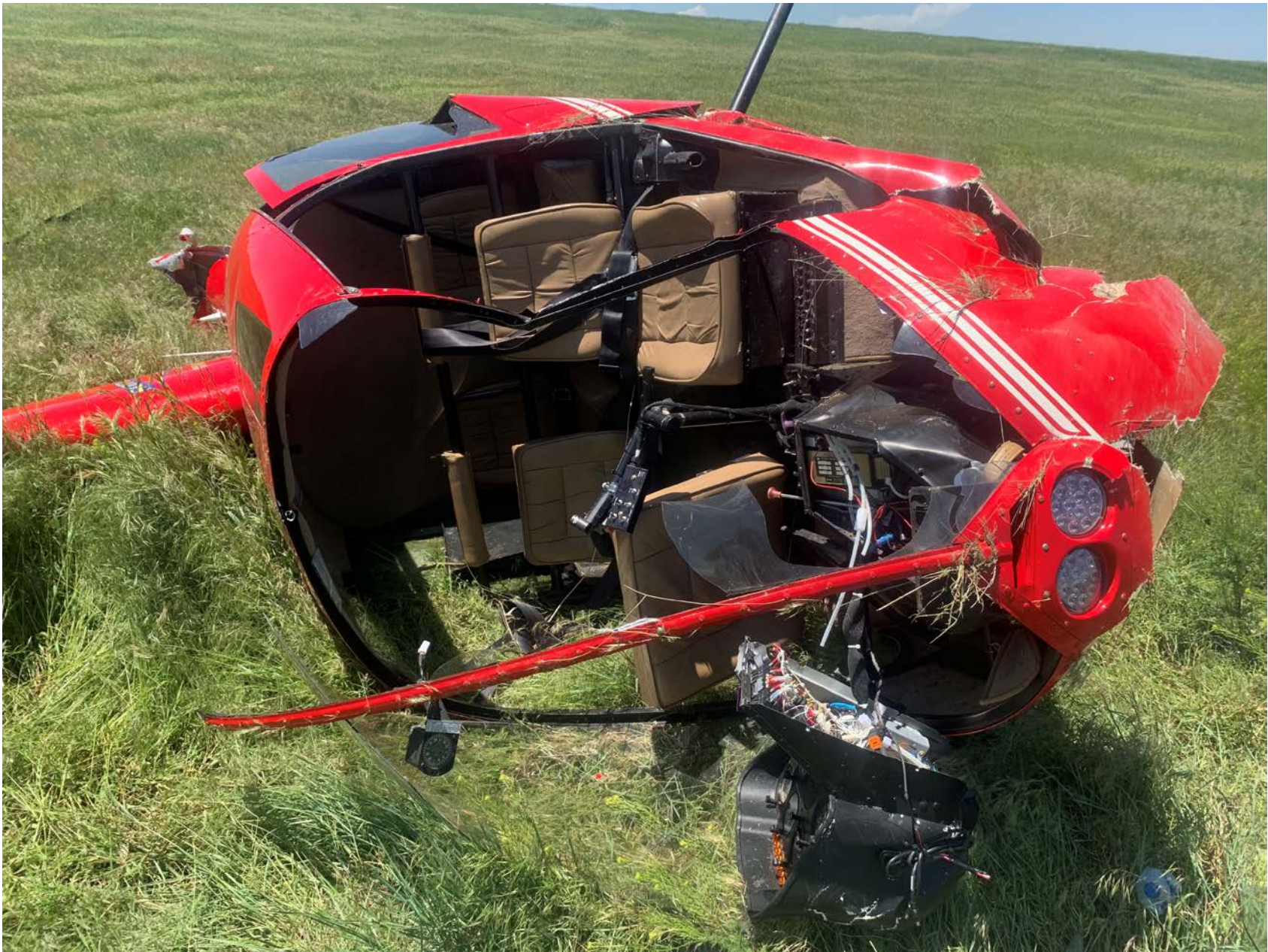
Photo 3 – Cockpit damage (courtesy of FAA)
