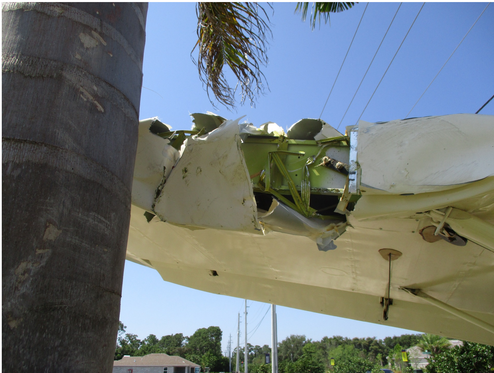
Photo 12 - FAA supplied close-up view of a tree and damage to the right wing leading edge.
