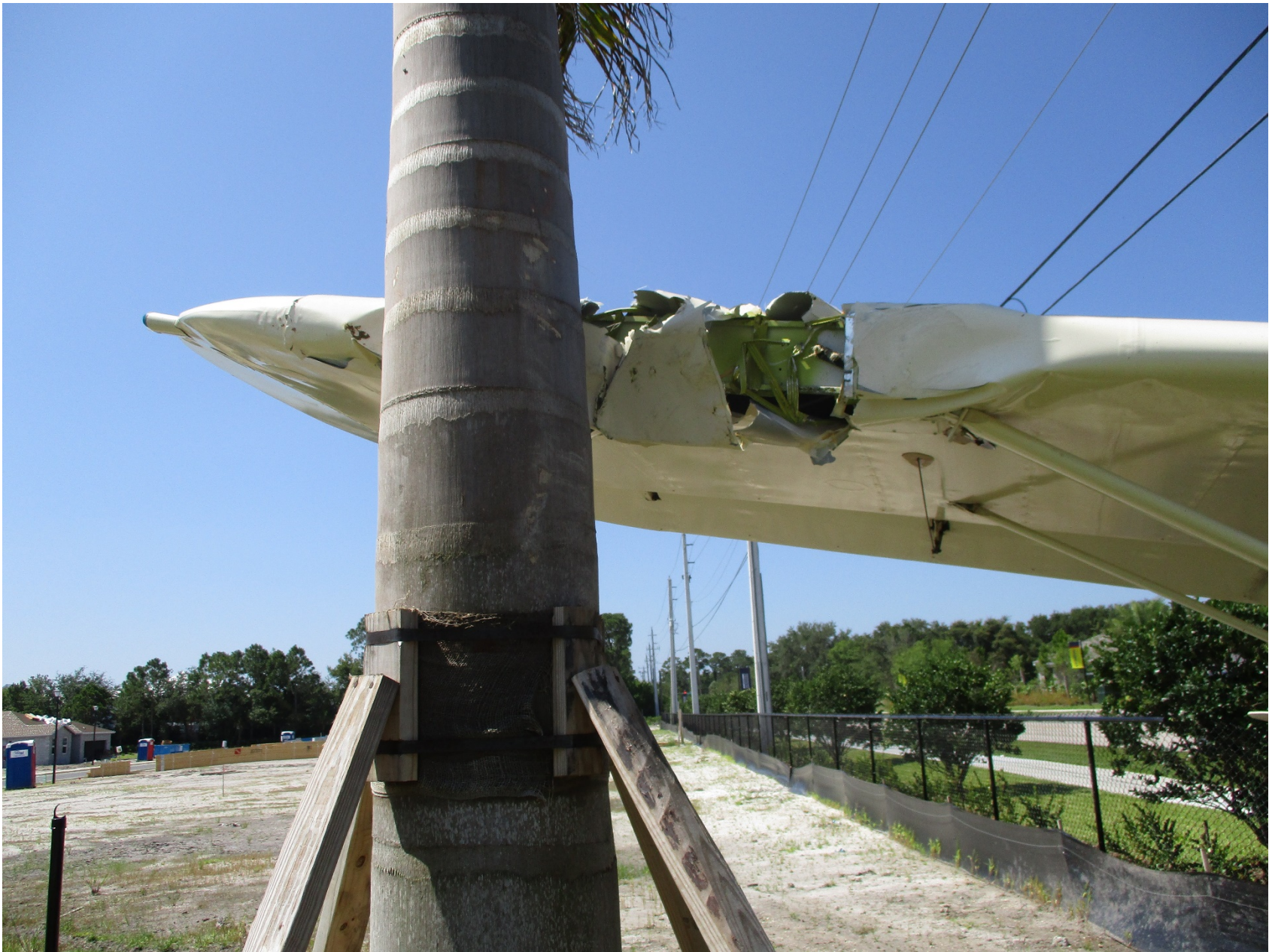
Photo 11 - FAA supplied view of a tree and damage to the right wing leading edge.
