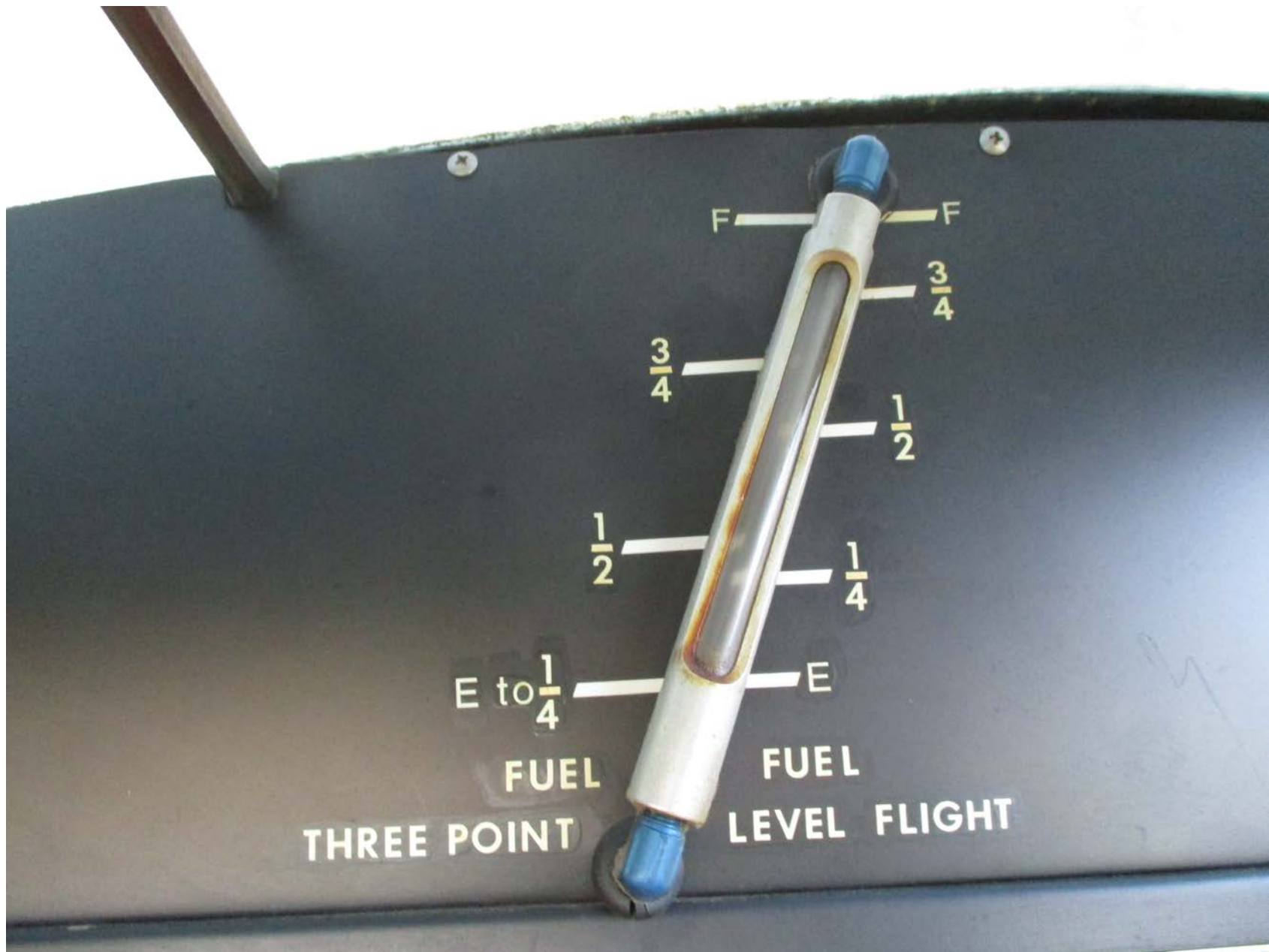
Photo 5 - FAA supplied view of a fuel sight glass.
