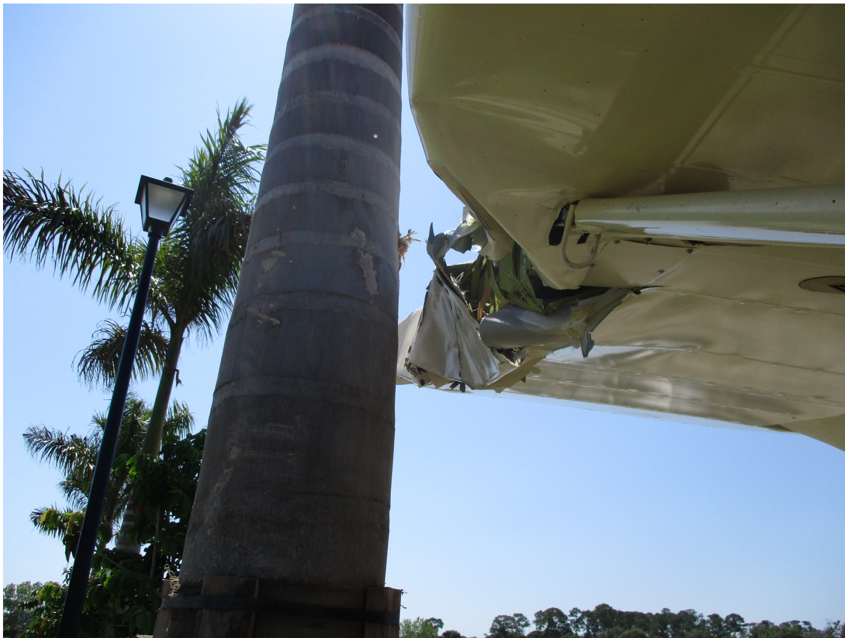
Photo 10 - FAA supplied view of a tree and damage to the right wing leading edge.
