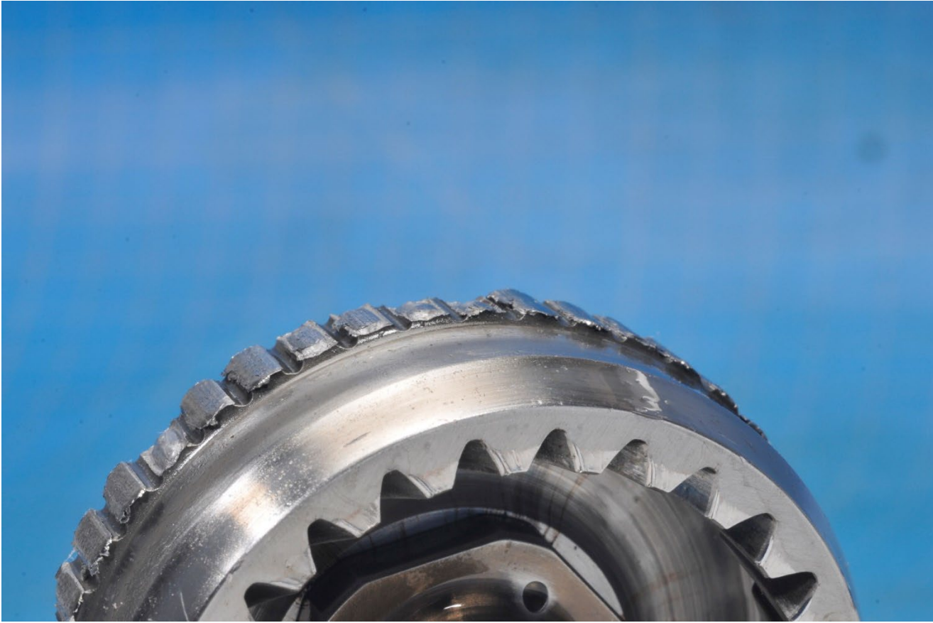
Photo 3 Closeup of Helical Cam Gear Teeth
