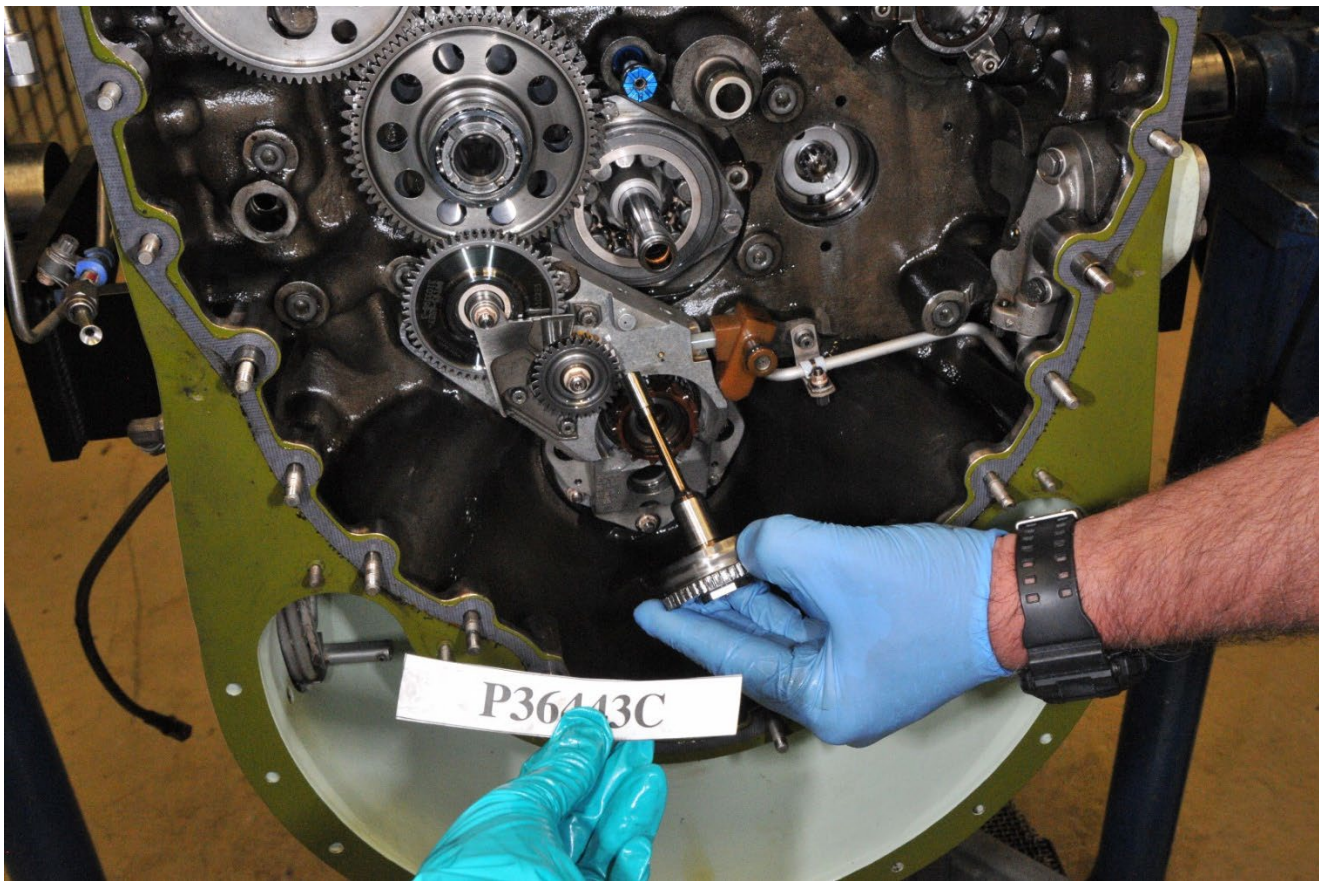
Photo 1 Helical Cam Gear as found during Teardown Examination
