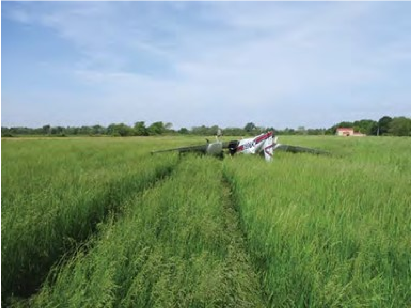
Photo 2 – Landing Gear Tracks Leading to Airplane Wreckage
