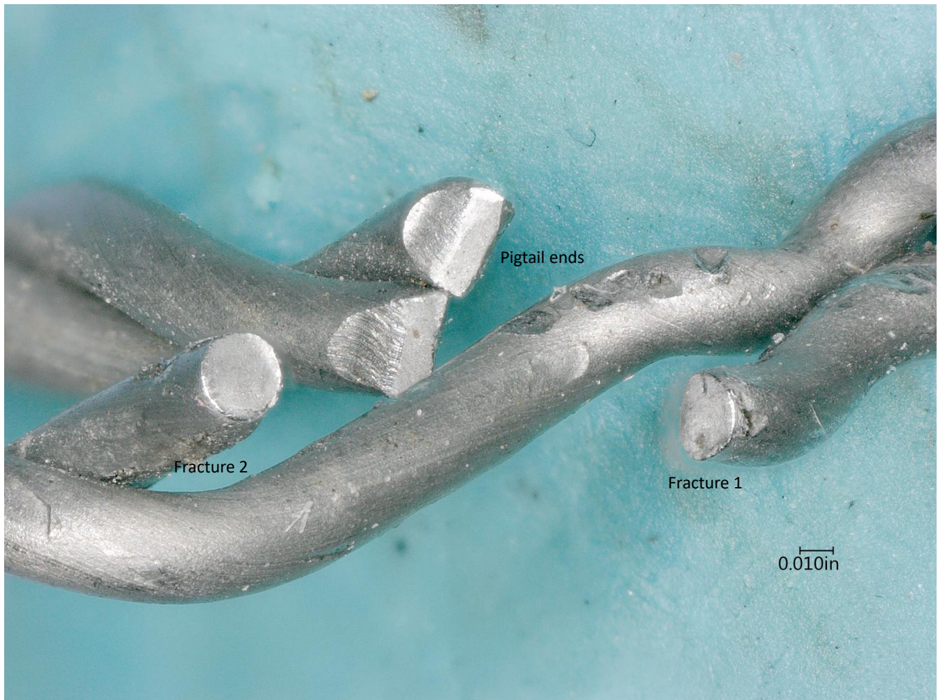
Figure 19 Oblique view of the safety wire to reveal the fracture surfaces and the terminal cuts on the pigtail.
