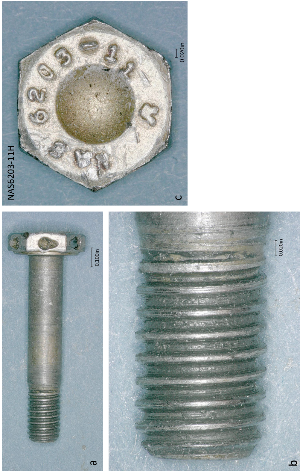
Figure 9 Close views of the threads and head markings on the right aileron hinge attachment bolt.
