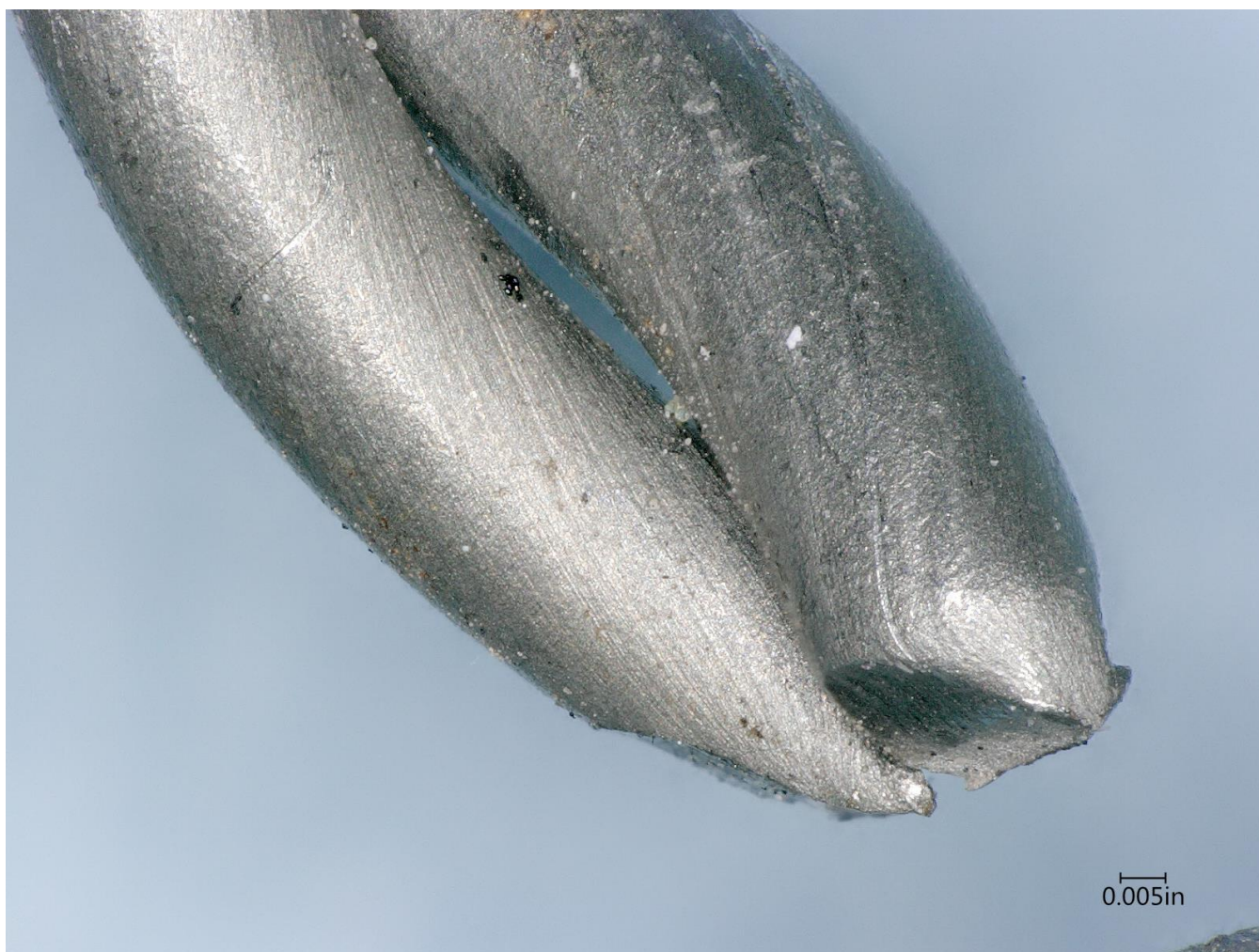
Figure 20 Higher magnification image of the plier-cut terminal-end of the safety wire pigtail.
