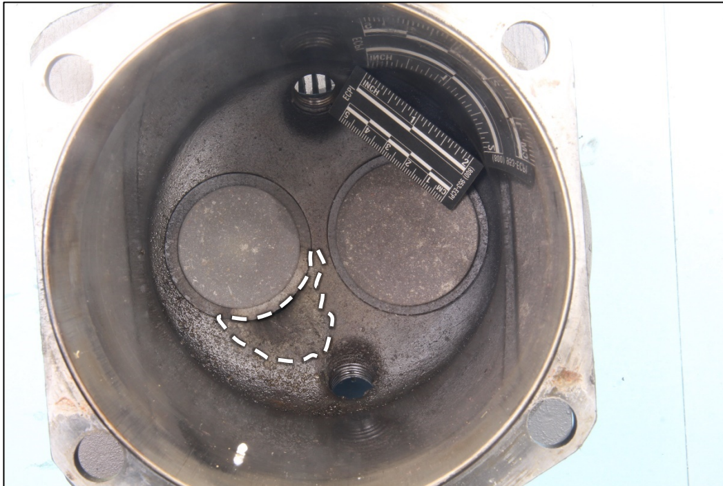
Figure 3. Interior of the number 2 cylinder assembly from the right engine. A dashed line indicates an area of missing cylinder head material between the exhaust valve and one of the spark plug ports.
