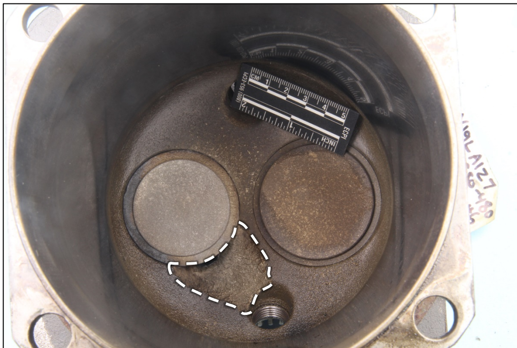
Figure 2. Interior of the number 6 cylinder assembly from the left engine. A dashed line indicates an area of missing cylinder head material between the exhaust valve and one of the spark plug ports.
