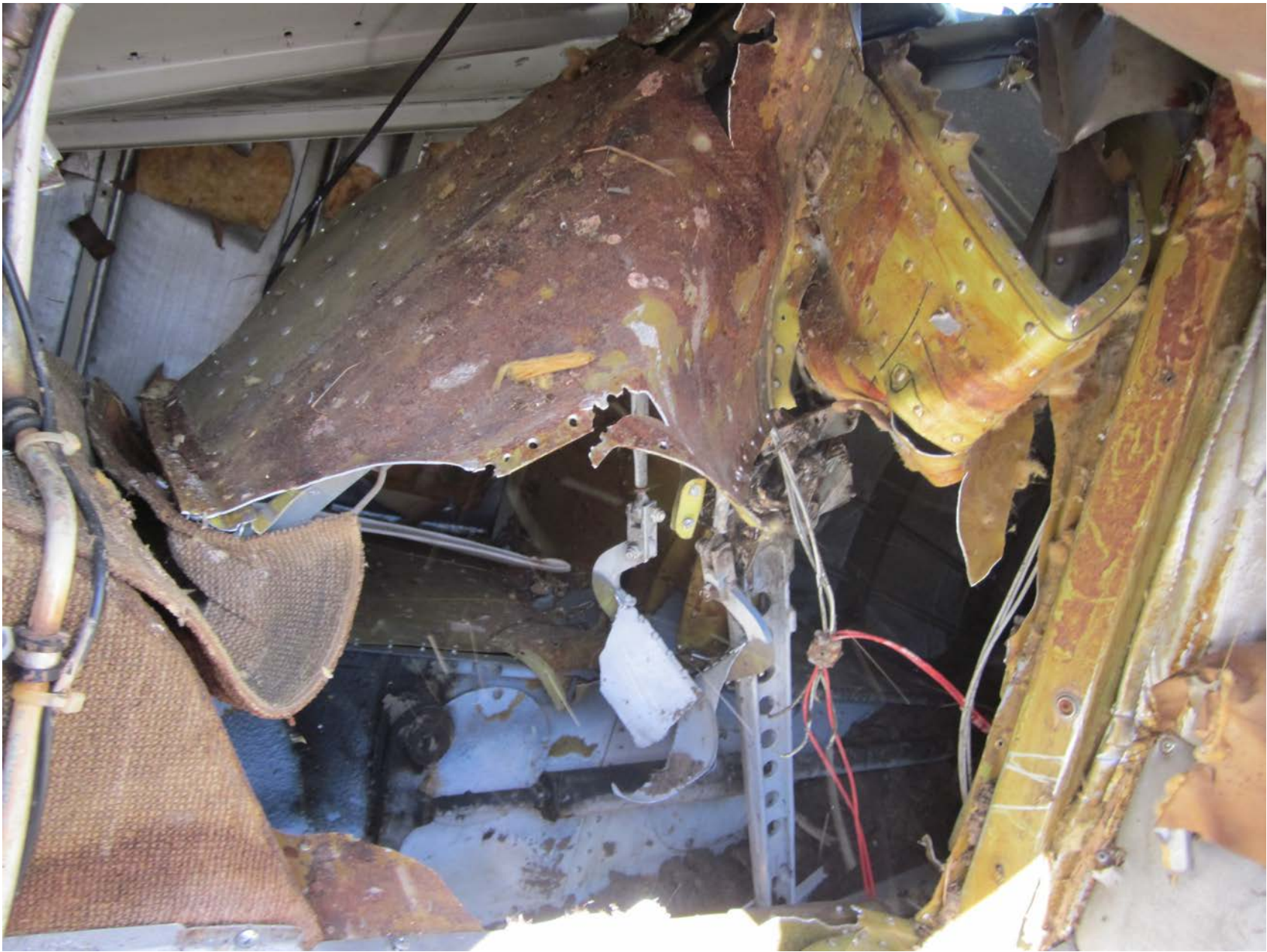
Photo 3 – View of the damage to the fuselage (courtesy of the Federal Aviation Administration).
