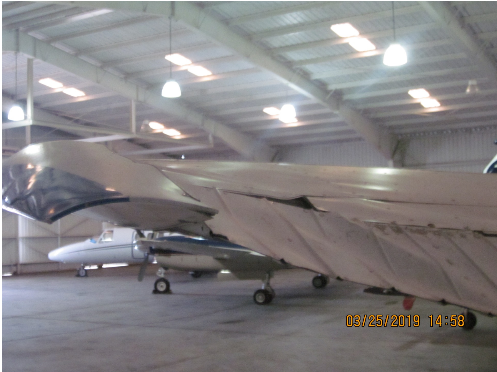
Photo 1 – Damage to Left Wing Aileron and Upper Wing Skin (Courtesy of FAA)
