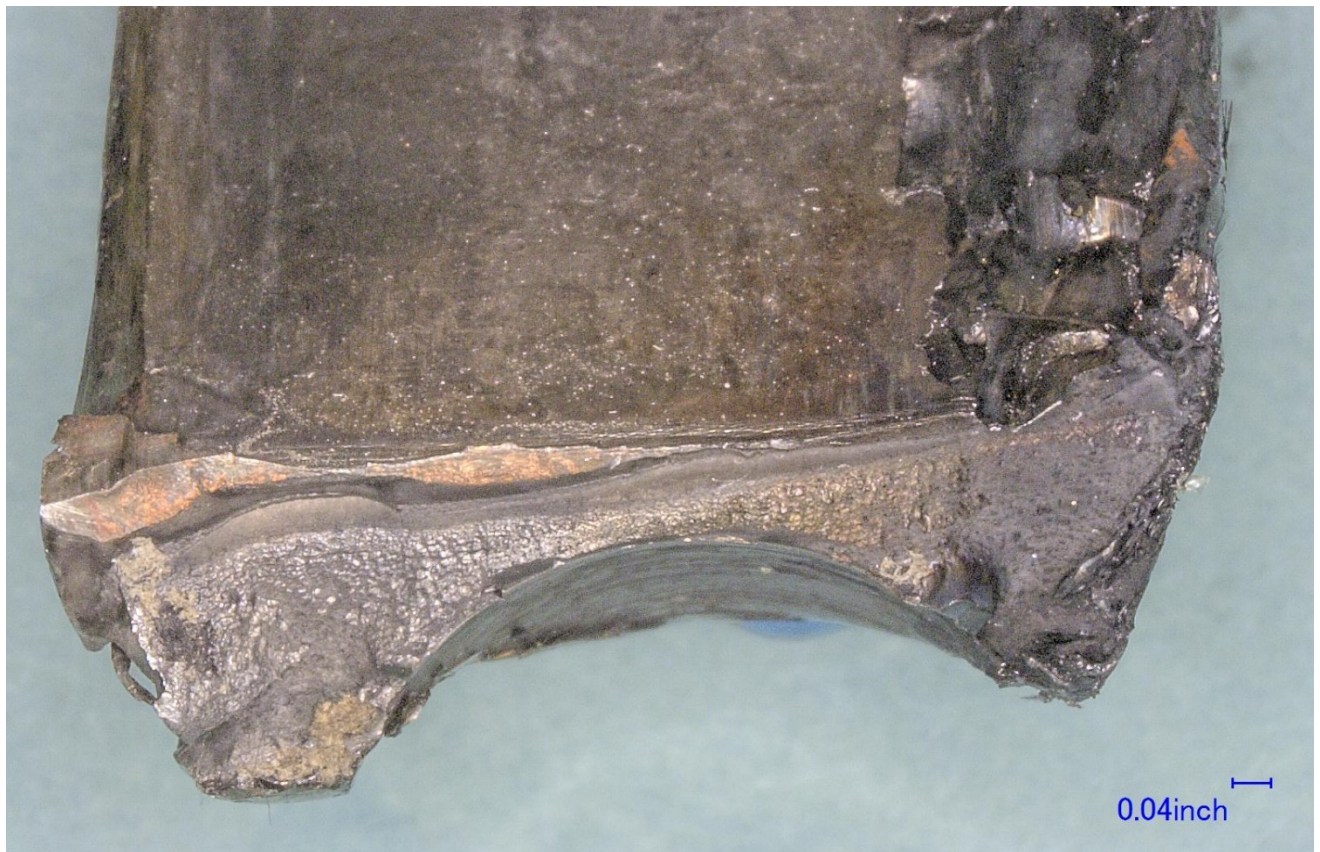
Figure 19 – View of the less damaged area of the fracture surface of the #4 connecting rod.
