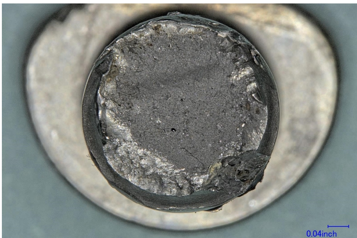
Figure 14 – View of the upper mating face of the bolt fracture surface.
