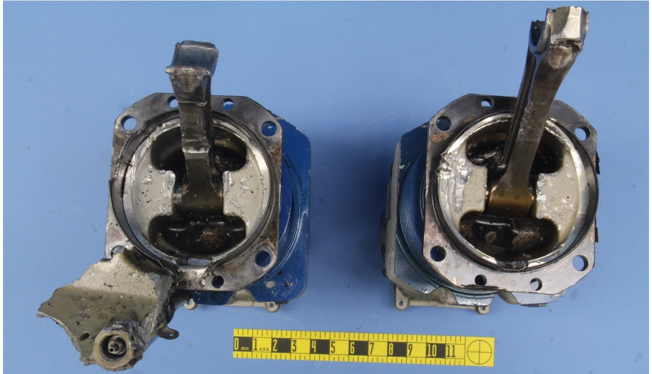
Figure 6 – View of the connecting rod sides of the cylinder assembly remnants from the #4 and #6 cylinders, with the rods moved upward from Figure 4, showing cylinder damage.
