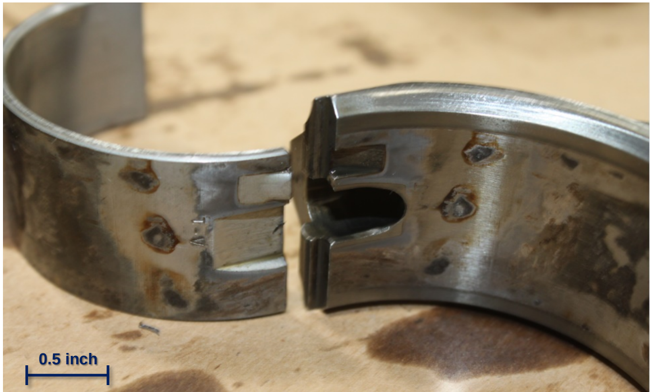
Figure 4 – View of the mating bearing surfaces of the #3 connecting rod surface and the outer bearing surface, showing three matching marks (courtesy Tim Sorensen, AS-CEN).
