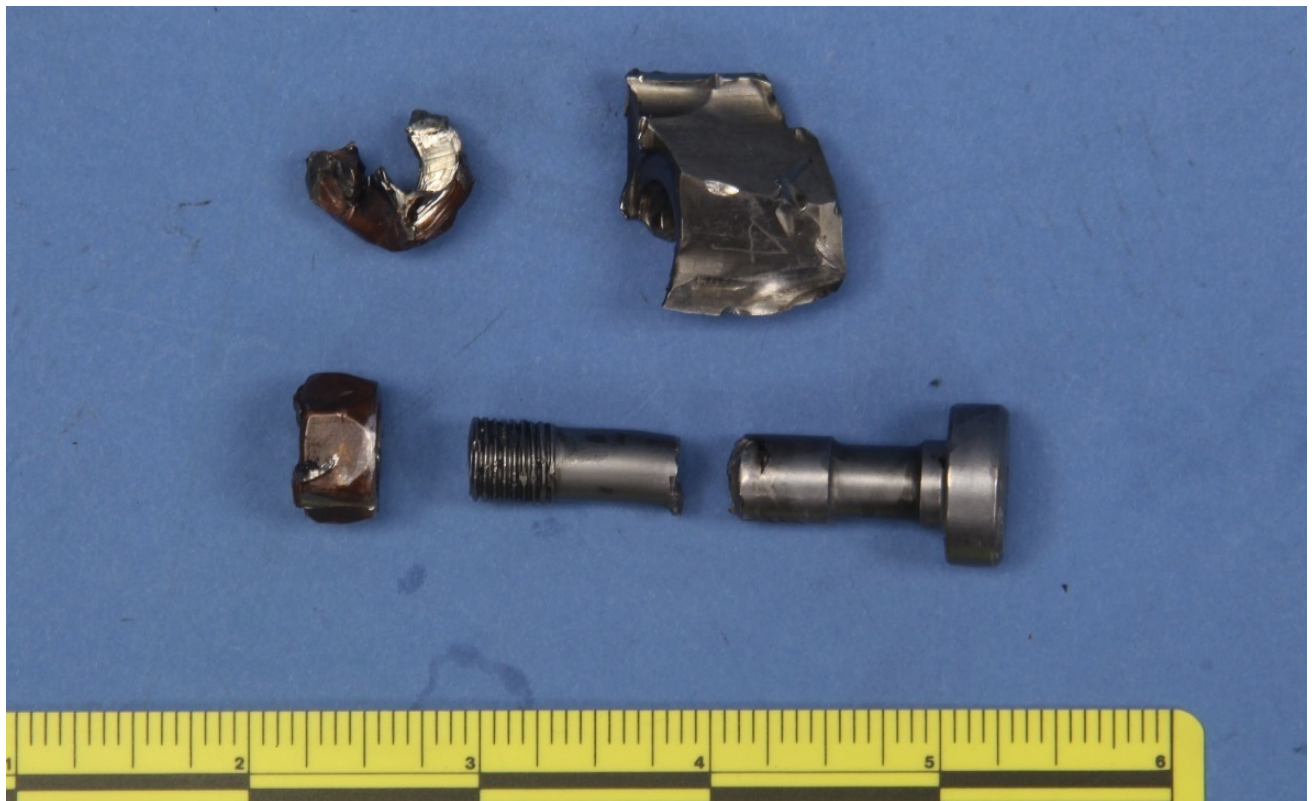
Figure 12 – Remnants of the #4 connecting rod cap, with remnants of an attachment bolt and two nuts.
