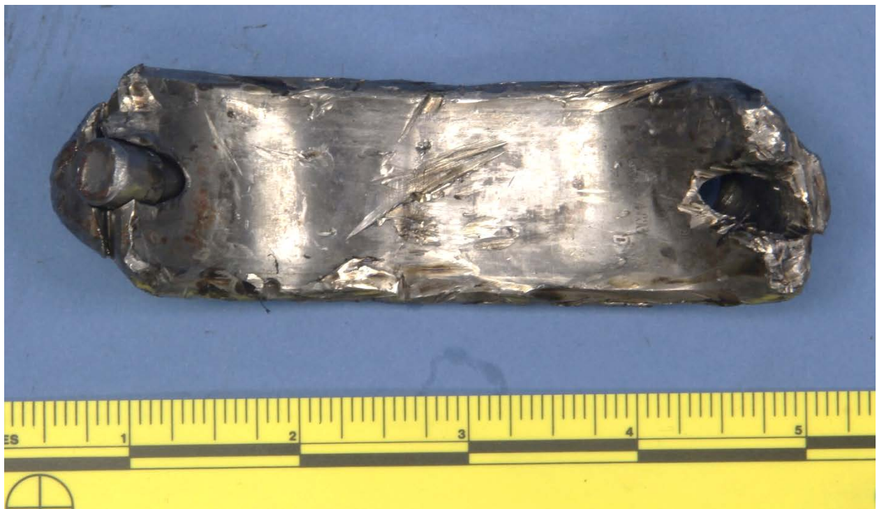
Figure 8 – View of the loose and intact #6 connecting rod cap remnant from the inside surface.
