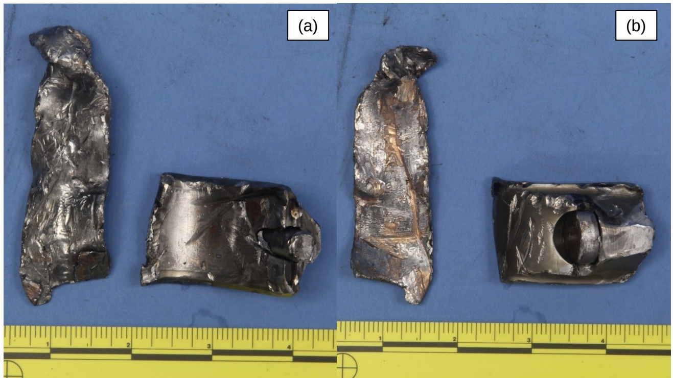
Figure 11 – Remnants of the #4 bearing and a cap fragment viewed from (a) the inner and (b) outer surfaces.
