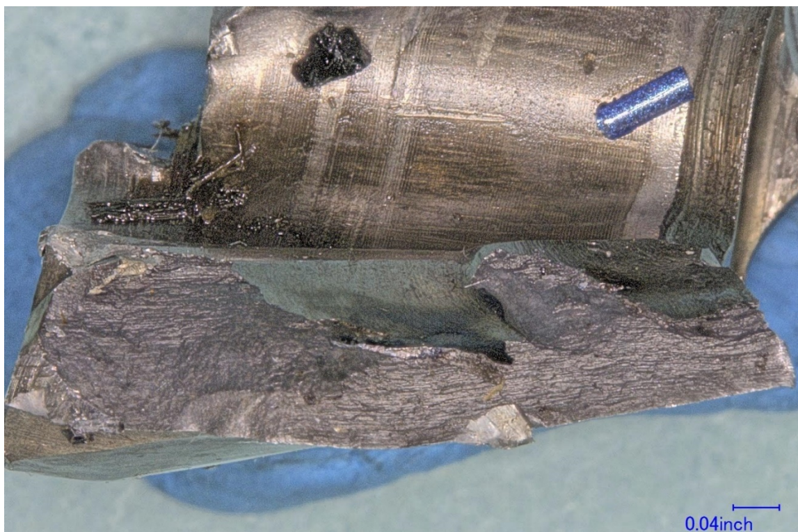
Figure 13 – View of the undamaged area of the fracture surface from the remnant in Figure 12.
