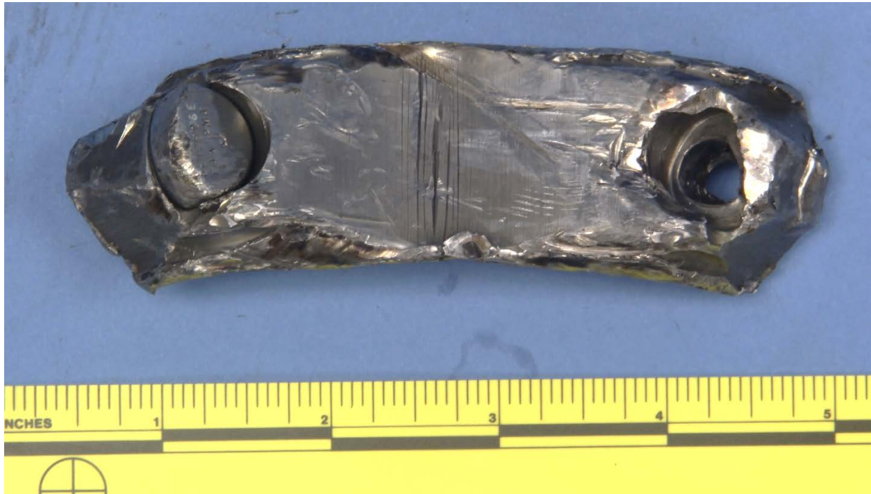
Figure 9 – View of the loose and intact #6 connecting rod cap remnant from the outside surface. There was a bolt remnant in the cap remnant.
