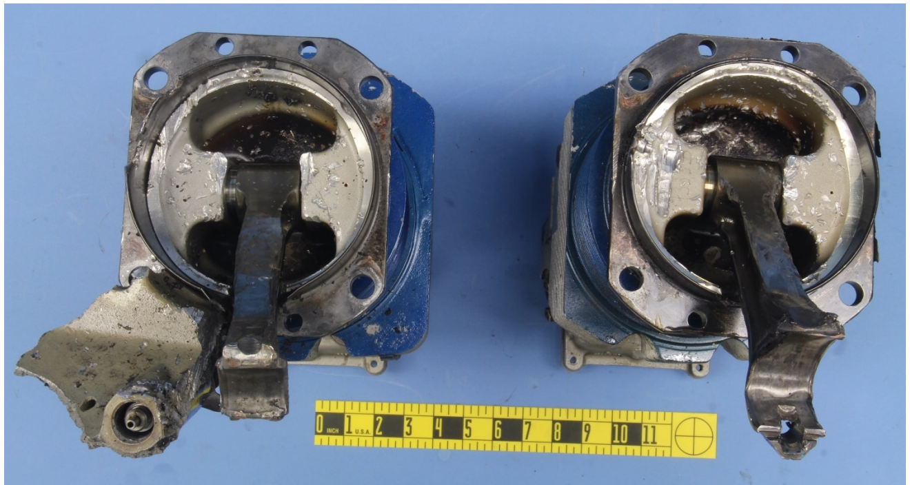
Figure 5 – View of the connecting rod sides of the cylinder assembly remnants from the #4 and #6 cylinders.
