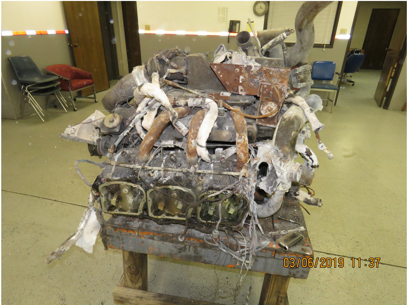
Photo 3 – Engine from accident airplane
