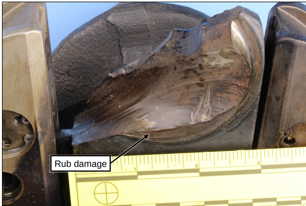
Figure 3. Overall view of the forward side of the fracture after the crankshaft was cut through the number 3 main journal and before the fracture surface was cleaned.
