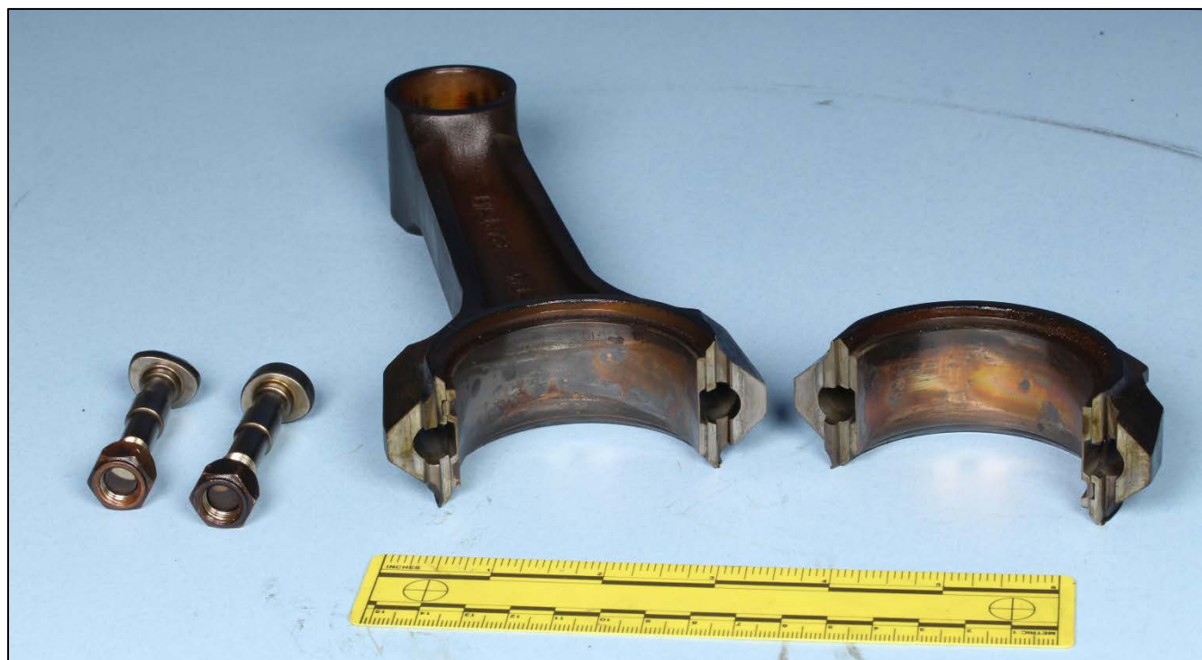
Figure 2. Number 6 connecting rod assembly after disassembly from the crankshaft.
