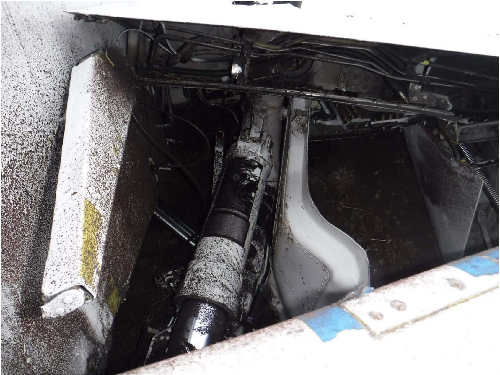
Photo 4 – Collapsed Right Main Landing Gear, Photo courtesy of Lone Star Retrieval
