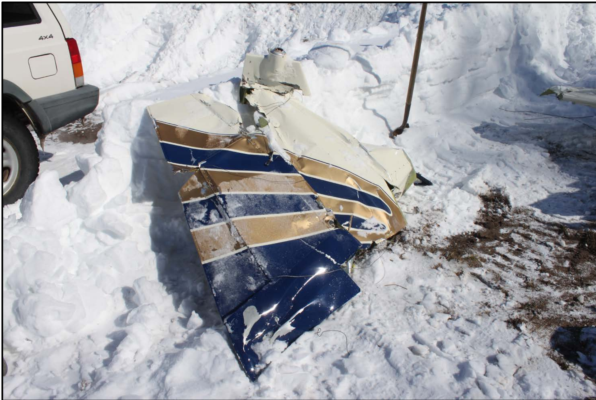
Photo 13 – Vertical Stabilizer (NTSB Photo)
