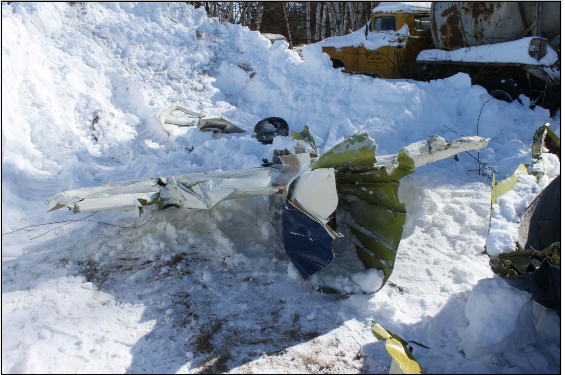
Photo 14 – Aft Fuselage / Horizontal Stabilizers (NTSB Photo)
