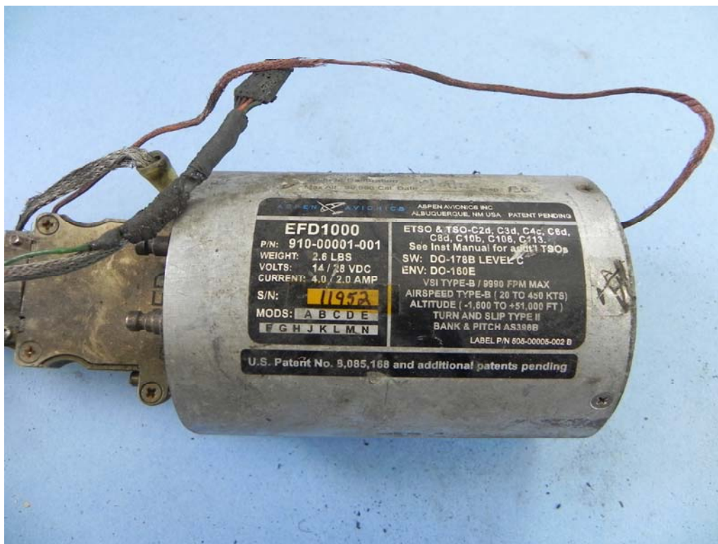
Figure 1. Photo of damaged EFD1000 Pro
