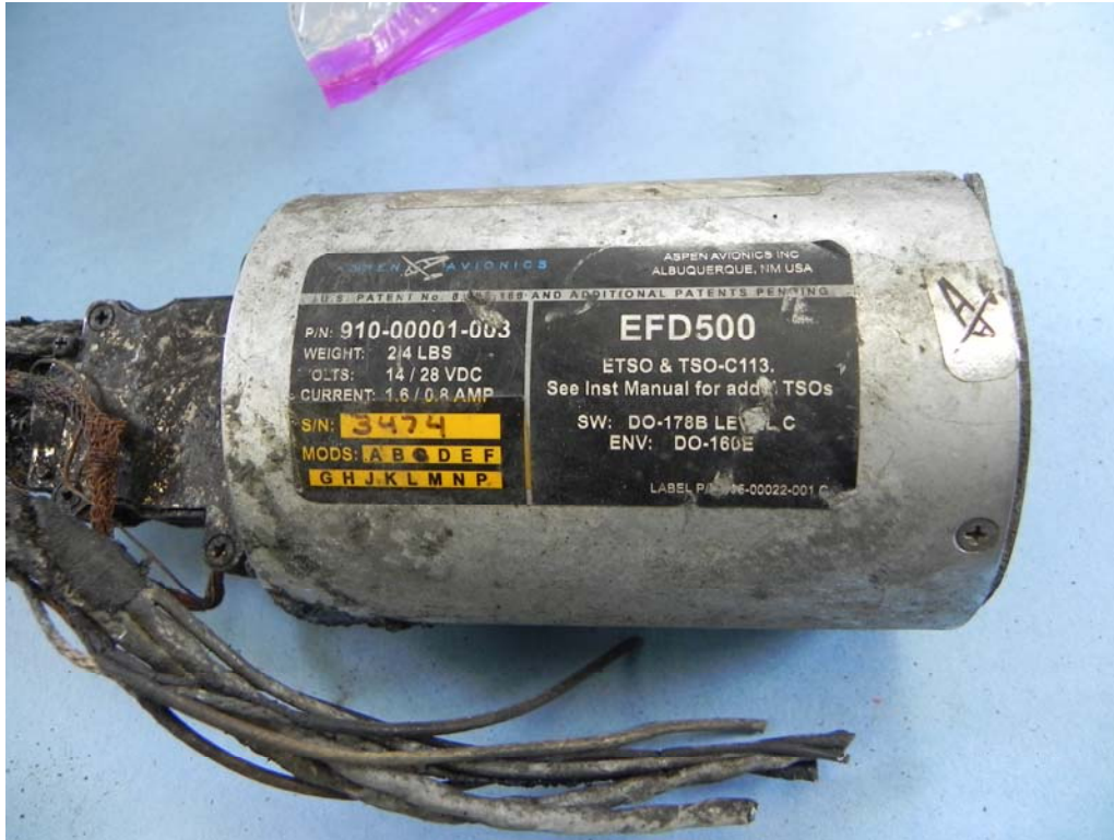
Figure 2. Photo of damaged EFD500
