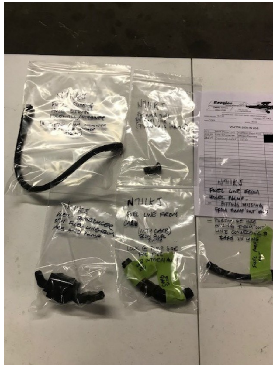
Photo 3 – Fuel Line Components collected from Accident Airplane (Courtesy of NTSB)
