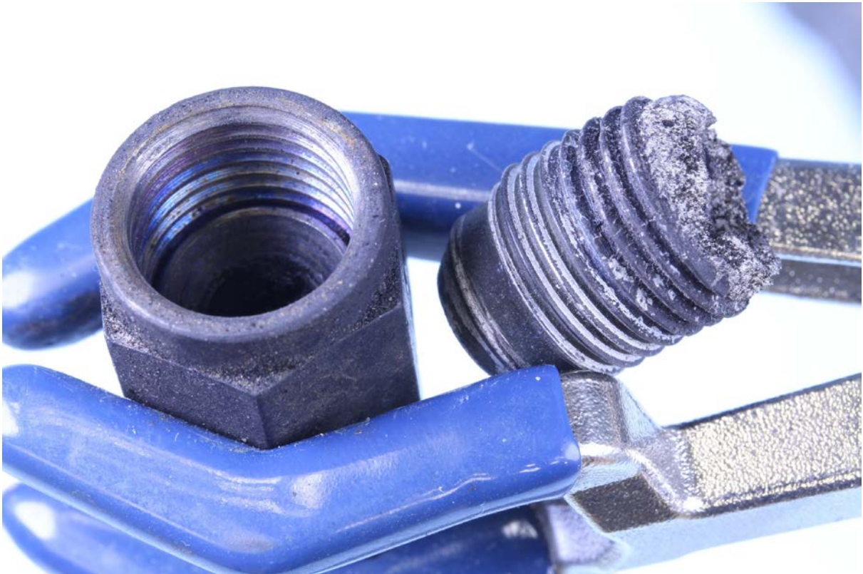
Figure 3: Fitting from component #3 with oxides from high temperature exposure.
