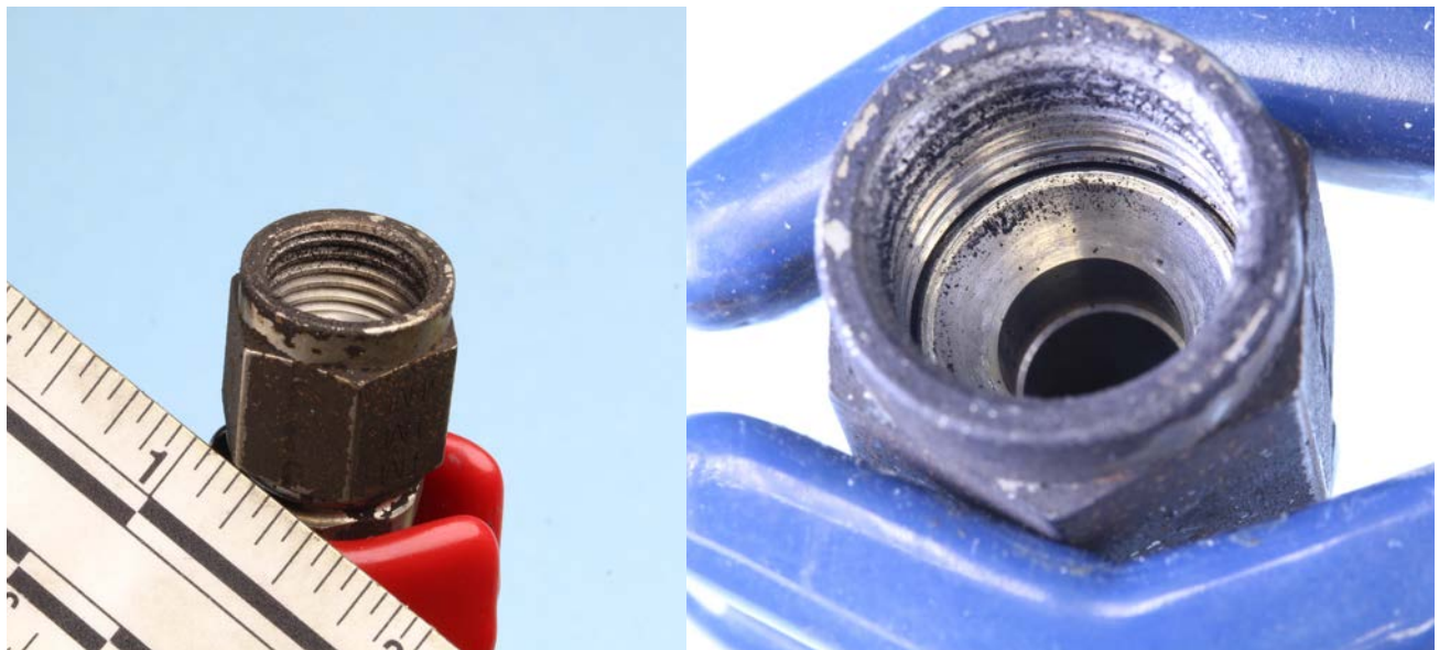
Figure 4: Fitting from component #3 with soot deposits inside. Two views of the same fitting.
