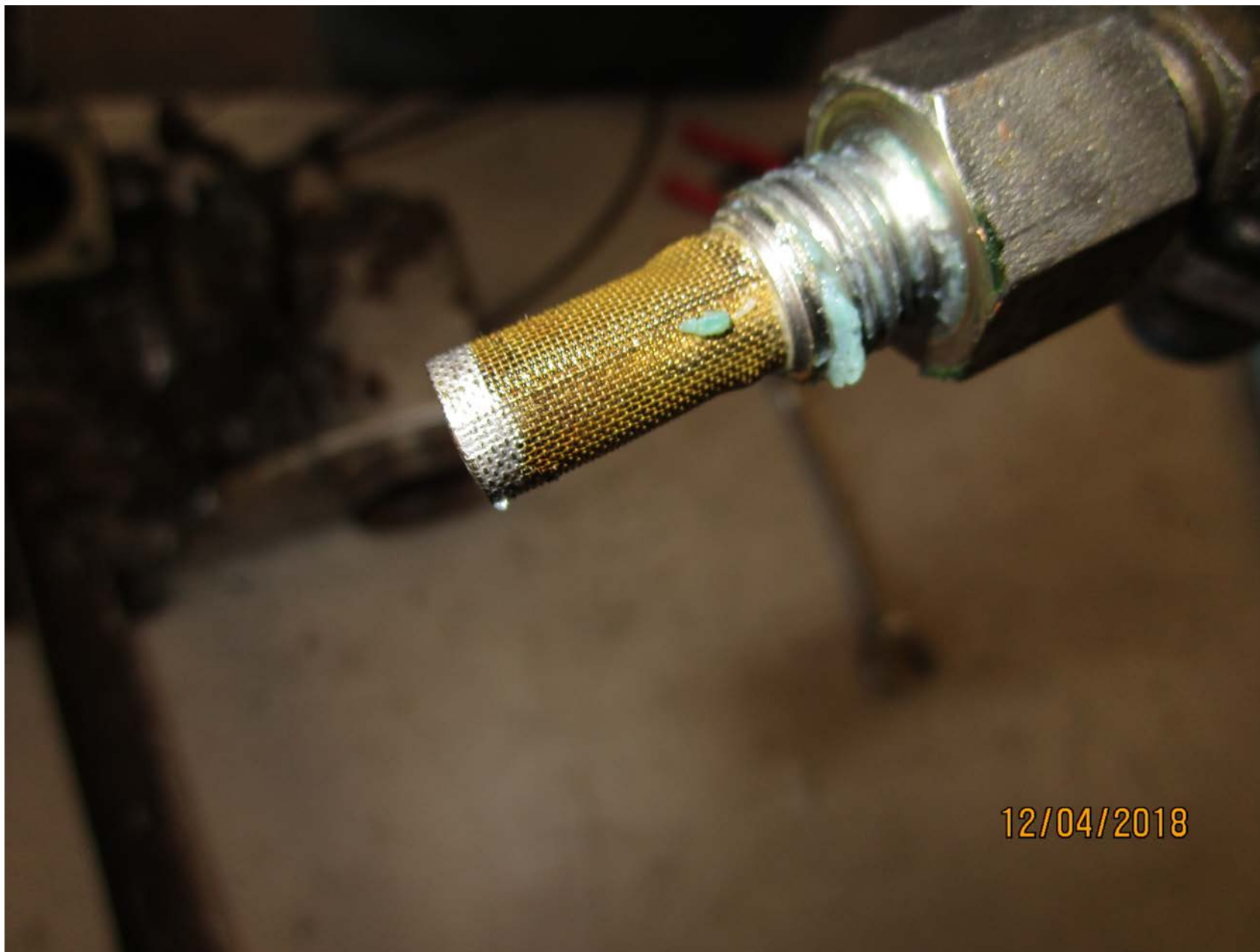
Photo 8 - View of the removed fuel filter from the carburetor.
