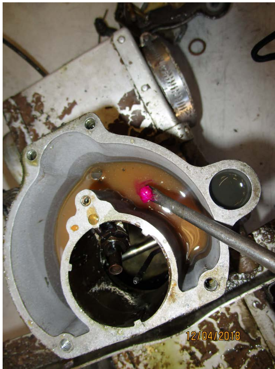
Photo 9 - View of the carburetor fuel bowl containing a liquid and water testing paste with a positive indication.
