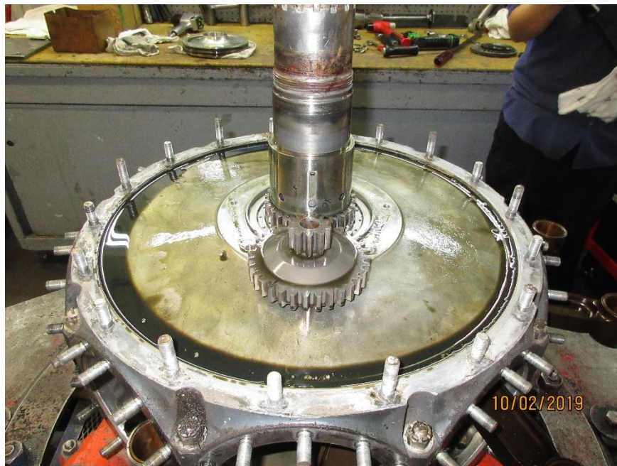
Power Section with Cylinders and Nose Case removed Photo # 8
