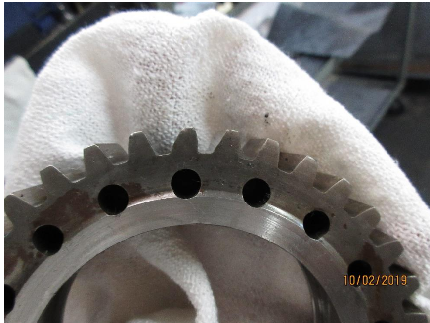
8797 Floating Gear (*Note damage to teeth) Photo #14
