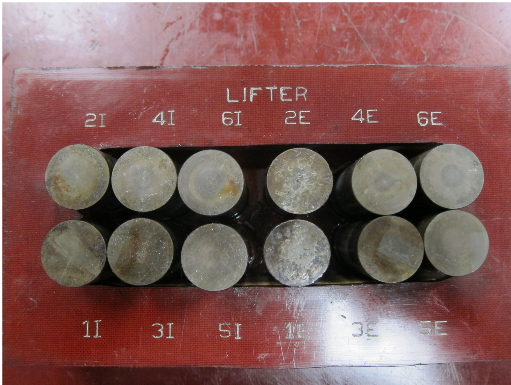
Photo 5 – Engine Lifters (CMI Photo)
