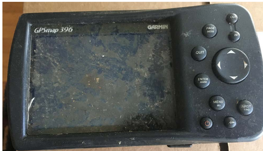
Figure 1 – Front of device with damage to the screen
