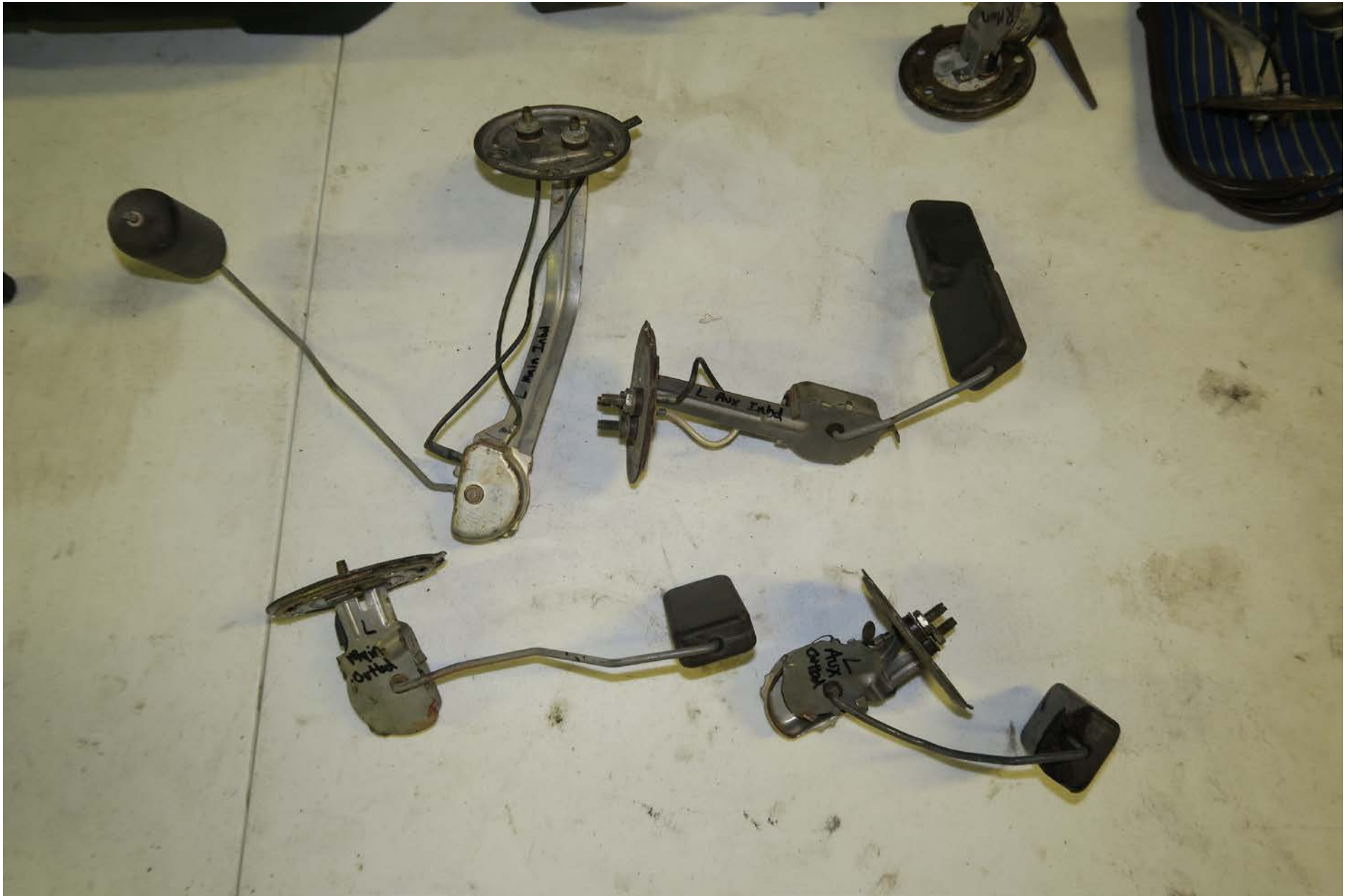
Photo 9 – All left wing fuel transmitters
