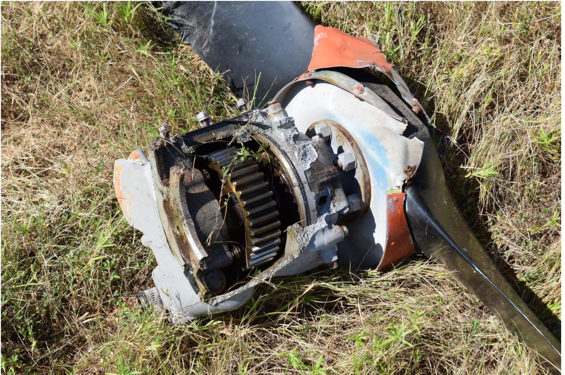
Photo 3 – Reduction Gearbox and Propeller, Photo from FAA
