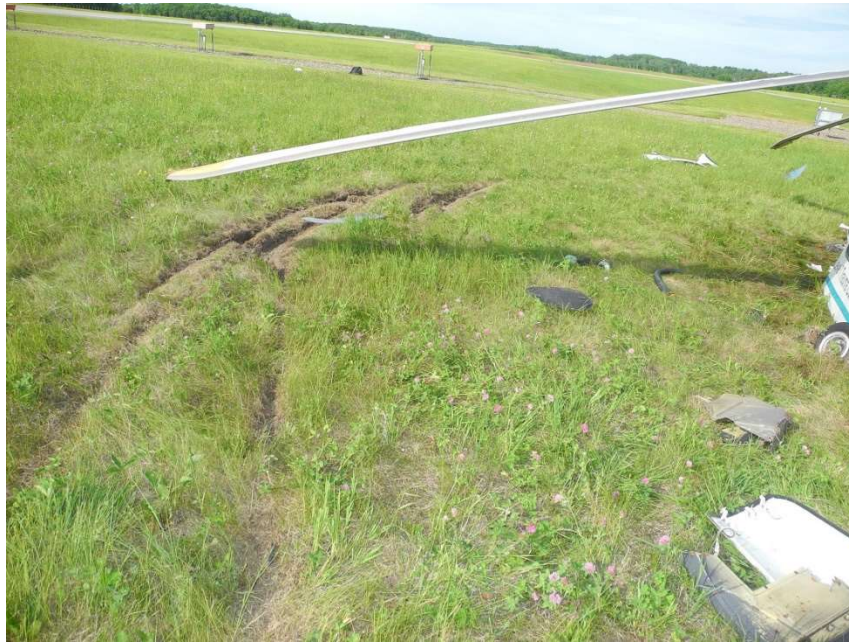
Figure 3. Ground scars to the left of the accident helicopter.
