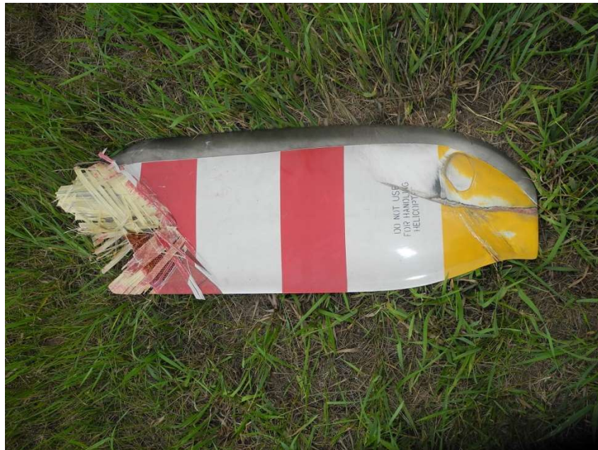
Figure 5. The separated tail rotor blade, found about 211 feet from the main wreckage.
