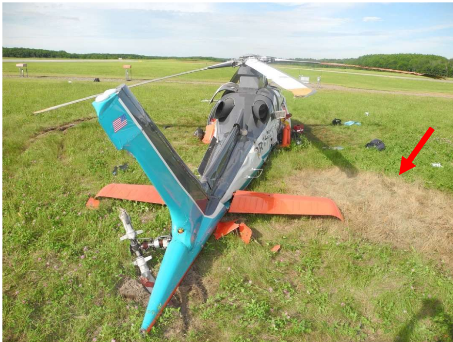
Figure 8. A red arrow points to discoloration observed on the grass to the aft-right of the No. 2 engine exhaust.
