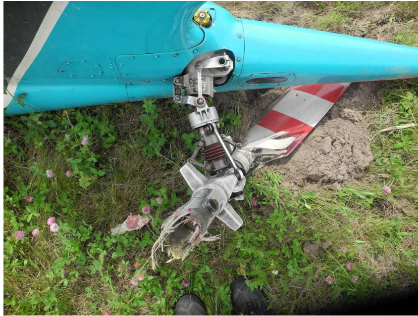
Figure 4. The tail rotor attached to the tail gearbox.
