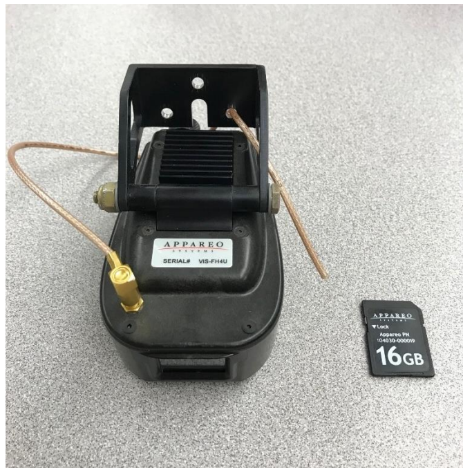
Figure 1. The Appareo Vision 1000 device and the associated SD card, as received.
