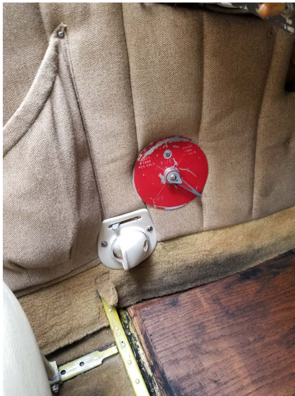
Photo 6 – Fuel selector position as found at accident site
