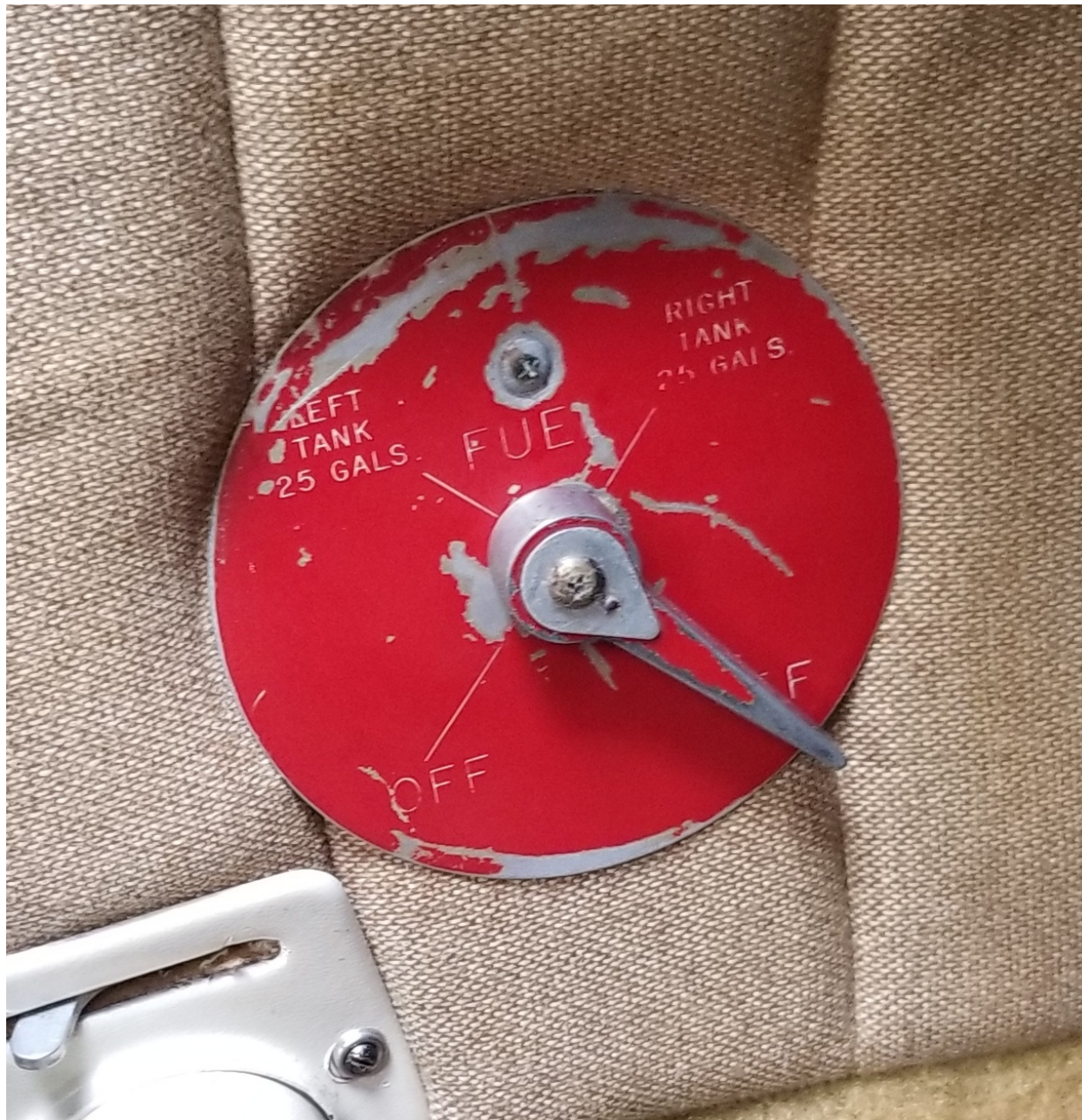
Photo 9 – Enlarged photo of fuel selector in accident airplane
