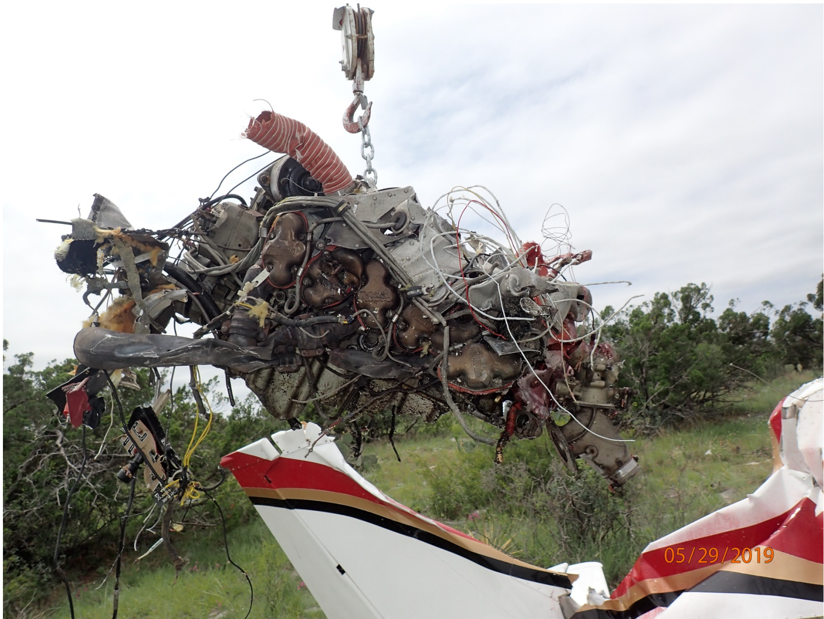
Photo 3 – Airplane Engine After Removal from Embedded Terrain and Airplane Structure
