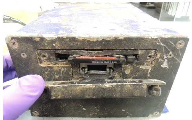
Figure 3. CF card mounted in SATLOC M3.
